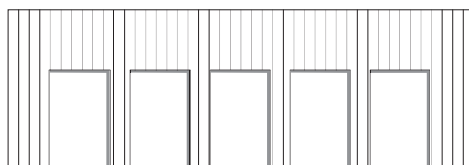
Test 2: When separate the row of windows with columns the window width now become 3 meters. The room is even though still exposed to overheating hours.
