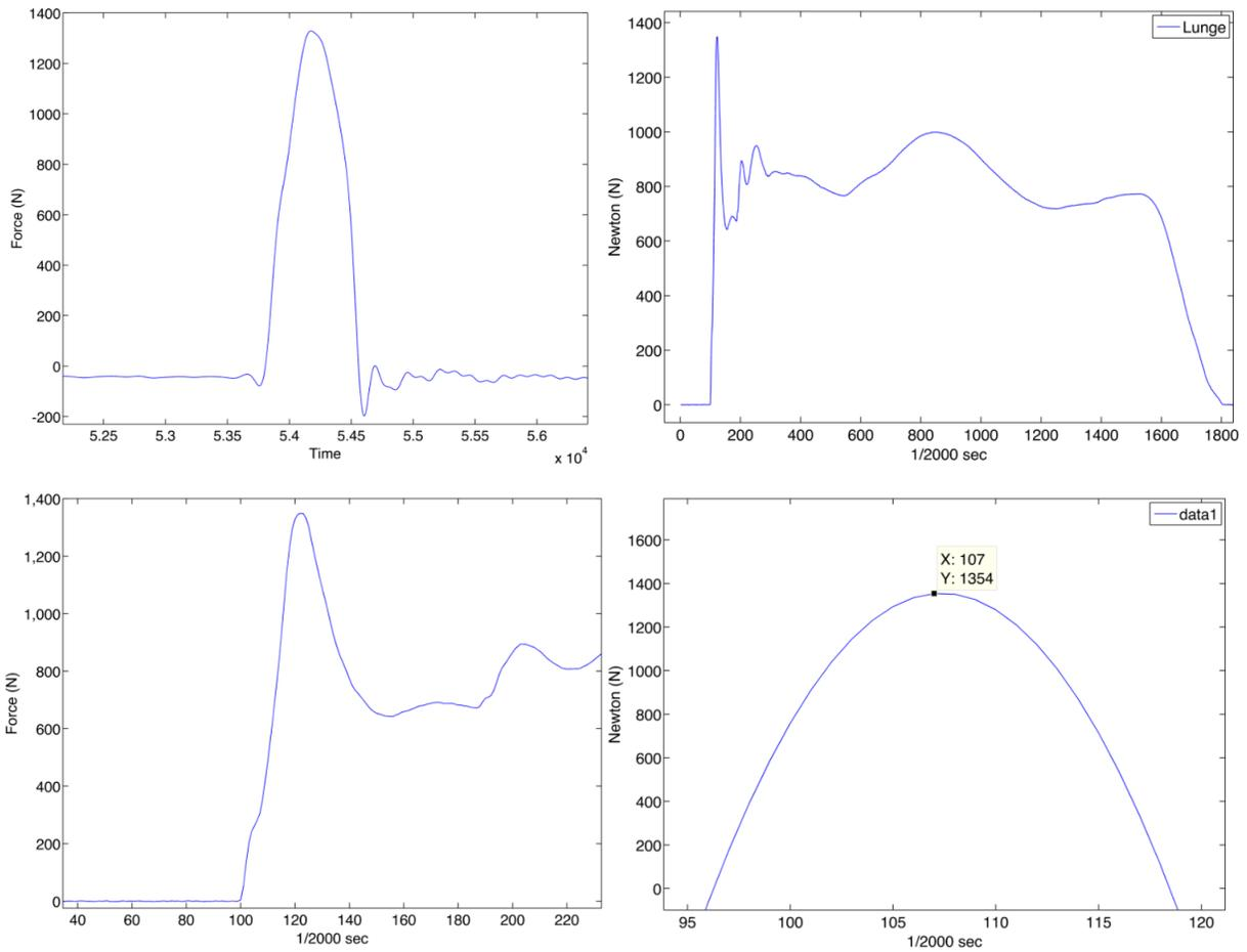
**Figure 1:** Top left (1a): Impact with AID. Top right (1b): Badminton lunge impact performed by a player. Bottom left (1c): Heel strike part of the badminton lunge force-time curve. Bottom right (1d): Quadratic fit of the impact peak from the badminton lunge.
