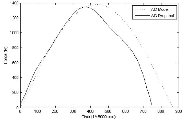
**Figure 6:** Force-time curves of the AID-model (theoretical) and mean of 15 AID-drop tests for the badminton lunge configuration.
