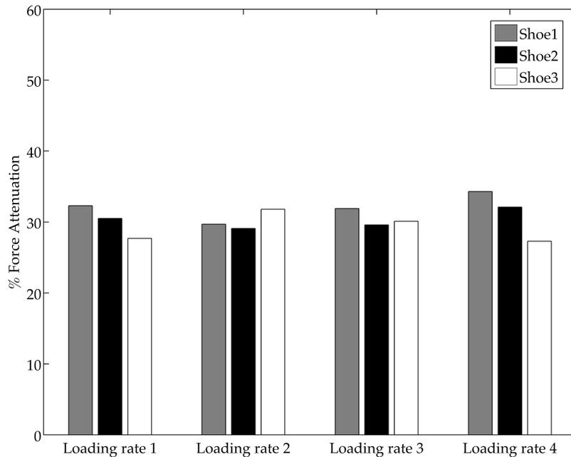
**Figure 8:** Mean percentagewise force attenuation of Shoe1, Shoe2 and Shoe3 from the loading rate test.
