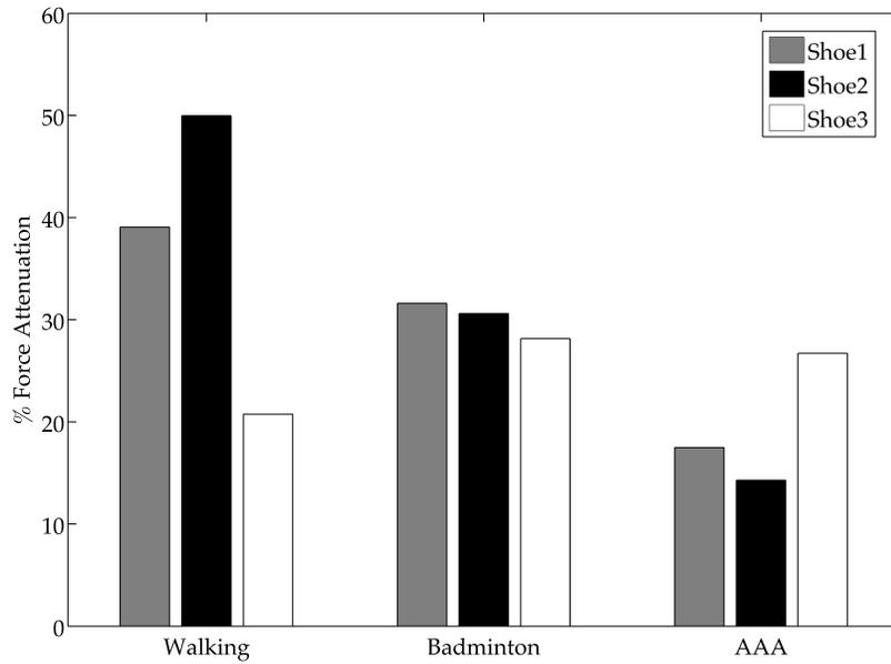
**Figure 7:** Mean percentagewise force attenuation of Shoe1, Shoe2 and Shoe3 from the force attenuation test.
