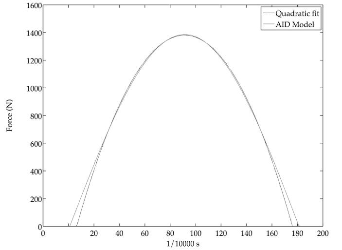
**Figure 3:** A comparison between the AID-model and the quadratic fit made from the badminton lunge. The configuration illustrated is the badminton configuration found in table 2.
