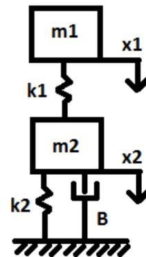
**Figure 2:** A free body diagram of the AID-model.  $m_1$  and  $m_2$  are the masses of the missile and floor/shoe, respectively.  $x_1$  and  $x_2$  are the displacements of the missile and floor/shoe, respectively.  $k_1$  and  $k_2$  are the spring constants of the missile and floor/shoe, respectively.  $B$  is the dampening coefficient.
