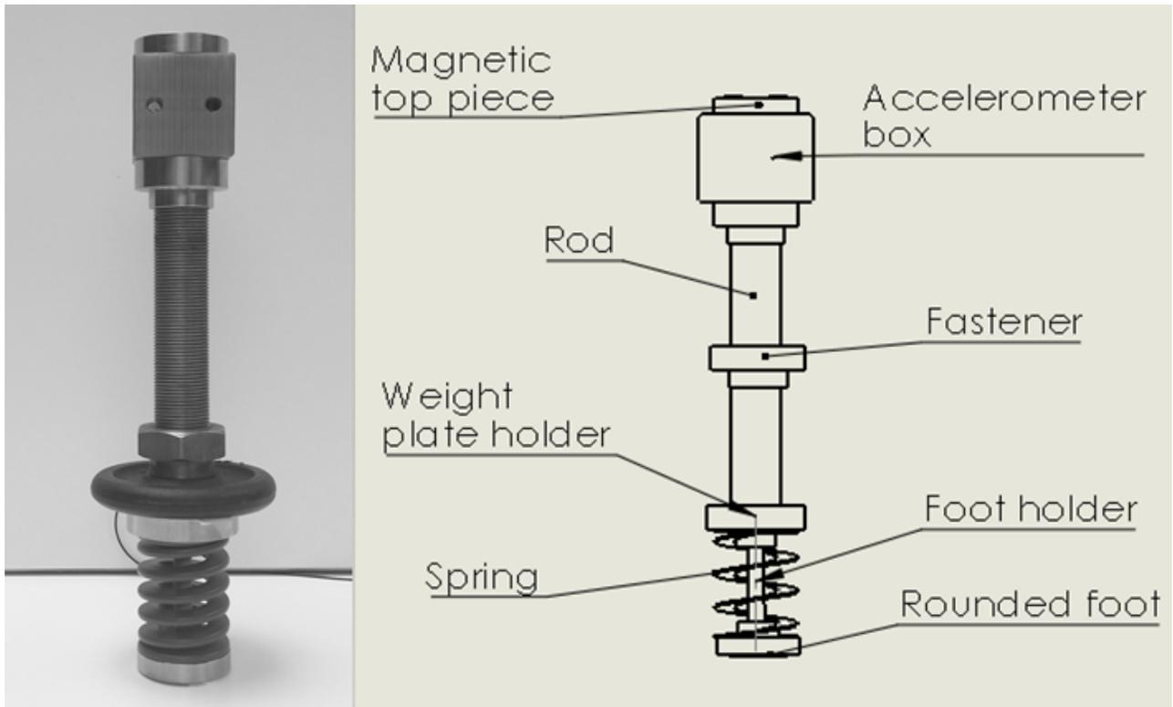
**Figure 5:** Left: The missile of the AID. Right: Labelled technical overview of the AID. The overview is without added weight plate(s).
