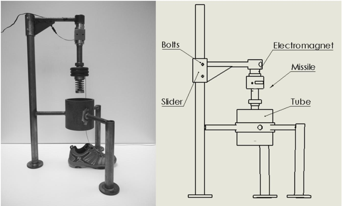
**Figure 4:** The test setup. The missile is held by an electromagnet. Acceleration is recorded upon release of the missile. After impact, the missile is contained by the surrounding tube.
