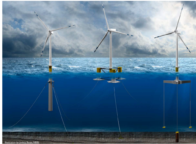
Figure 1.2: Spar buoy (left, with catenary mooring lines), Semi-submersible (middle, with catenary mooring lines) and TLP. [52]
