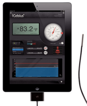
Ill. 2 iCelsius PRO probe connected by wire to ipad (iCelsius Pro Sort, No date)
