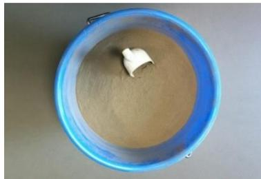
Figure 35 - Low-calcium (ASTM class F) dry fly ash
