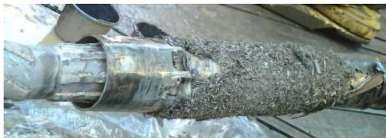
Figure 9 - Metal debris (swarf) [11]
