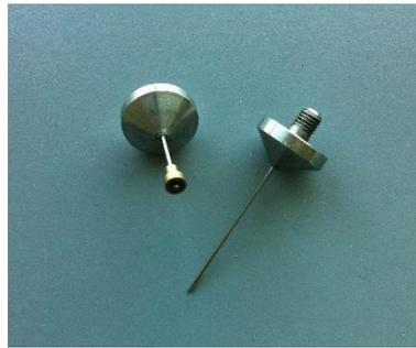
Figure 33 - Different needles used in Vicat test
