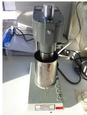
Figure 25 - Cylindrical viscometer FANN S35SA
