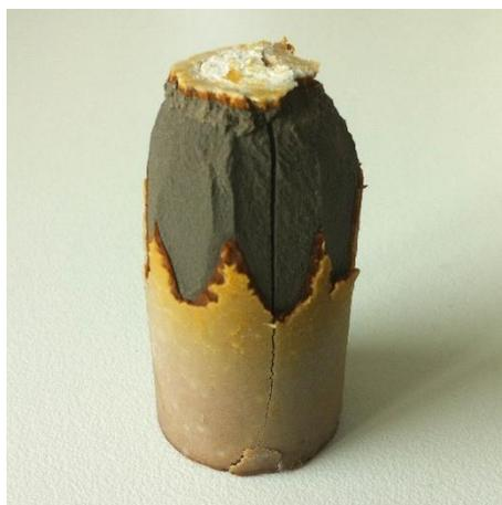
Figure 71 - Residual amorphous silicate zone
