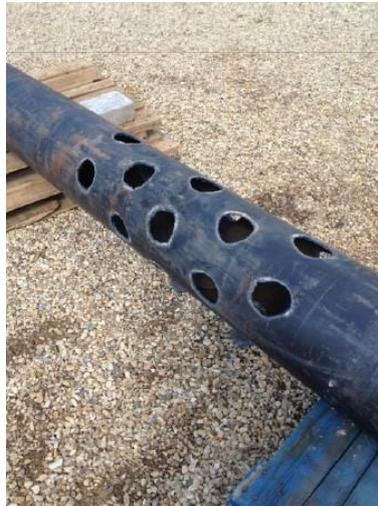
Figure 7 - Perforated tubing [11]
