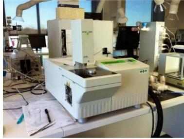
Figure 30 - Mettler Toledo DSC822e
