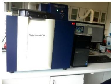
Figure 27 - X-ray fluorescence (XRF) spectrometer
