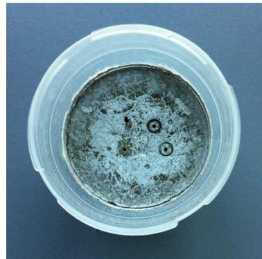
Figure 34 – Initial and final setting time tests
