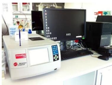
Figure 29 - DelsaMax Pro light scattering analyser
