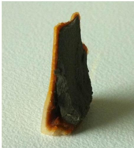
Figure 70 - Tight layer of sludge on the surface of OPC
