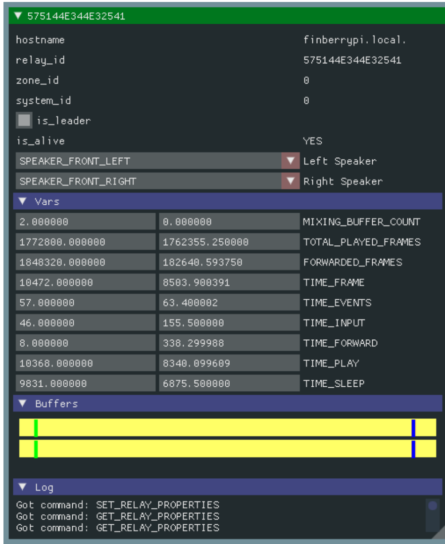
Figure 8: Debug interface. Shows major configuration properties of a relay. Allows the manipulation of these basic properties. Shows performance and debugging statistics. Shows mixing handles (green playback, blue write, red forward). Here red is not visible as the entire buffer was forwarded. Shows a subset of the logs produced by the relay.
