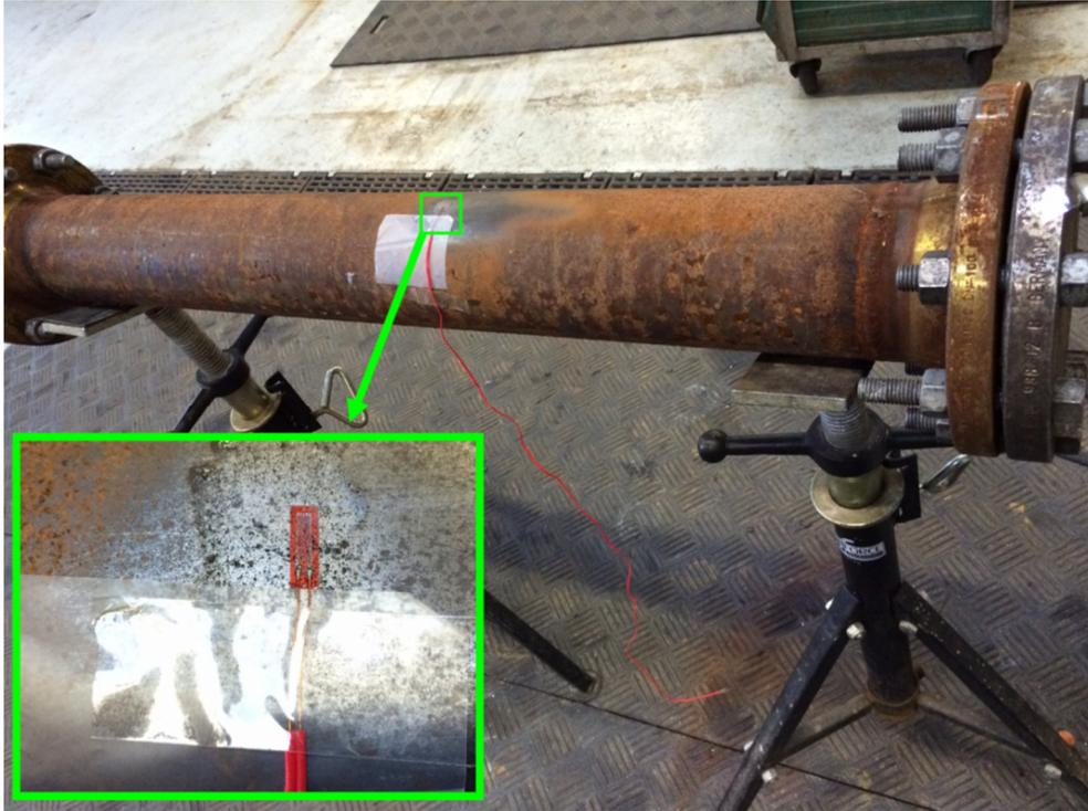
**Figure 3-7: Test-1, Strain gauge for measuring circumferential strain**
