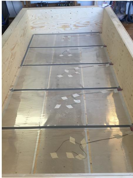
**Figure 4.3.** Placement of the electrical heating mats into the backwall of vertical channel.
