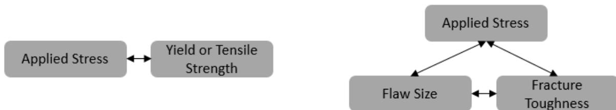
Figure 4: (R) Relation of Classical failure theory, (L) Relation of Fracture mechanics
