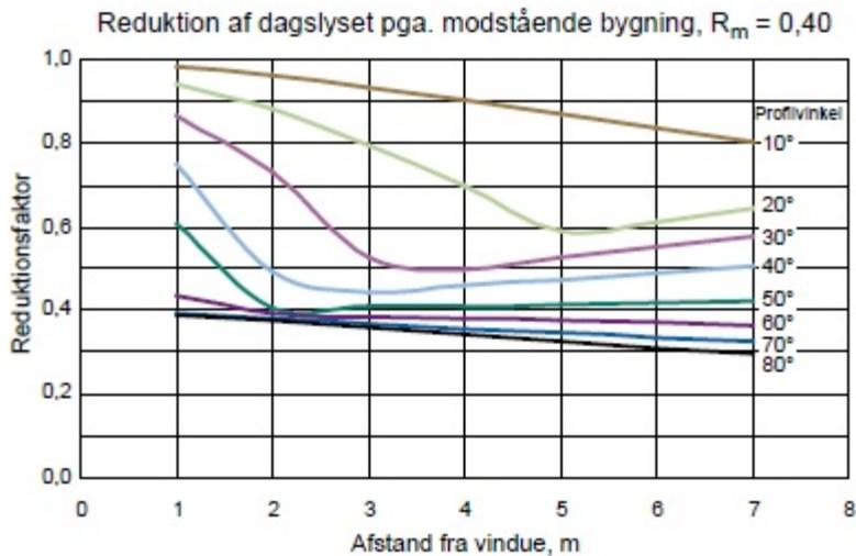
Figure O.9. Reduction factor for an opposing building with an average reflectance of  $R_m = 0.40$
