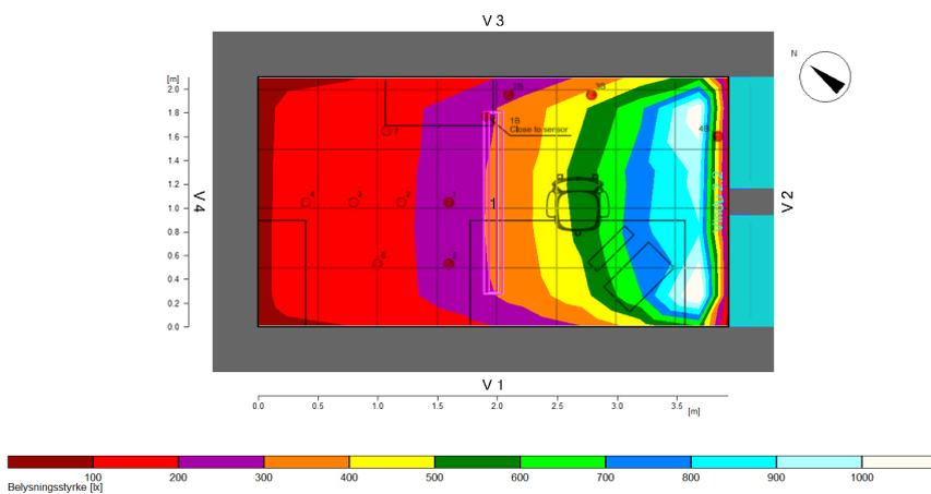
**Figure 4.12.** The ray tracing calculation method in Relux for CIE overcast sky showing illuminance distribution in the cell office with external obstruction
