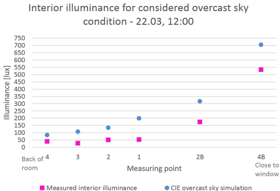
Figure 5.13. The interior illuminance for believed overcast sky condition the 22<sup>nd</sup> of March compared with simulated interior illuminance for overcast CIE sky condition at 12:00.
