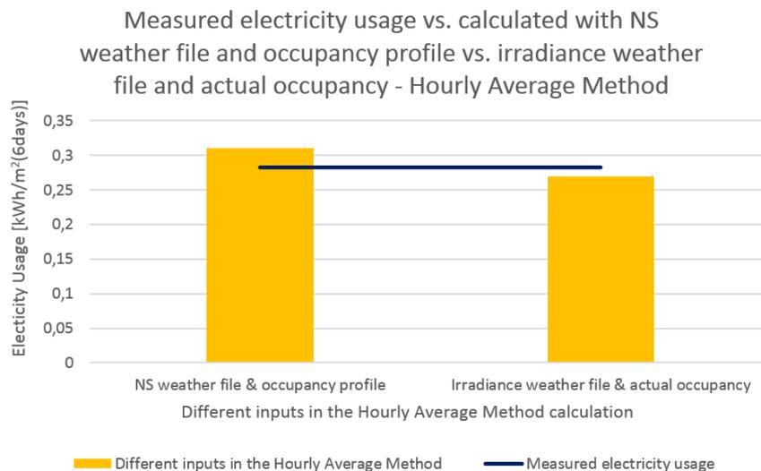
**Figure 16.4.** The calculated electricity usage with NS weather file and occupancy profile as an input in the *Hourly Average Method*, and the irradiance weather file and actual occupancy as an input, compared to the measured electricity usage.
