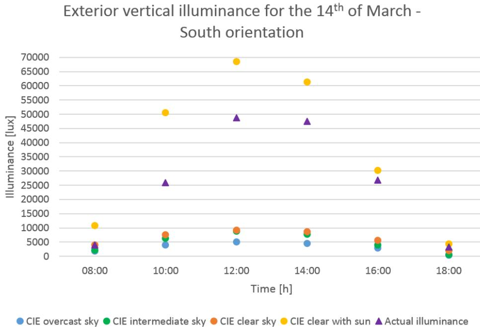
**Figure 5.20.** The exterior illuminance on a vertical reference plane on the south façade at 12:00 for 14<sup>th</sup> of March comparing measured sky to simulated overcast, intermediate, clear and clear with sun CIE sky conditions.
