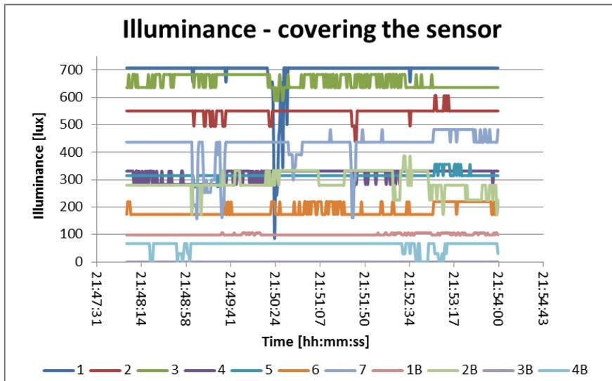
**Figure G.5.** Illuminance measured by the luxmeters in the room when the daylight sensor is covered
