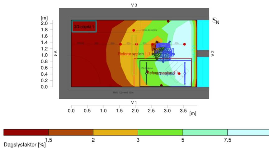
**Figure C.7.** Daylight factor from Relux obtained with the raytracing method for the cell office with furniture
