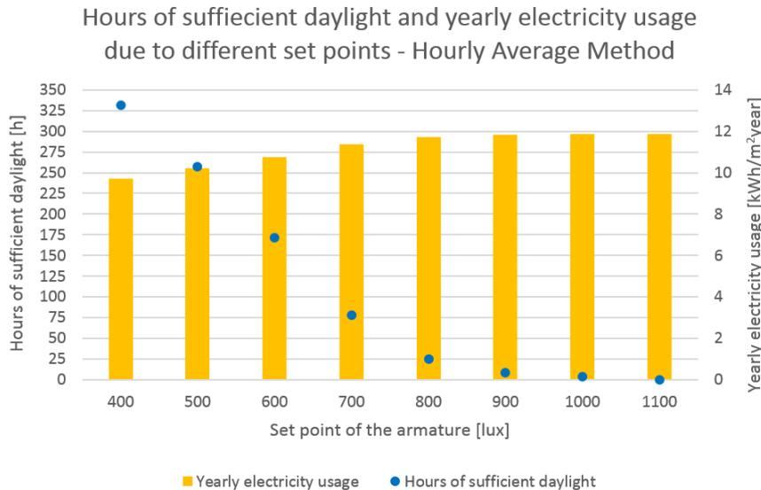
**Figure 16.5.** Hours of sufficient daylight and corresponding yearly electricity usage due to different set points for the armature calculated with the *Hourly Average Method*
