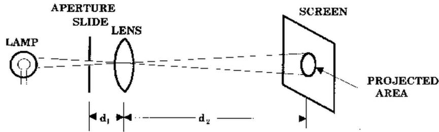
*Figure 3.4.* Luminous intensity per unit area projected in a specific direction depends on the projected area (Halsted, February 2015).
