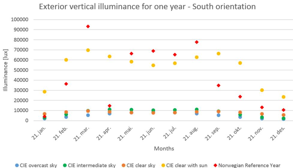
**Figure 5.26.** The exterior illuminance on a vertical reference plane on the south façade at 12:00 for the 21<sup>st</sup> of every month of a year comparing the Norwegian reference year to simulated overcast, intermediate, clear and clear with sun CIE sky conditions.
