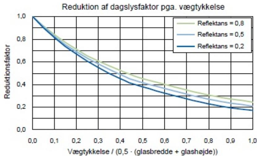
Figure O.5. Reduction factor for wall thickness
