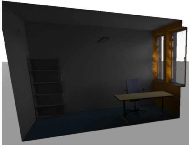
**Figure C.8.** 3D illustration of the luminance from Relux obtained with the raytracing method for the cell office with furniture
