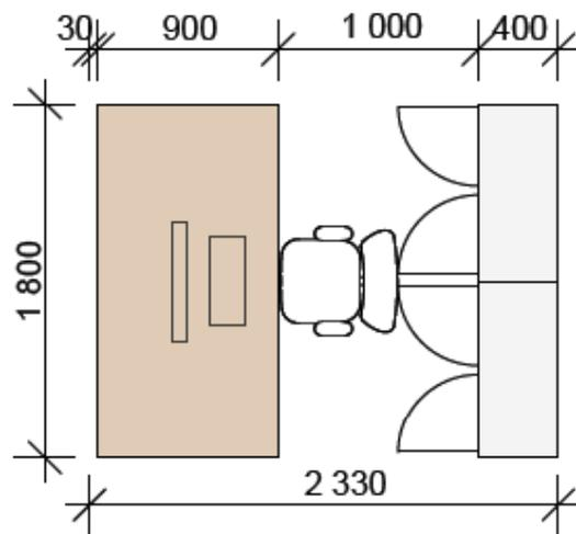
**Figure A.19.** A typical workspace module with measurements
