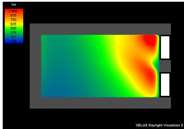
*Figure 4.9.* Photon mapping in VELUX Daylight Visualizer CIE clear sky showing illuminance distribution in the cell office
