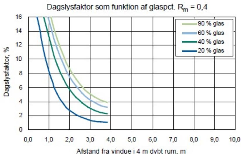
Figure O.1. Daylight factors for a 4 m deep room with different window areas
