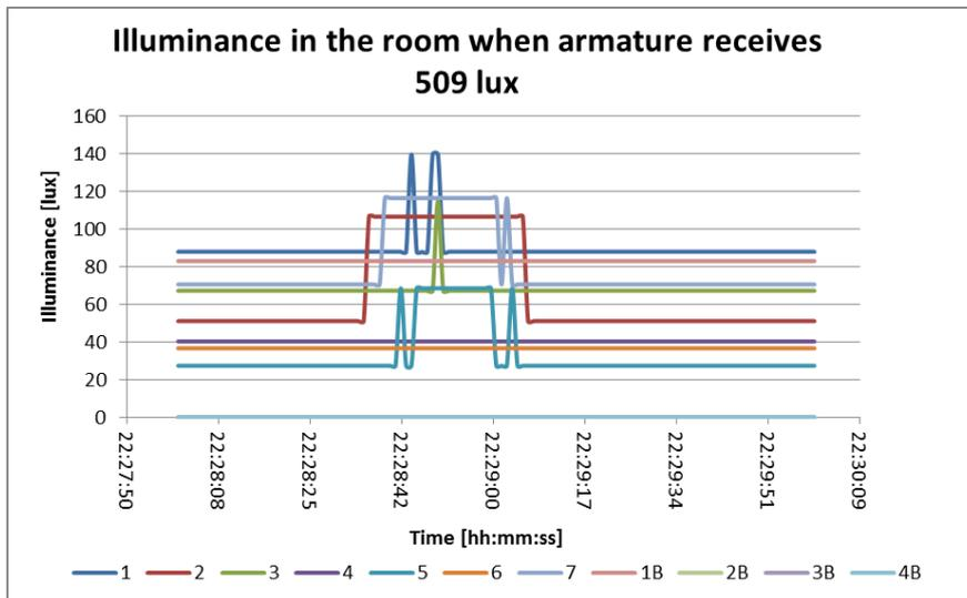
**Figure G.6.** Illuminance measured by the luxmeters in the room when the daylight sensor receives 509 lux
