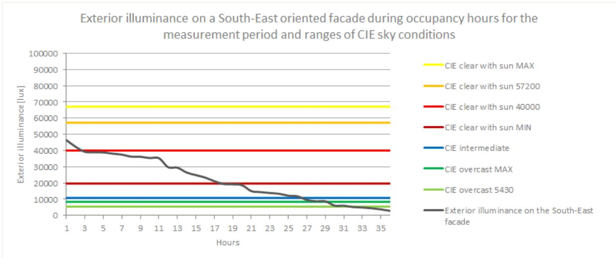
**Figure 15.6.** TotVEI from measurement period using irradiance weather data file for exact occupancy
