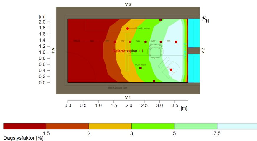
**Figure C.2.** Daylight factor from Relux obtained with the radiosity method for the cell office without furniture
