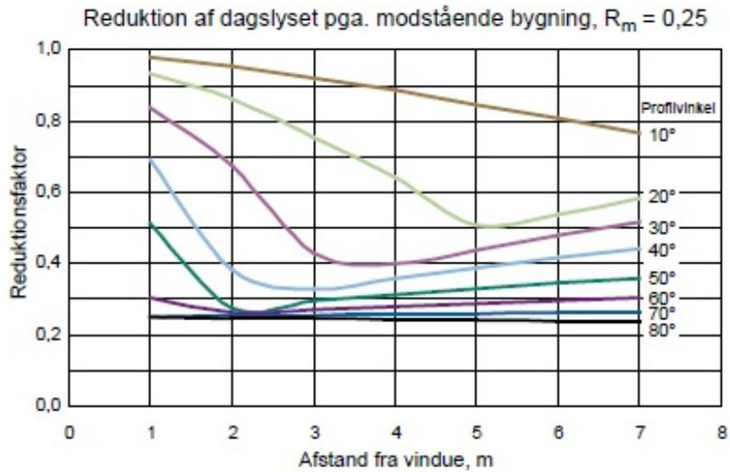
Figure O.8. Reduction factor for an opposing building with an average reflectance of  $R_m = 0.25$
