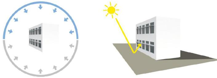
**Figure 5.21.** Mirrored sky concept for ground plane reflection for the ray tracing method in Relux (RELUX Informatik AG, 2011).
