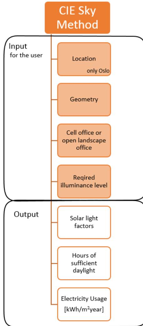
*Figure 15.1.* Illustration of the flow of inputs and output in the *CIE sky method*
