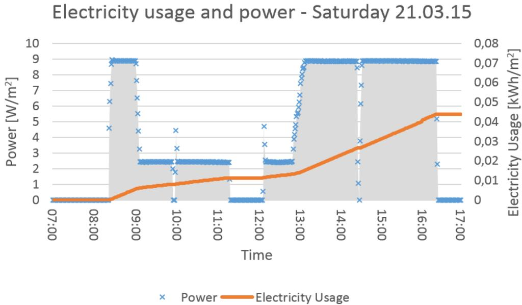
**Figure 6.3.** The power and electricity usage of the armature in the cell office during Saturday the 21<sup>st</sup>.
