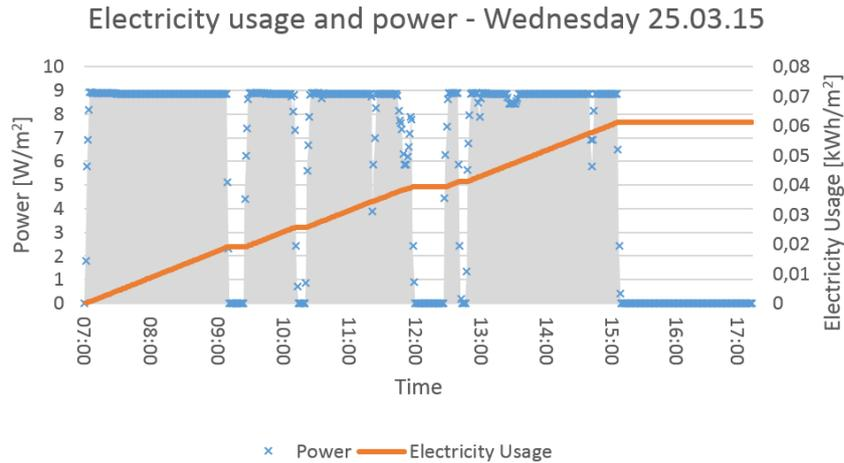
**Figure I.47.** The effect and electricity usage of the armature during Wednesday 25.03.15
