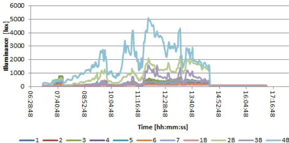
Figure L.4. Interior illuminance when the shading was activated from 14 : 30
