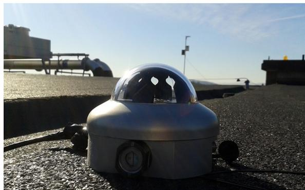
*Figure D.2.* The pyranometer
