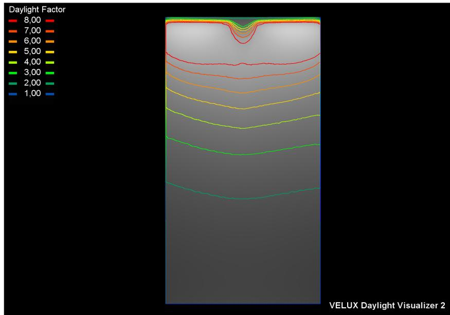
*Figure C.12.* Daylight factor for a single cell office
