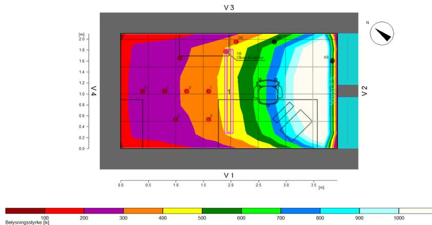
*Figure 4.2.* The radiosity calculation method in Relux for CIE overcast sky showing illuminance distribution in the cell office without external obstruction
