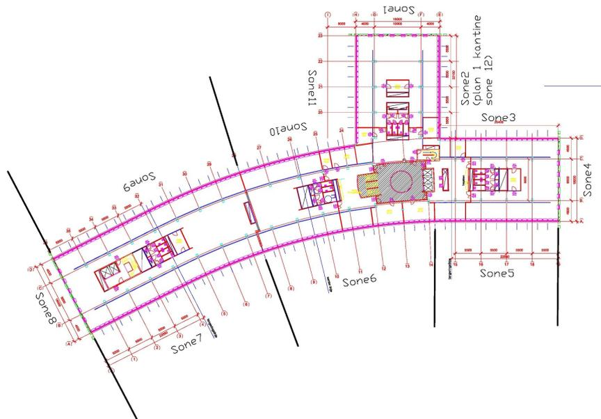
**Figure A.29.** The twelve zones for the control system of the solar shading
