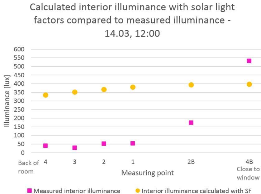
**Figure 14.9.** Calculated interior illuminance with solar light factors for the cell office in the case building compared to measured illuminance at 12:00 on March the 14<sup>th</sup>
