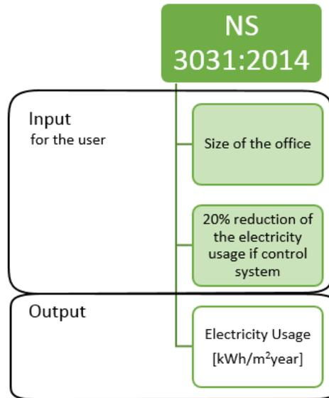
*Figure 13.2.* Illustration of the flow of inputs and output in the method from *NS 3031:2014*.
