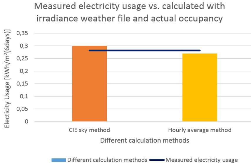
**Figure 17.3.** The calculated electricity usage by *CIE Sky Method* and *Hourly Average Method* with irradiance weather file and actual occupancy, compared to the measured electricity usage
