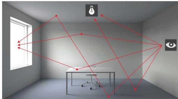
**Figure 4.4.** The backward ray tracing calculation method (Statens Byggeforskningsinstitut, 2013)
