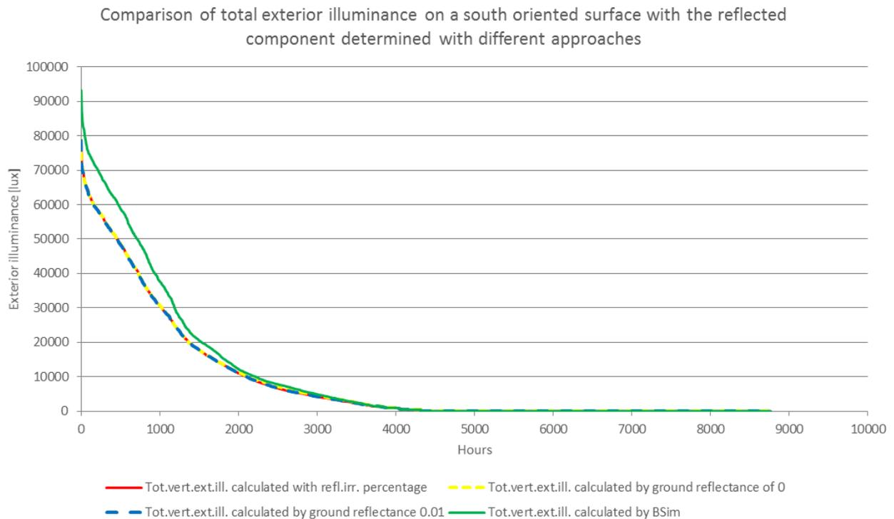
**Figure 14.10.** Extracting RefVEI from the percentage of the irradiance components and from the deviation between DiffVEI and DirVEI with and without ground reflectance
