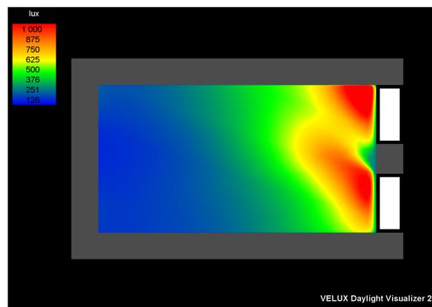
**Figure 4.16.** Photon mapping in VELUX Daylight Visualizer for CIE clear sky showing illuminance distribution in the cell office with external obstruction
