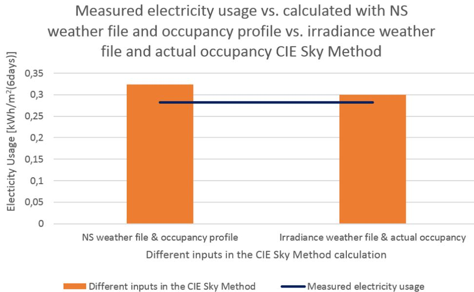
**Figure 15.8.** Comparison of the calculated electricity usage with the NS weather file and occupancy profile as an input in the *CIE sky method*, and the irradiance weather file and actual occupancy as an input to the measured electricity usage
