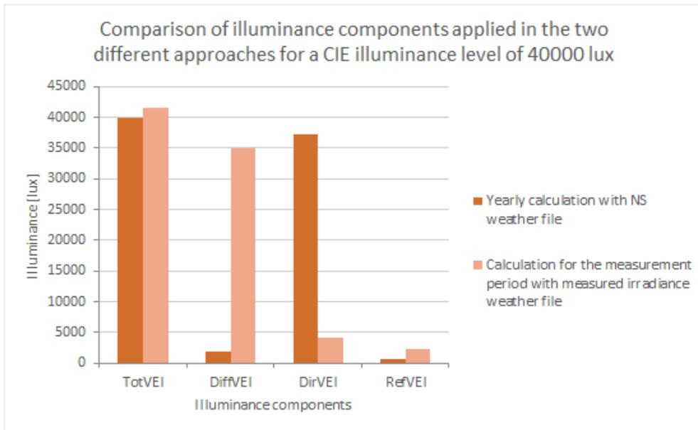
**Figure 15.9.** Comparison of the illuminance components applied in the different cases for a CIE illuminance level of 40000 lux
