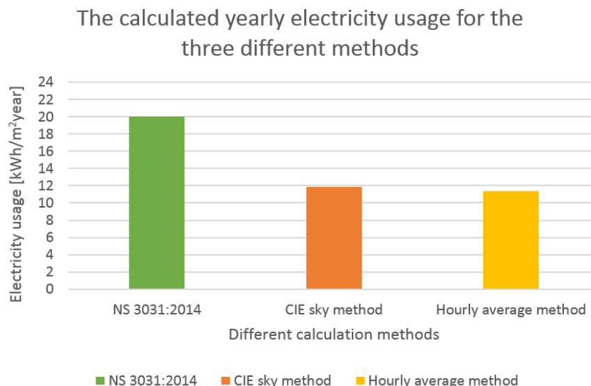
*Figure 17.1.* The calculated yearly electricity usage from the three different
