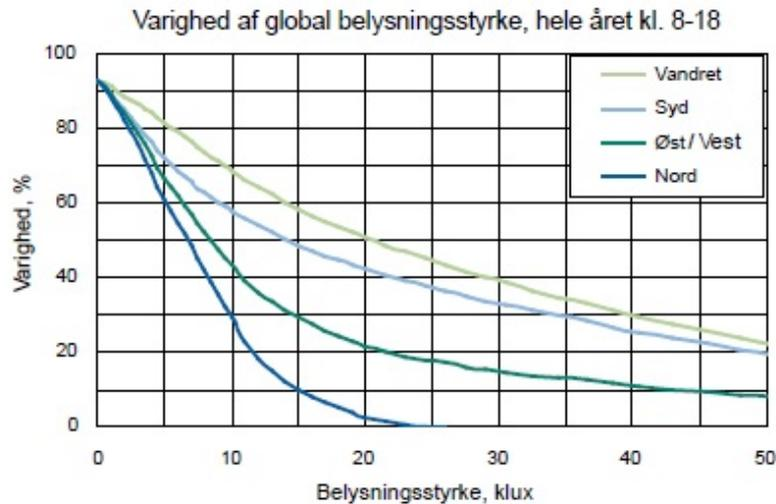
Figure O.19. The duration of the illuminance on a horizontal and four vertical planes
