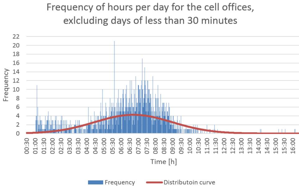
**Figure 8.6.** Frequency histogram and normal distribution of hours per day for cell offices, excluding the days shorter than 30 minutes
