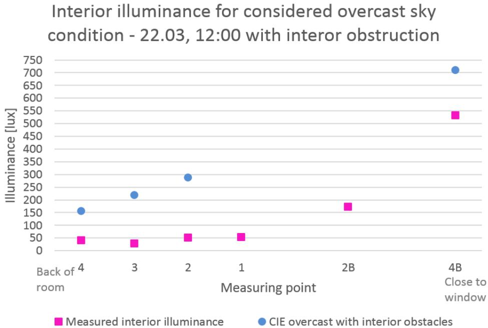
**Figure 5.15.** The interior illuminance for believed overcast sky condition the 22<sup>nd</sup> of March compared with simulated interior illuminance with internal obstructions for overcast CIE sky condition at 12:00.
