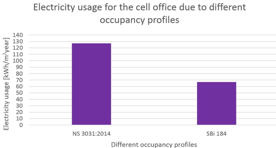
Figure 7.1. Yearly electricity usage for the cell office due to different occupancy profiles from NS3031:2014 and SBi 184
