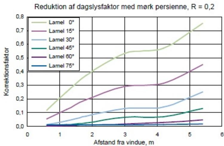
Figure O.15. Correction factor for a dark blinds positioned in different angles
