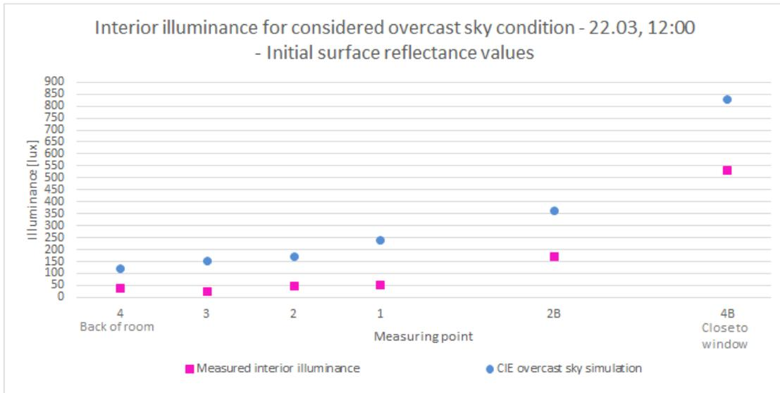
**Figure 3.11.** Measured interior illuminance compared to simulated interior illuminance when the first set of reflectance values are applied
