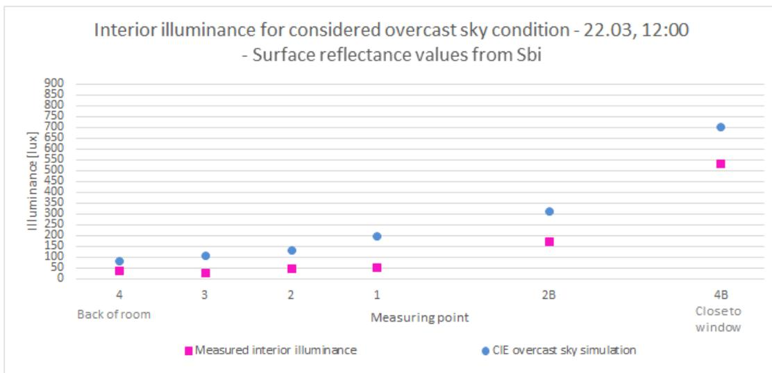
**Figure 3.12.** Measured interior illuminance compared to simulated interior illuminance with surface reflectance values extracted from *SBi*
