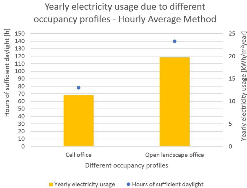
**Figure 16.6.** Hours of sufficient daylight and corresponding yearly electricity usage of the armature calculated with the Hourly Average Method with different occupancy profiles
