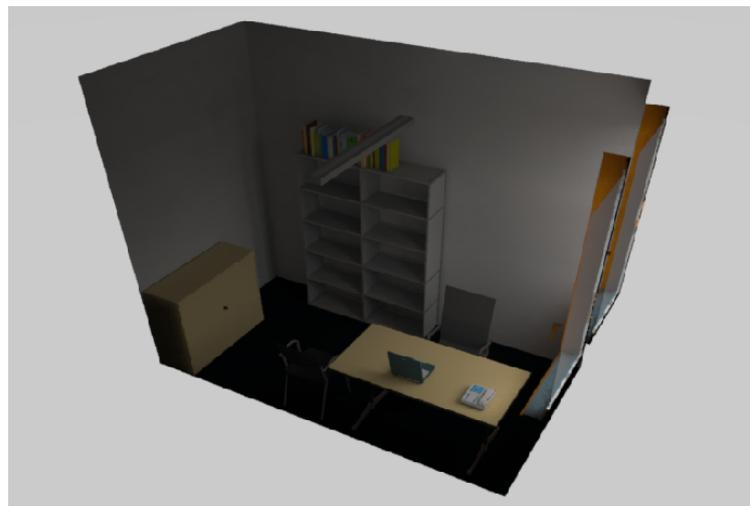
**Figure 5.14.** Illustrative picture of the scene in Relux for the interior luminance obtained with ray tracing for CIE overcast sky condition the 22<sup>nd</sup> of March at 12:00.
