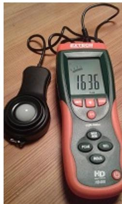
*Figure F.1.* Hand-held illuminance meter used for the reflectance measurements
