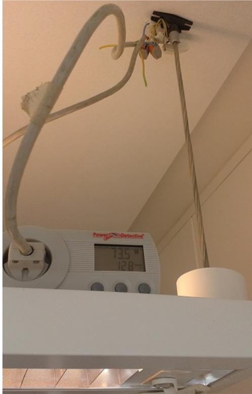
*Figure H.5.* The placement and attachment of the SparOmeter on the armature
