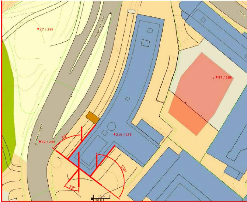
*Figure A.12.* The orientation of the façades measured with AutoCAD on the map obtained from Kartverket
