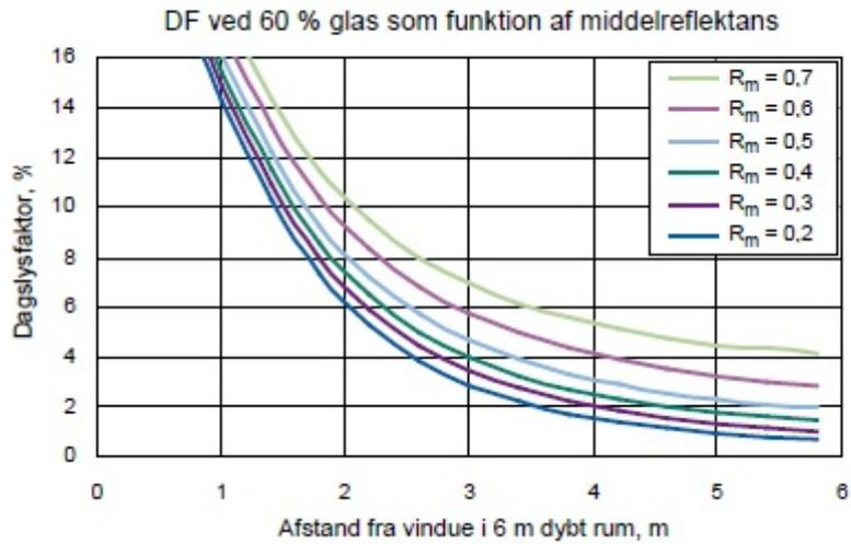
*Figure O.11.* The variation in the daylight factor as a function of the mean reflectance
