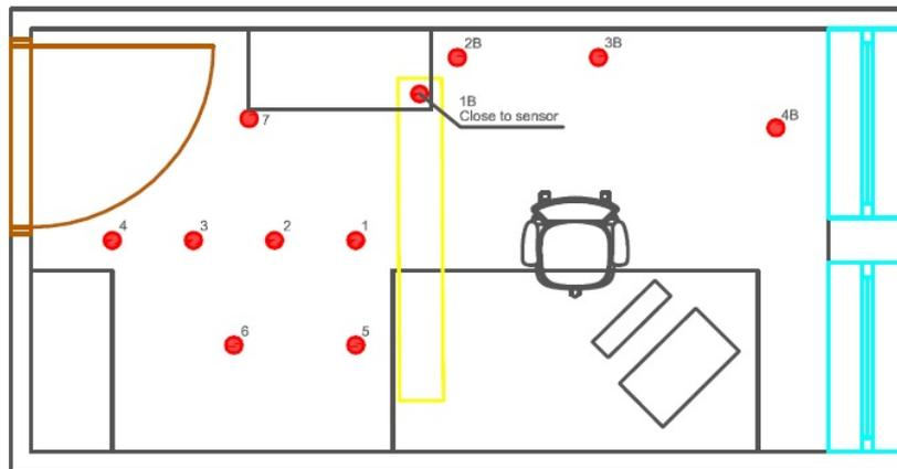
*Figure 5.12.* The placement of the illuminance meters in the cell office.
