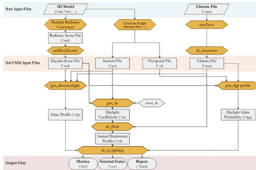
**Figure B.2.** Chart showing input, output and subprograms used in DAYSIM (Daysim, December 2014b).
