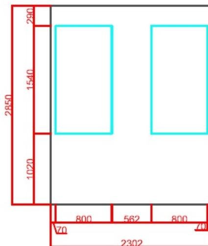
**Figure 2.12.** Façade of the cell office with dimensions
