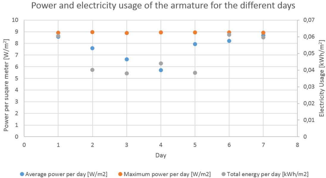
**Figure 6.1.** The effect, power and hours of use of the armature for the different days.
