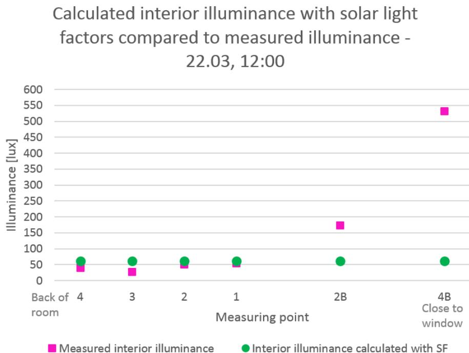
**Figure 14.8.** Calculated interior illuminance with solar light factors for the cell office in the case building compared to measured illuminance at 12:00 on March the 22<sup>nd</sup>
