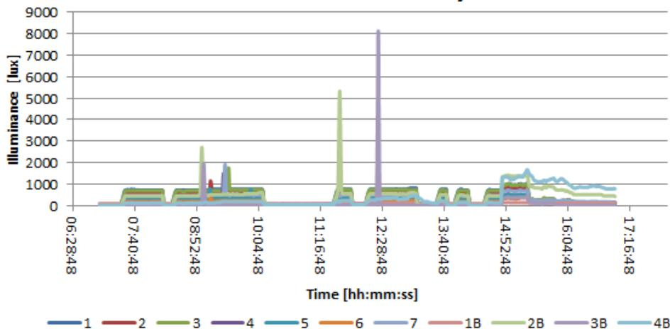
Figure L.5. Interior illuminance when the shading was activated until 14 : 30
