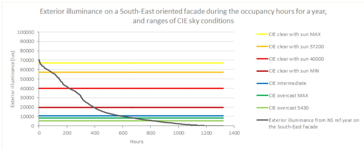
Figure 15.4. The yearly TotVEI from the Norwegian reference year weather file compared to the TotVEI from Relux for different CIE sky conditions on the façade with an orientation of 128 ° during occupancy hours
