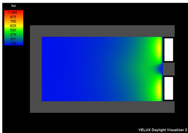
**Figure 4.13.** Photon mapping in VELUX Daylight Visualizer for CIE overcast sky showing illuminance distribution in the cell office with external obstruction
