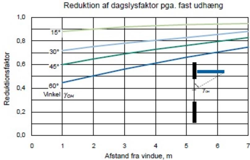
Figure O.10. Reduction factor for different sized overhangs
