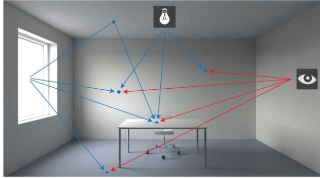
*Figure 4.7.* The photon mapping calculation method (Statens Byggeforskningsinstitut, 2013)
