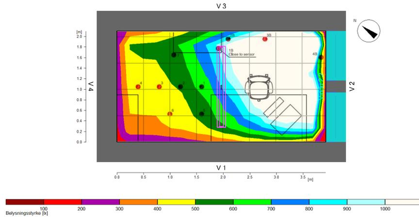
**Figure 4.6.** The ray tracing calculation method in Relux for CIE clear sky showing illuminance distribution in the cell office without external obstruction
