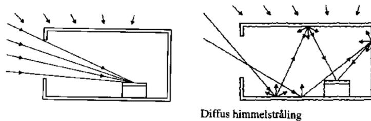
**Figure 14.3.** The direct component to the left and the indirect component to the right for SF2 (Statens Byggeforskningsinstitut, 2010)
