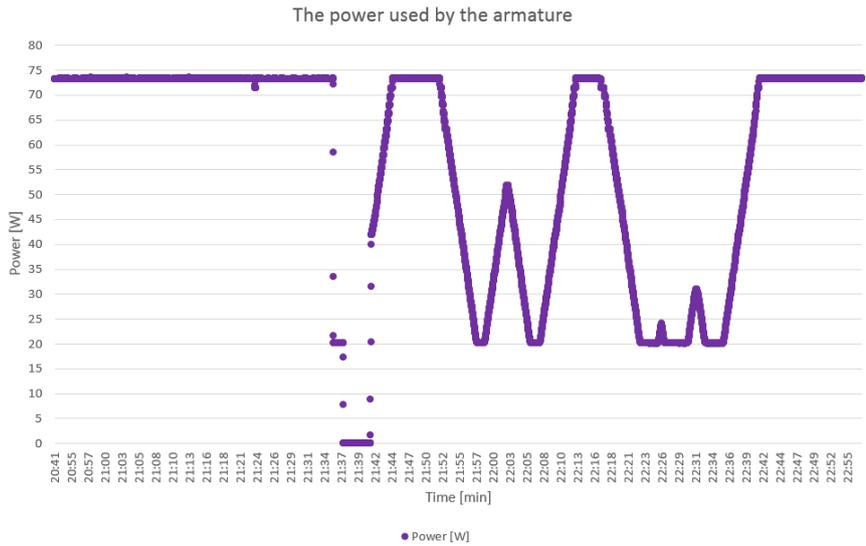
Figure G.10. Measured power for the SparOmeter during the experiment
