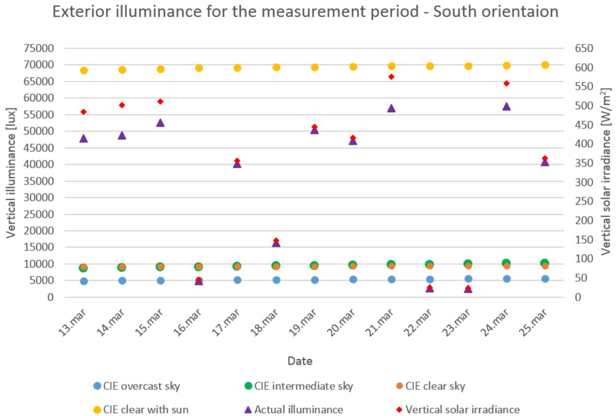
**Figure 5.17.** The exterior illuminance on a vertical reference plane on the south façade at 12:00 for the measurement period comparing vertical solar irradiance and actual illuminance to simulated overcast, intermediate, clear and clear with sun CIE sky conditions.
