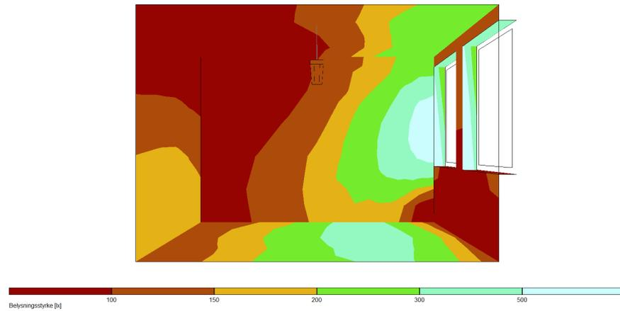
*Figure C.4.* 3D view of the illuminance obtained with the radiosity method in Relux for the cell office without furniture
