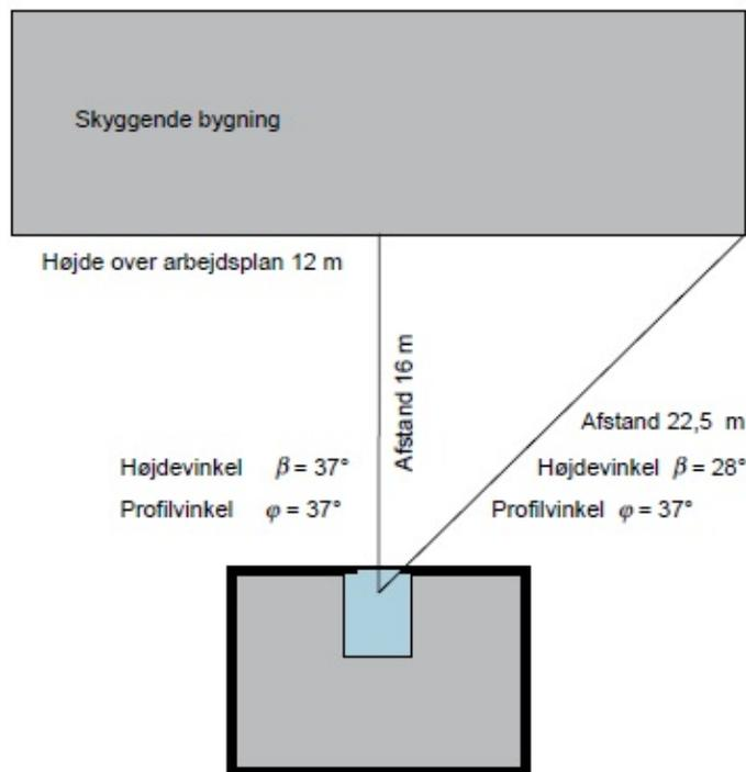
*Figure O.7.* Example on how to determine the profile angle
