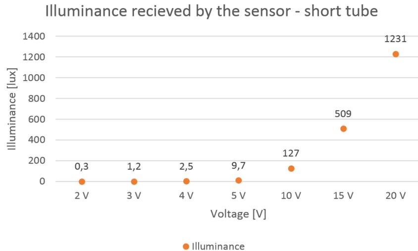
**Figure G.3.** Correlation between voltage input to the light bulb and illuminance received by the sensor
