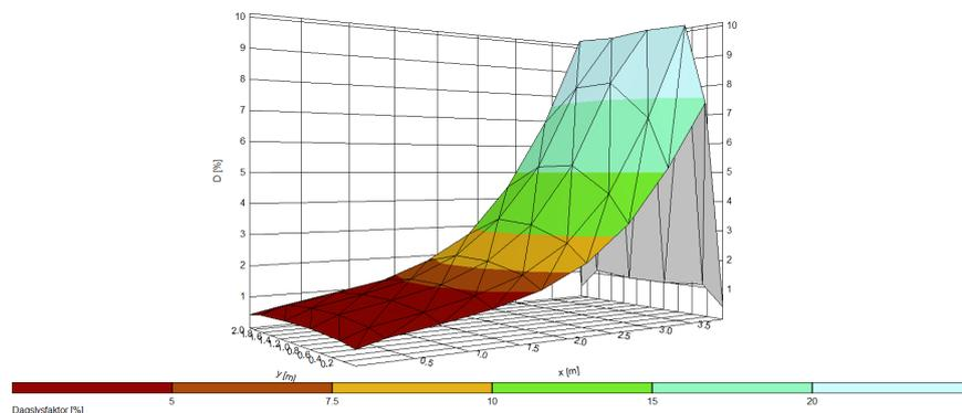
**Figure C.3.** 3D graph of the daylight factor from Relux obtained with the radiosity method for the cell office without furniture
