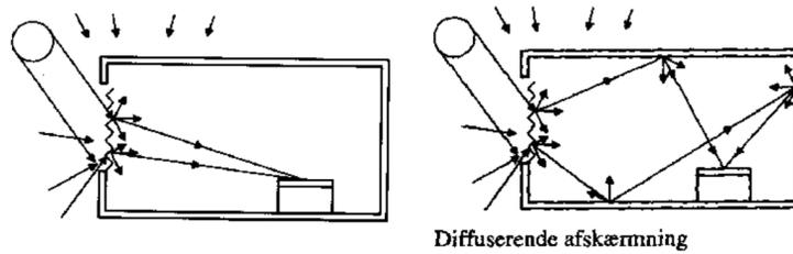
**Figure 14.5.** The direct component to the left and the indirect component to the right for SF4 (Statens Byggeforskningsinstitut, 2010)
