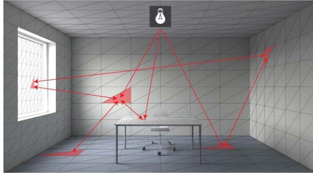
*Figure 4.1.* The radiosity calculation method (Statens Byggeforskningsinstitut, 2013)
