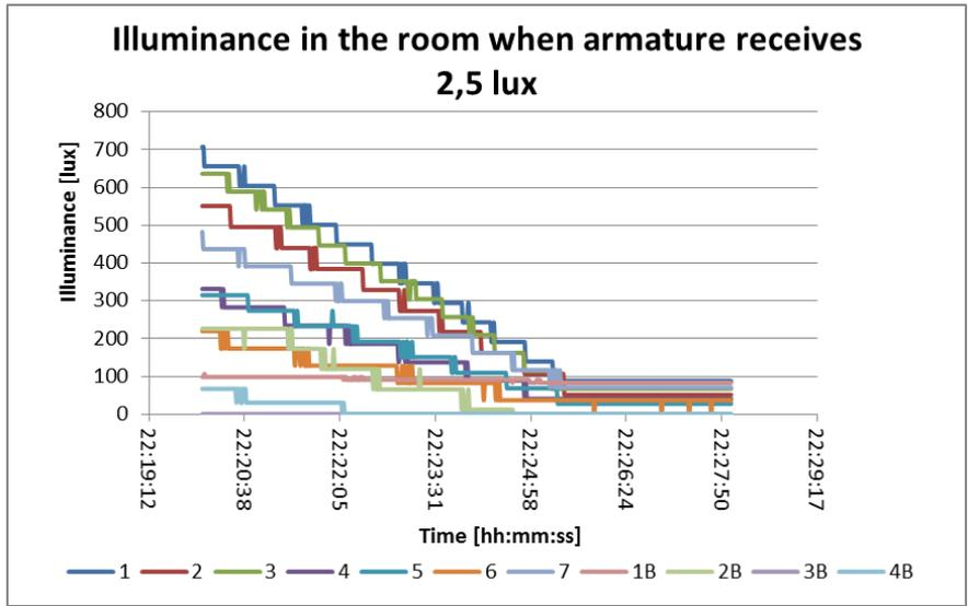
Figure G.9. Illuminance measured by the luxmeters in the room when the daylight sensor receives 2.5 lux
