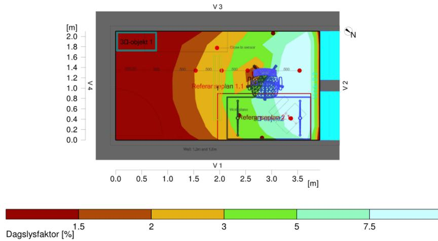
**Figure C.6.** Daylight factor from Relux obtained with the radiosity method for the cell office with furniture
