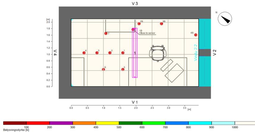
**Figure 4.3.** The radiosity calculation method in Relux for CIE clear sky showing illuminance distribution in the cell office without external obstruction
