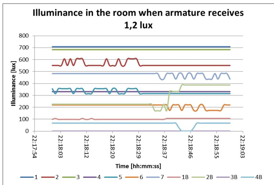
Figure G.8. Illuminance measured by the luxmeters in the room when the daylight sensor receives 1.2 lux
