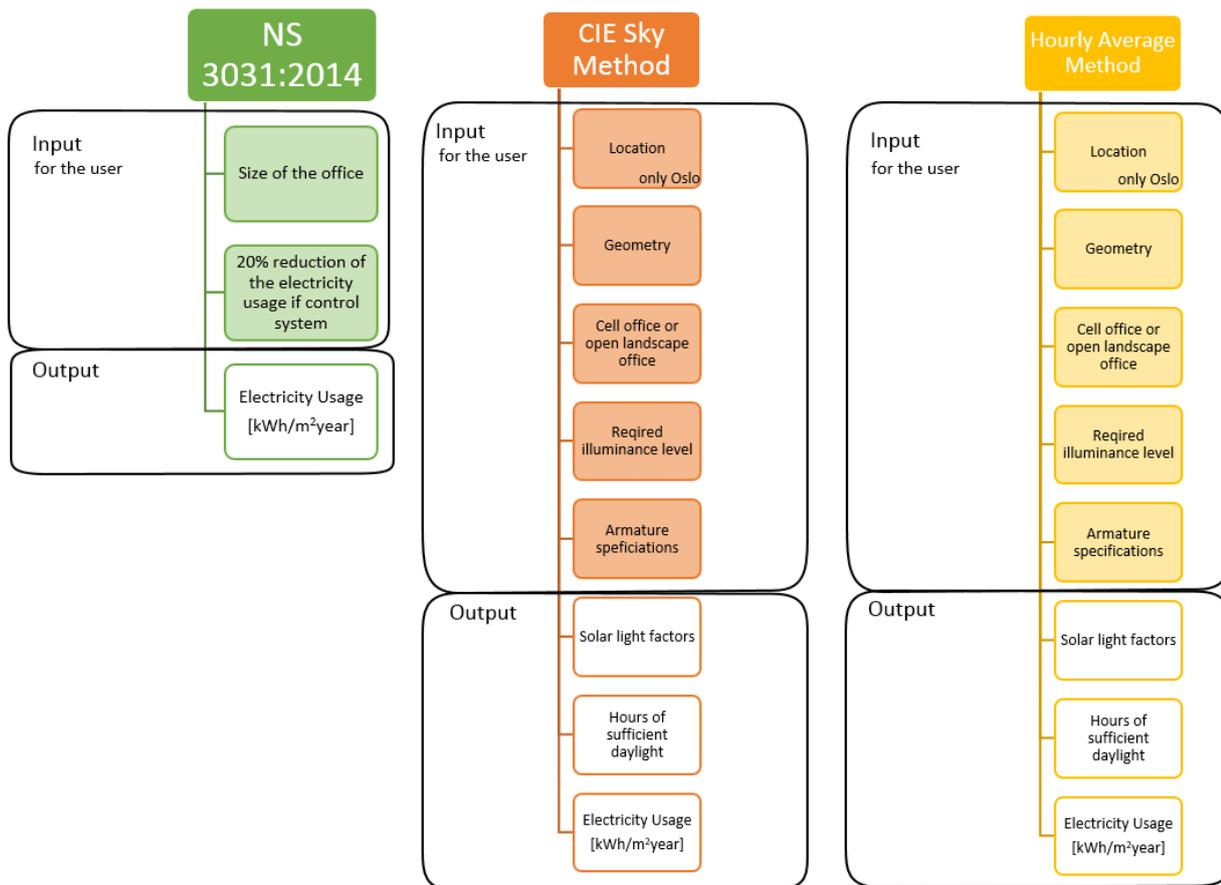
**Figure 14.1.** Illustration of the flow of inputs and output in the three estimation methodologies
