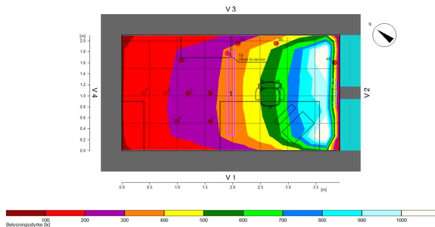
**Figure 4.5.** The ray tracing calculation method in Relux for CIE overcast sky showing illuminance distribution in the cell office without external obstruction
