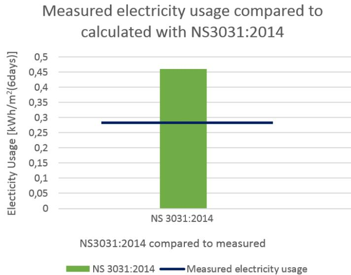
**Figure 13.3.** The calculated electricity usage for the measurement period with the method from *NS3031:2014* compared to the measured electricity usage.
