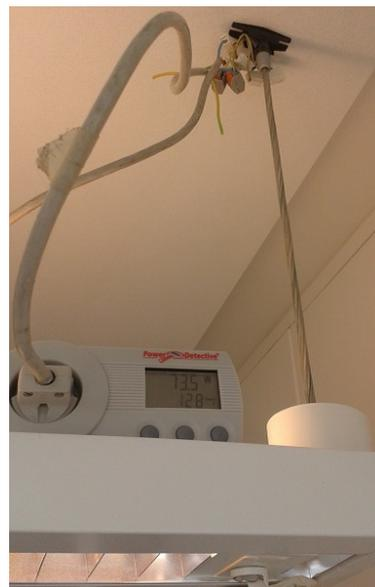
*Figure 2.16.* The electricity usage and power of the armature measured with a SparOmeter
