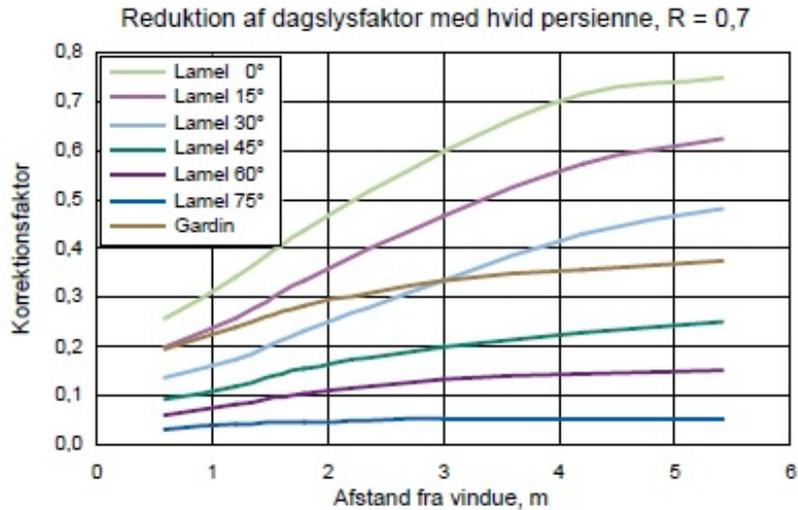
Figure O.14. Correction factor for a white curtain and white blinds positioned in different angles
