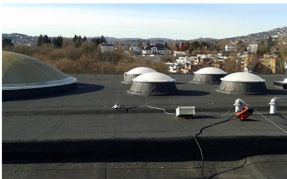
*Figure D.1.* The placement of the pyranometer on the roof
