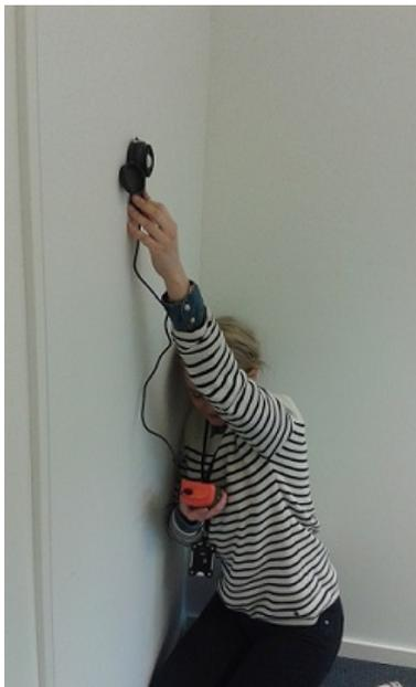
*Figure J.1.* Measuring the illuminance received by the surface
