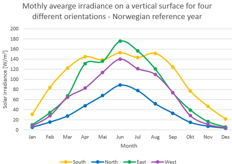
**Figure 5.22.** The monthly average solar irradiance on a vertical surface for the four cardinal orientations for the Norwegian reference year
