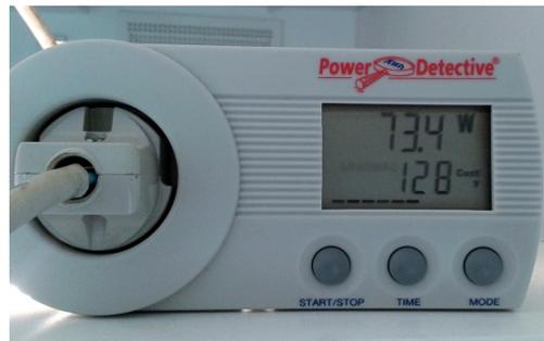
*Figure H.3.* Power Detective SparOmeter measuring the kWh
