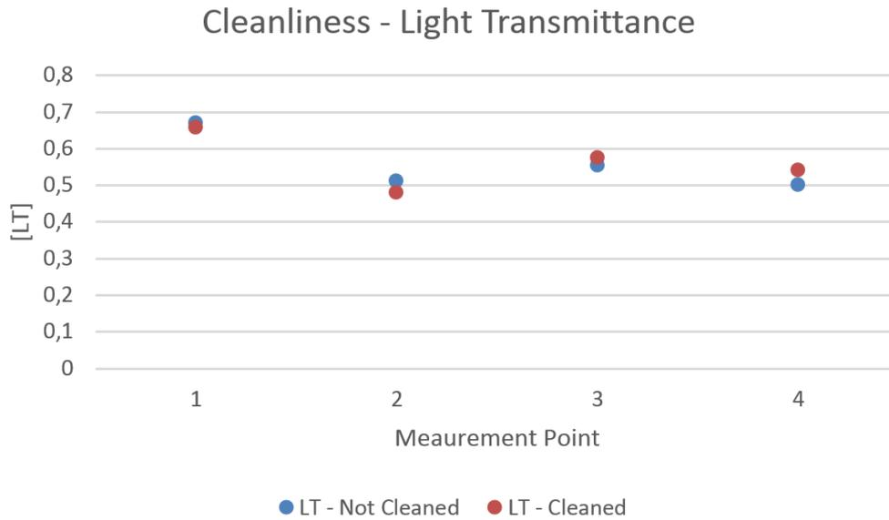
**Figure 3.9.** Light transmittance before and after the glazing was cleaned
