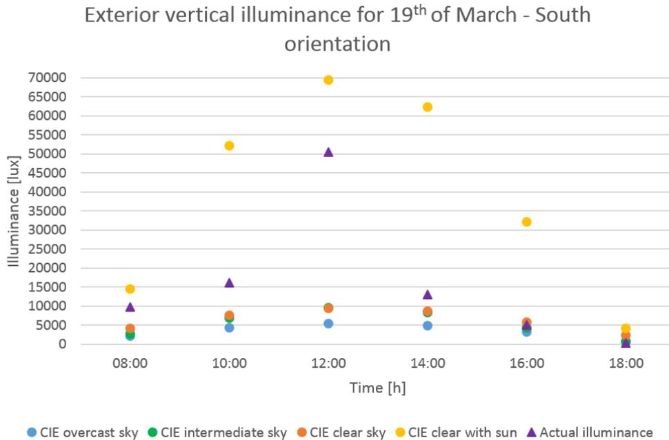
**Figure 5.18.** The exterior illuminance on a vertical reference plane on the south façade at 12:00 for 19<sup>th</sup> of March comparing measured sky to simulated overcast, intermediate and clear CIE sky conditions.
