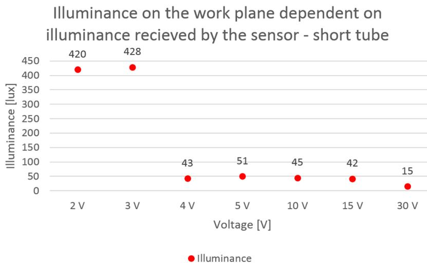
**Figure G.4.** Illuminance measured by the hand-held illuminance meter on the work plane
