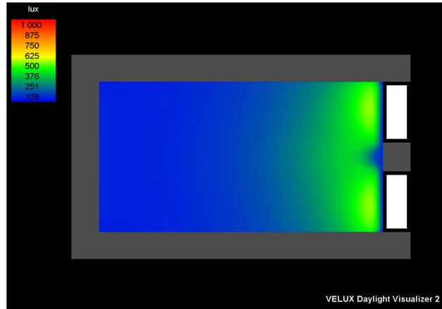
*Figure 4.8.* Photon mapping in VELUX Daylight Visualizer CIE overcast sky showing illuminance distribution in the cell office
