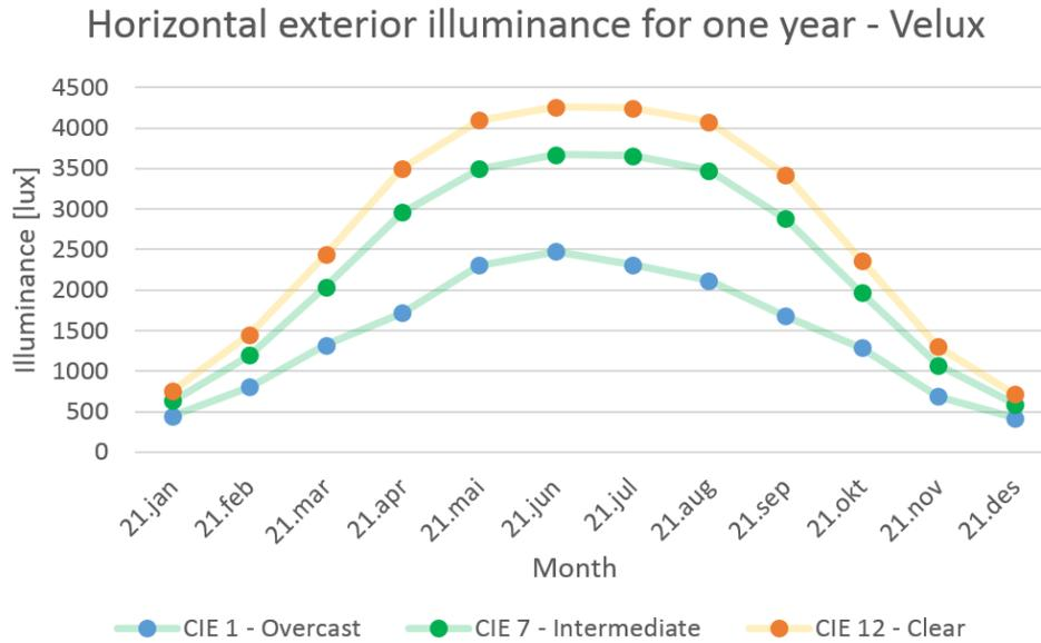
**Figure 5.23.** The exterior horizontal illuminance at 12:00 for the 21<sup>st</sup> of every month of a year comparing the overcast, intermediate and clear CIE sky conditions.
