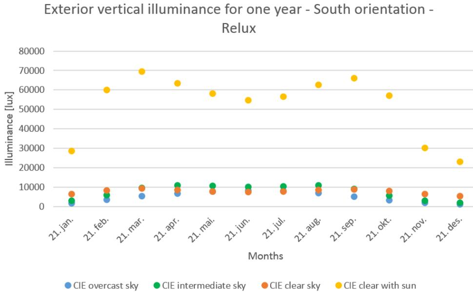
**Figure 5.25.** The exterior illuminance on a vertical reference plane at 12:00 for the 21<sup>st</sup> of every month of a year comparing the overcast, intermediate, clear and clear with sun CIE sky conditions.
