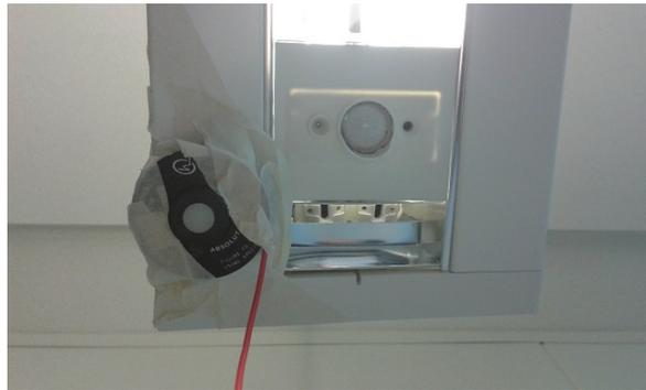
*Figure E.3.* Luxmeter attached to the armature close to the daylight sensor
