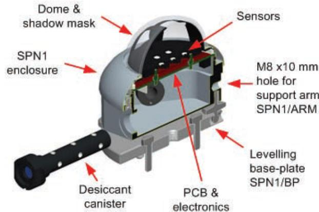
*Figure D.3.* Section of the SPN1 sunshine pyranometer
