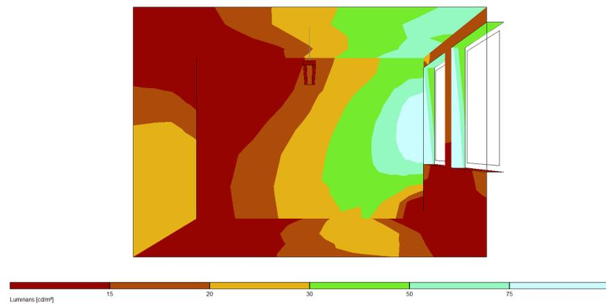
*Figure C.5.* 3D view of the luminance obtained with the radiosity method in Relux for the cell office without furniture
