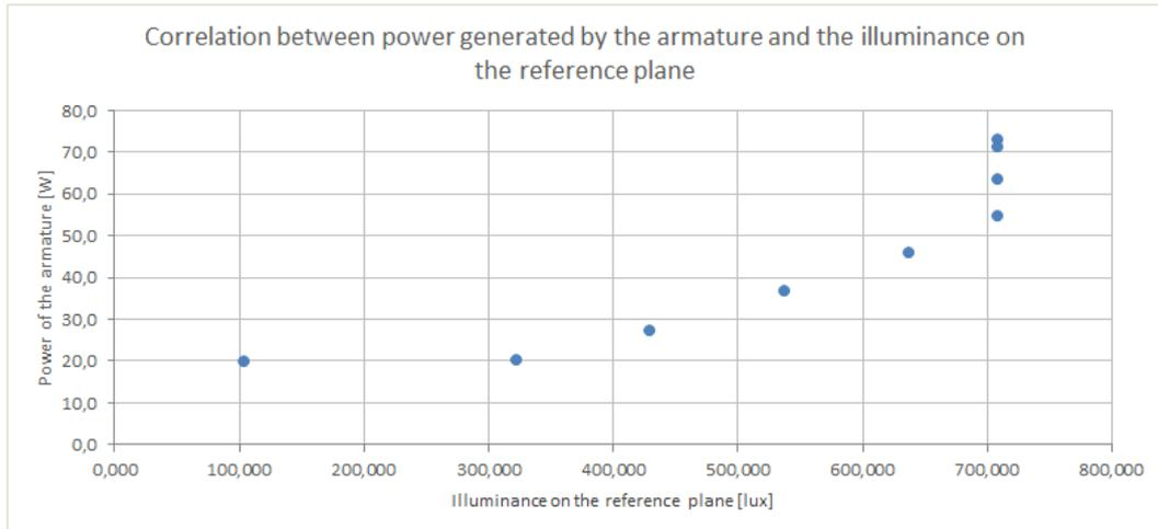
**Figure 6.5.** The correlation between the power of the armature and generated illuminance
