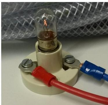
*Figure G.1.* Light bulb used to manipulate the daylight sensor
