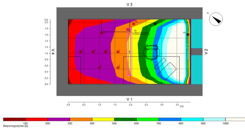
**Figure 4.11.** The radiosity calculation method in Relux for CIE overcast sky showing illuminance distribution in the cell office with external obstruction
