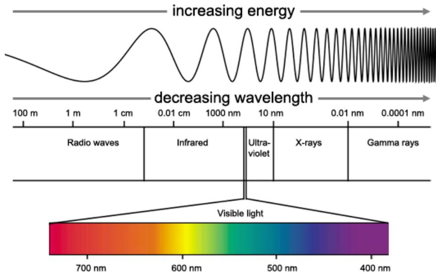
**Figure 3.13.** Different wavelengths and the visible light spectrum (Piatt, January 2015)
