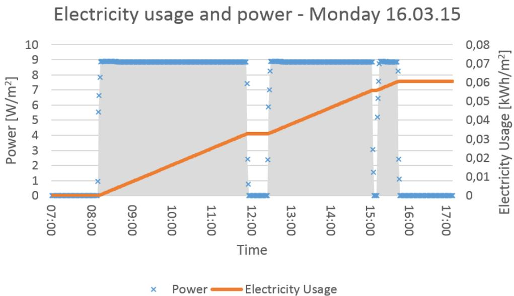
**Figure 6.2.** The power and electricity usage of the armature in the cell office during Monday the 16<sup>th</sup>.
