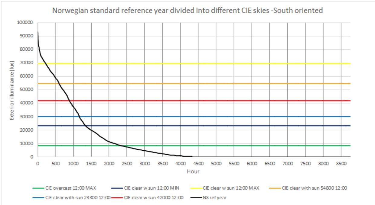
**Figure 5.27.** The exterior illuminance on a South oriented façade from the Norwegian reference year and the different levels of illuminance from the CIE sky conditions, extracted from simulations in Relux
