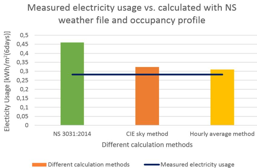
**Figure 17.2.** The calculated electricity usage from the three different methods for the measurement period of 6 days compared to the measured electricity usage
