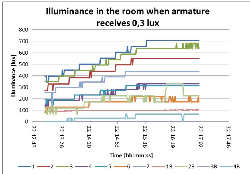
Figure G.7. Illuminance measured by the luxmeters in the room when the daylight sensor receives 0.3 lux
