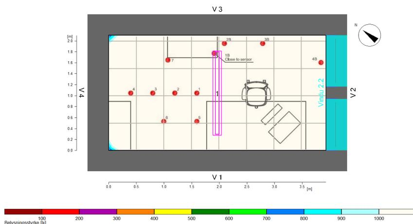
**Figure 4.14.** The radiosity calculation method in Relux for CIE clear sky showing illuminance distribution in the cell office with external obstruction
