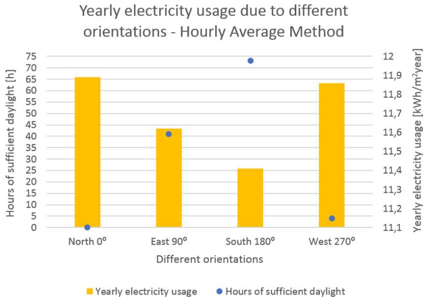
**Figure 16.7.** Hours of sufficient daylight and corresponding yearly electricity usage of the armature calculated with the *Hourly Average Method* with different orientations
