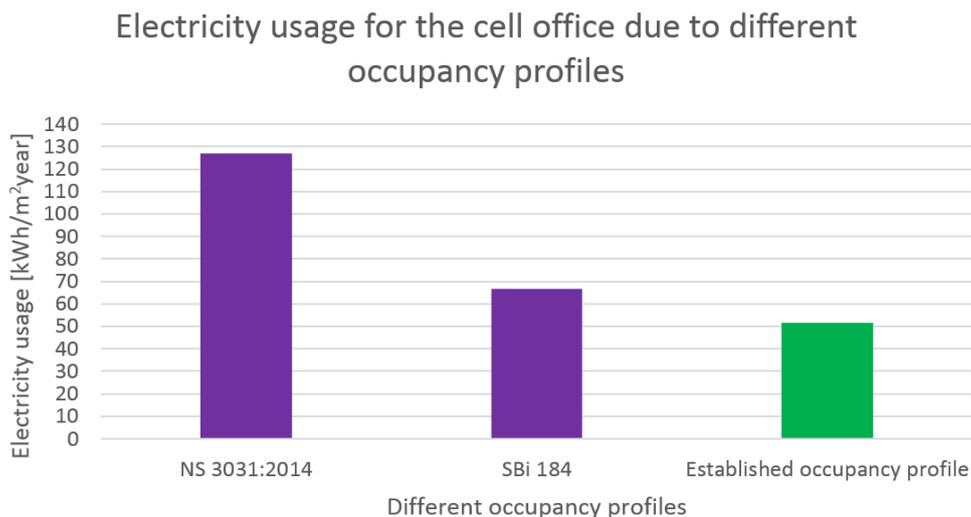
**Figure 12.1.** Yearly electricity usage for the cell office obtained for the established occupancy profile for cell offices compared to occupancy profiles from NS3031:2014 and SBi 184
