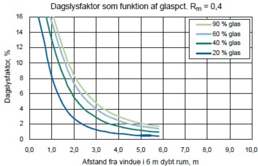
Figure 0.2. Daylight factors for a 6 m deep room with different window areas
