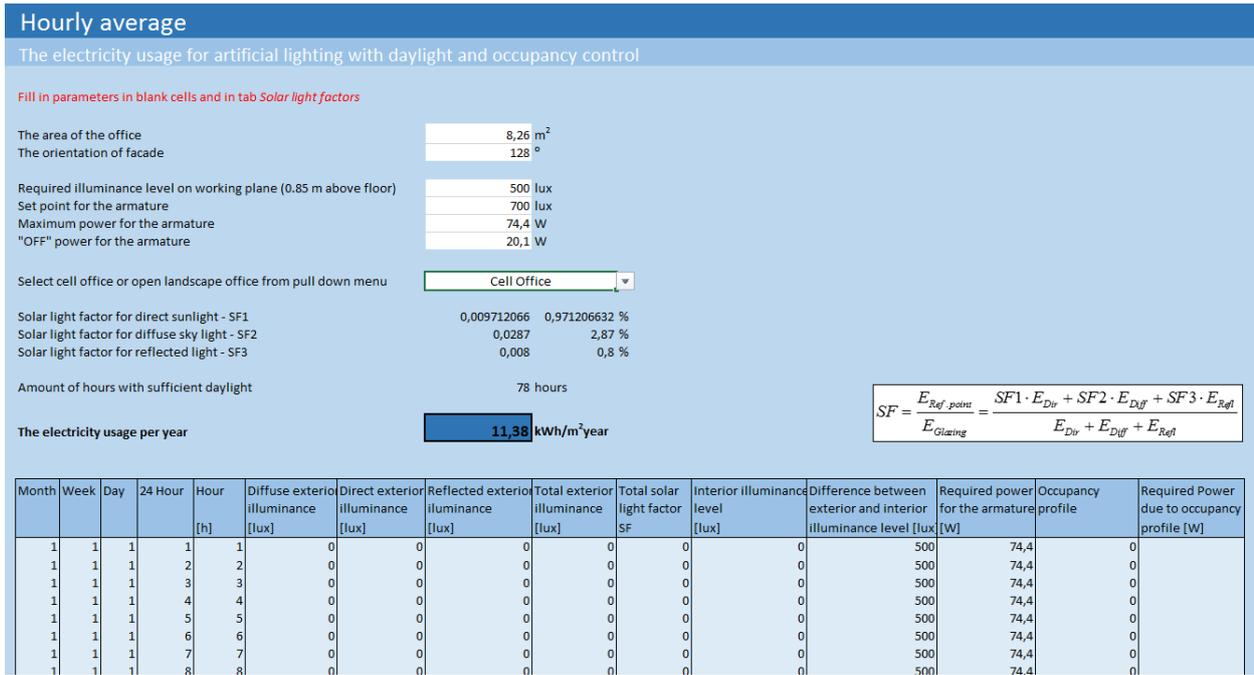
Figure 16.3. Screen shot of the Excel spreadsheet calculating for the hourly average method
