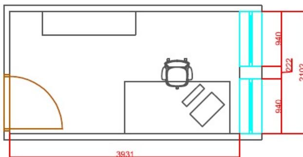
**Figure 2.11.** Plan view of the cell office with dimensions
