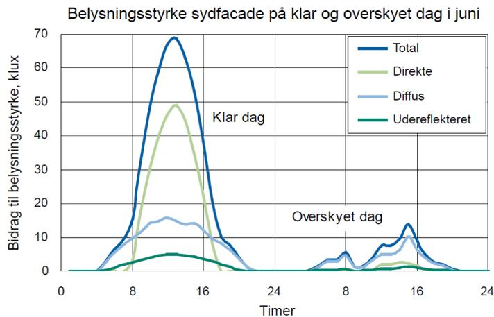
**Figure 14.6.** Typical values of illumination intensity on the South façade for a clear and overcast day in June (Statens Byggeforskningsinstitut, 2008)
