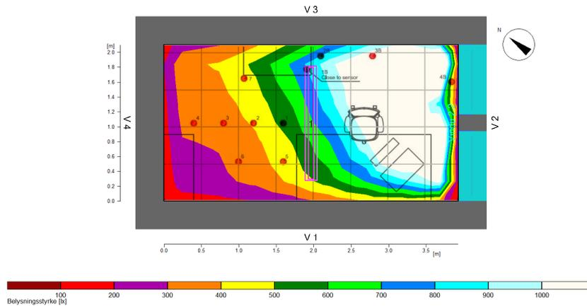
**Figure 4.15.** The ray tracing calculation method in Relux for CIE clear sky showing illuminance distribution in the cell office with external obstruction
