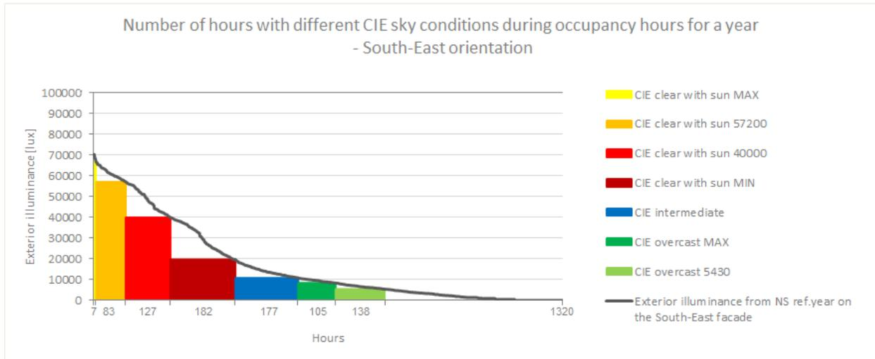
**Figure 15.5.** TotVEI from the Norwegian reference year weather data divided into intervals of hours where different CIE sky conditions occur
