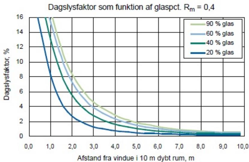
Figure 0.3. Daylight factors for a 10 m deep room with different window areas
