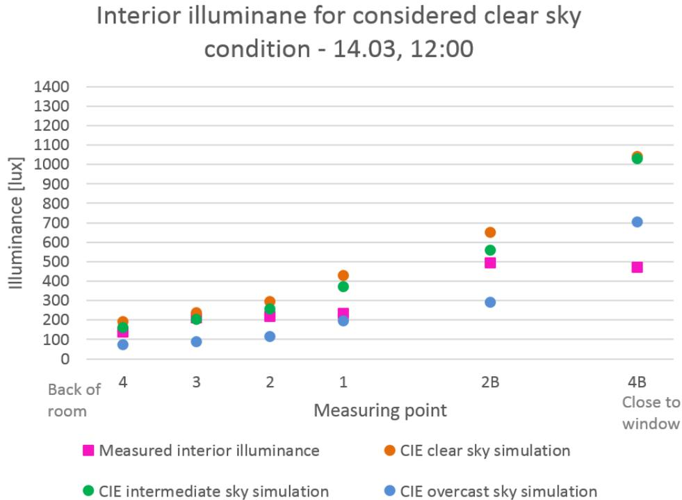
**Figure 5.16.** The interior illuminance for believed overcast sky condition for 14<sup>th</sup> of March compared with simulated interior illuminance for overcast, intermediate and clear CIE sky conditions.
