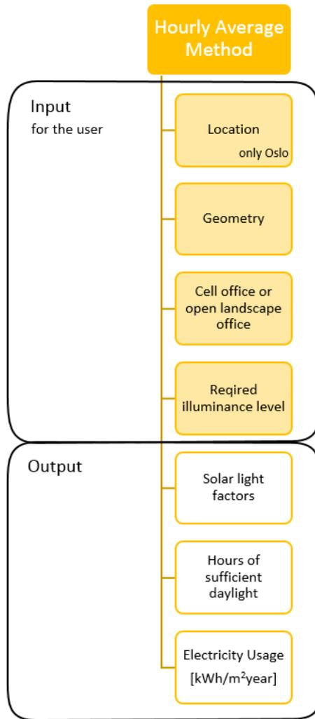
**Figure 16.1.** Illustration of the flow of inputs and output in the *Hourly Average Method*
