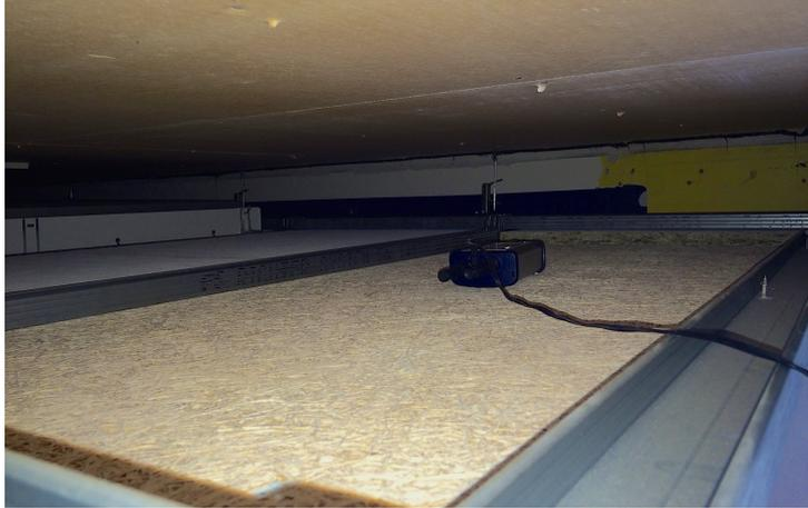
*Figure 3.3: Eltek GD47 wireless transmitter located above diffuse ceiling panel measuring air temperature and CO<sub>2</sub>-concentration.*
