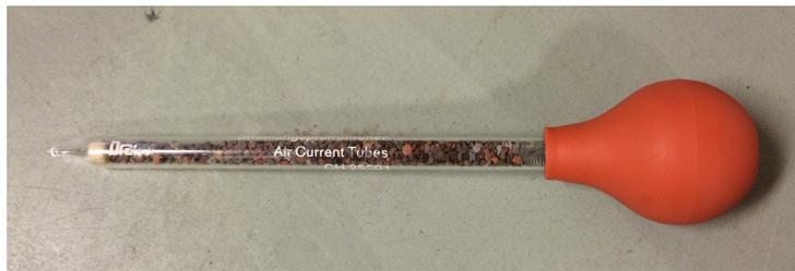
*Figure 2.15: Air current tube used for visualising air distribution by manually injecting smoke to the inlet air.*
