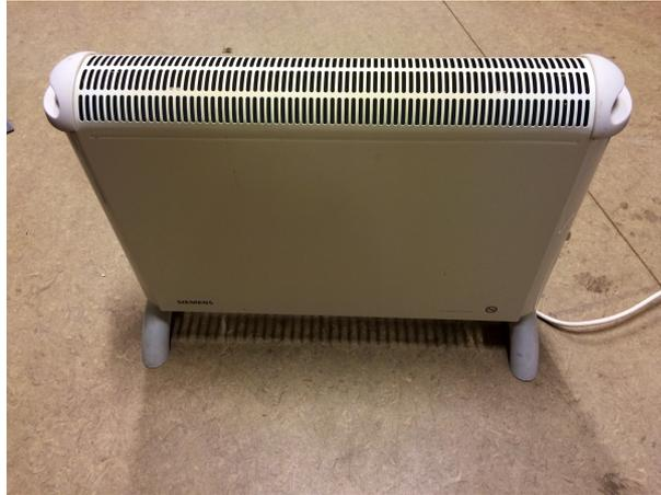
*Figure 4.8: Electrical radiator used for adjusting heat release.*
