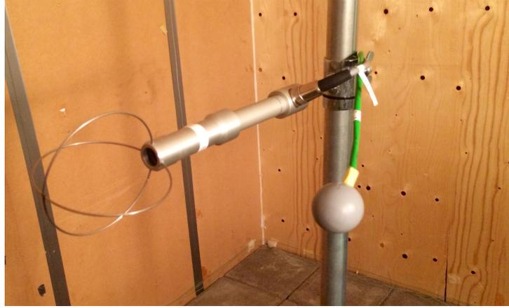
Figure 4.16: Dantec draught probe (shield pulled up) for measurements of air temperature and speed and operative temperature sensor (globe).
