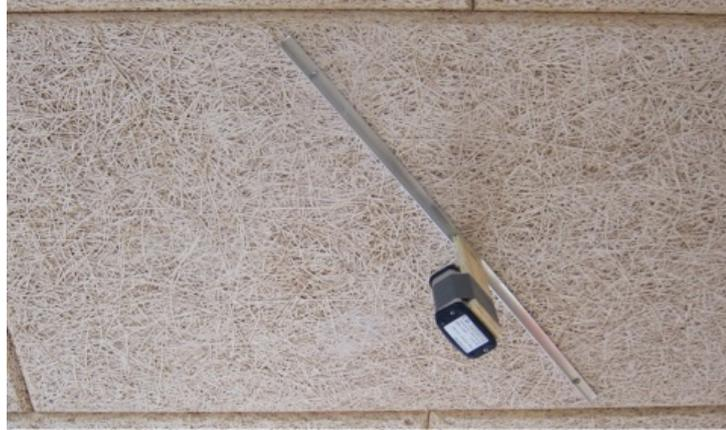
Figure 2.10: Eltek GC10 wireless transmitter attached to diffuse ceiling panel measuring air temperature. The build-in temperature sensor is touching the ceiling panel.
