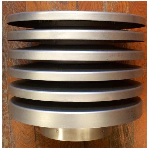
Figure 3.2: Protecting steel frame used for outdoor air measurements.
