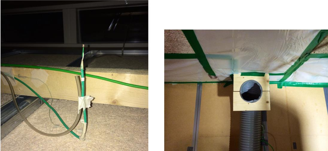
Figure 4.14: Left: Picture of thermocouples and pressure tubes located in plenum. Right: Picture of exhaust duct with thermocouples located in duct.
