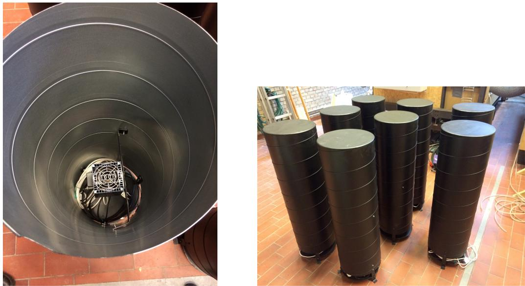
*Figure 4.5: Left: Picture of the heating element inside the thermal manikin used as heat load simulator in experimental setup. Right: Picture of all eight manikins used in the setup.*
