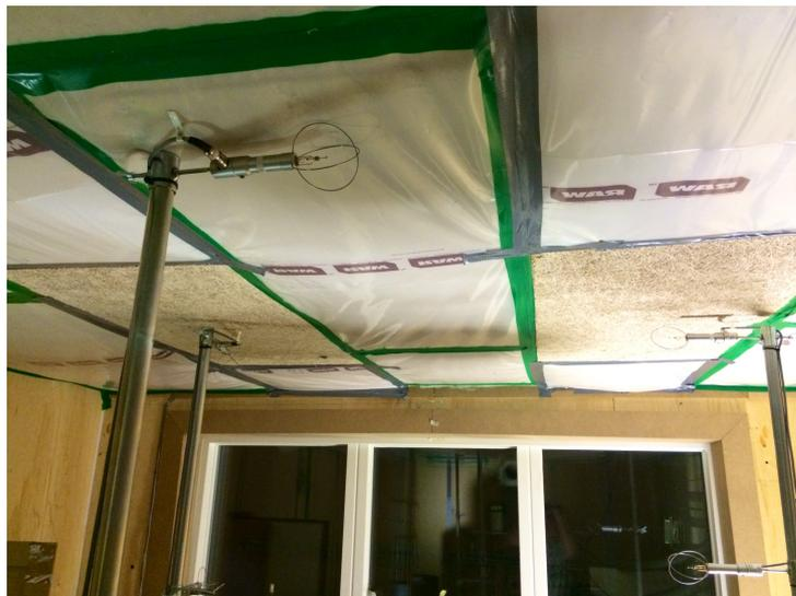
Figure 4.12: Reduced diffuse ceiling area by fitting a vapour barrier on room side of ceiling panels.
