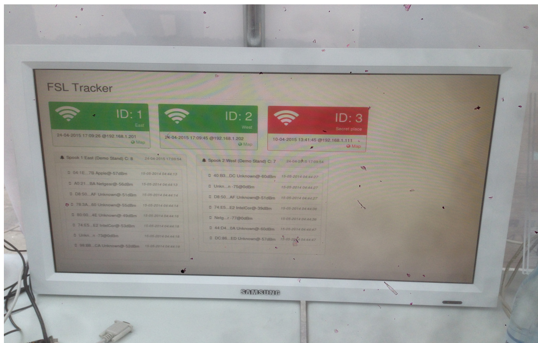
Fig 7: The online status in Central control (Web); Green colour indicates operating system is online and have detected detect many MAC addresses; Red colour indicates the system is offline.
