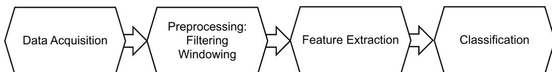
**Figure 2.1:** Pattern recognition-based control systems usually consist of four steps: data acquisition, preprocessing, feature extraction, and classification. Modified from [G. Li, 2011].
