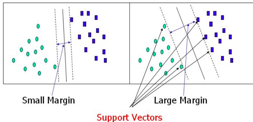
**Figure 6.2:** SVM examples illustrating support vectors and corresponding margins [https://www.dtreg.com/solution/view/20, n.d.].
