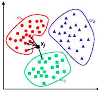
**Figure 6.1:** KNN example using euclidean distance and  $k$  equal to 5
