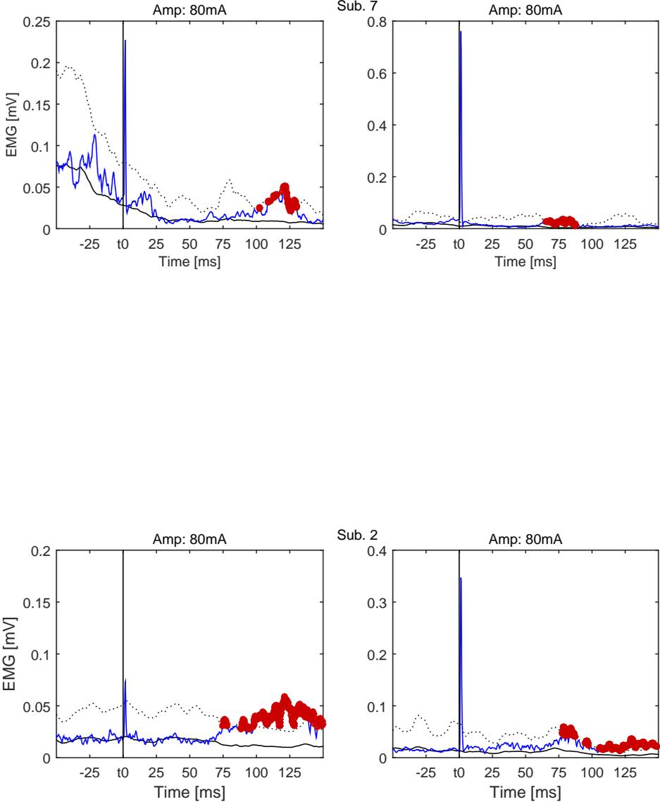
**Figure 9.7:** Example of responses of the Left Biceps Femoris to stimulation of the right sciatic nerve at 50% (left) and 90% (right) of the gait cycle.
