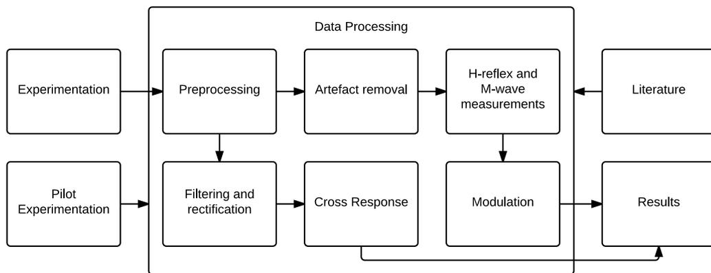
**Figure 5.4:** Workflow of the Dataprocessing chapter. There are two main paths of processing; the first one begins with artifact removal, followed by extraction of the H- and M-waves from both dynamic and static phases, which are then used to produce modulation results. The second line begins with EMG rectification and is followed up by cross response detection.
