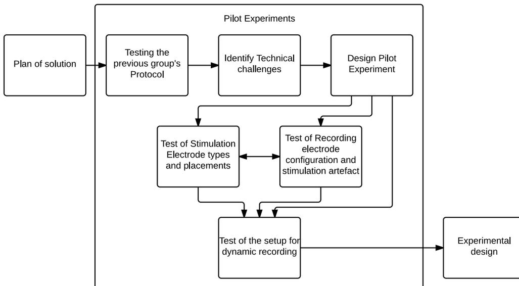
**Figure 5.2:** Work flow of the Pilot Experimentation chapter. The first step of the pilot experimentation chapter is testing out the protocol of [34] based on which a number of challenges are identified and pilot experiments are designed and carried out to produce a setup capable of hamstring H-reflex recording during dynamic movement.
