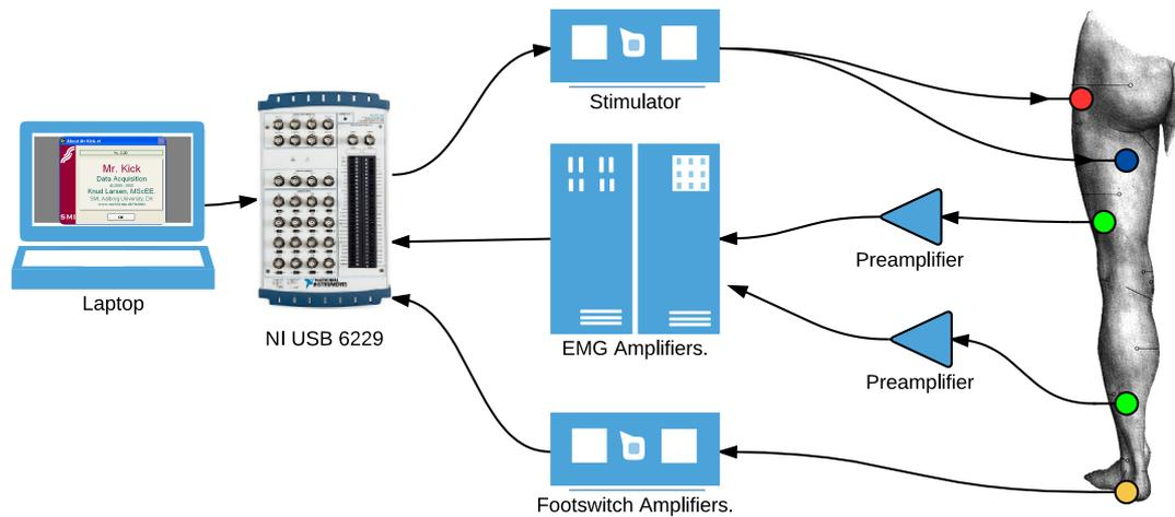
Figure 7.2: The new setup for our dynamic recording experiment.
