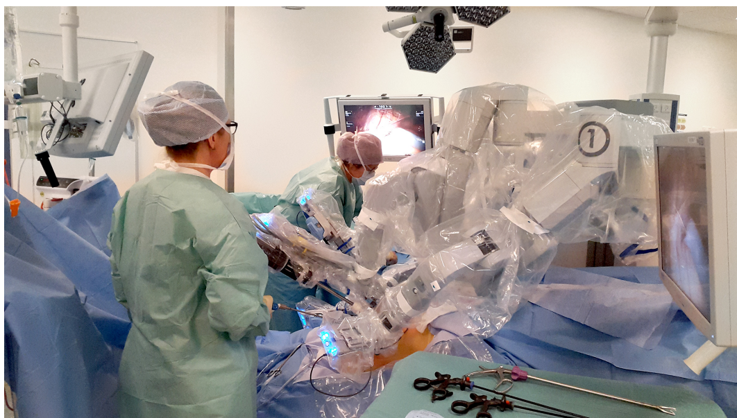
Figure 1.3: Prostatectomy at Aalborg University Hospital conducted by surgeon Grazvydas Tuckus with the da Vinci Xi robot. The robot arms are wrapped in sterile bags.
