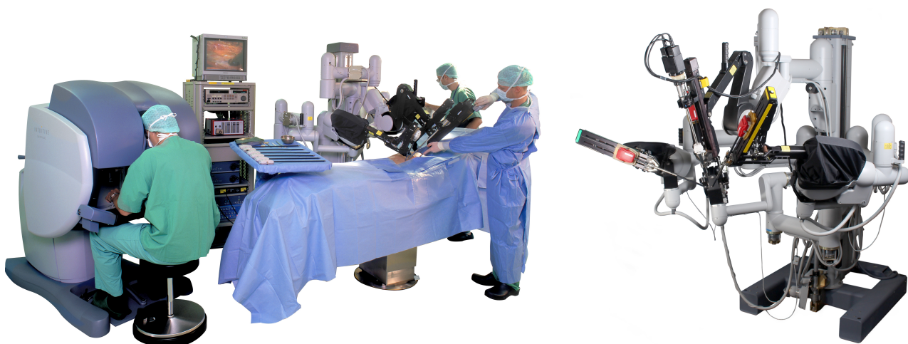
(a) Surgeon master console and slave robotic patient manipulator.
