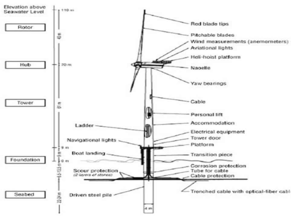
**Figure 9: Main parts of an offshore wind turbine installation (OCS Renewable Energy EIS, n.d.)**
