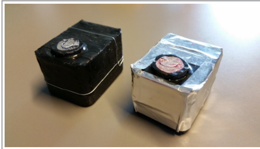
Figure 12: Exterior view of the widgets; the right one with only insulating tape and wires put on, the left one with the metallic tape added.
