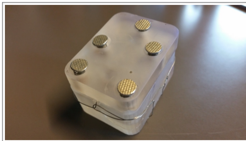
Figure 17: Fourth prototype viewed from the bottom with the nail and spring system added.
