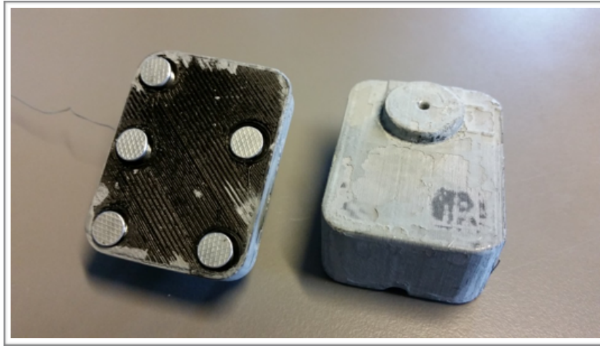
Figure 20: Exterior of the fifth prototype with button platform added and zinc paint applied.
