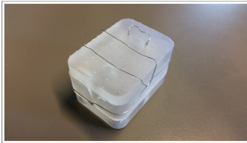
Figure 18: Fourth prototype with top added and wires run around the exterior of the top.
