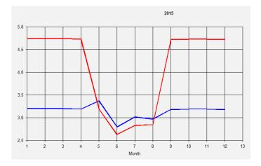
Figure 62: Rate of air flow in the single user's apartment (Bsim)
