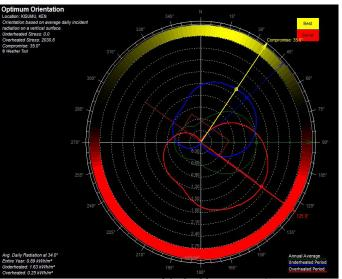
Figure 52:Optimum orientation of the buildings on site( Ecotect Analysis)
