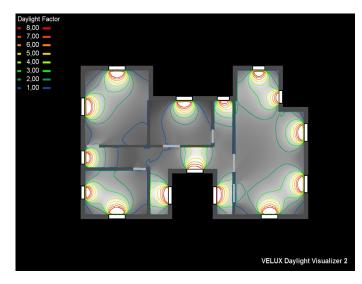
Figure 55: Day light factor in a family unit (Velux daylight visualizer 2)
