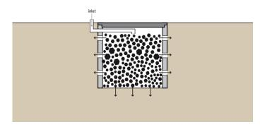
Figure 48: Schematic of a soak pit (Sswm.info, 2015)
