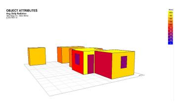
Figure 51: Solar radiation against the north and west facing facades( Ecotect Analysis)
