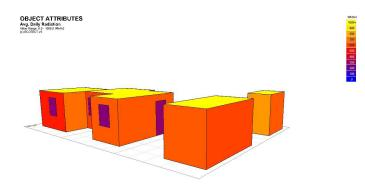
Figure 50: Solar radiation against the south and east facing facades (Ecotect Analysis)
