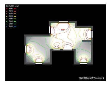
Figure 53: Day light factor in a single's unit (Velux daylight visualizer 2)
