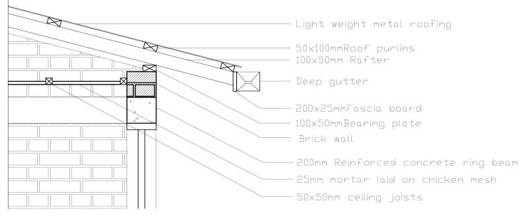
Figure 73 : Roof and open eave detail 1:20
