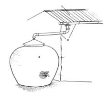
Figure 46: Three basic components of a rain water harvesting system (Sswm.info, 2015)
