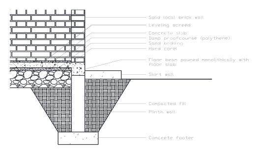
Figure 41: Construction system of a strip foundation
