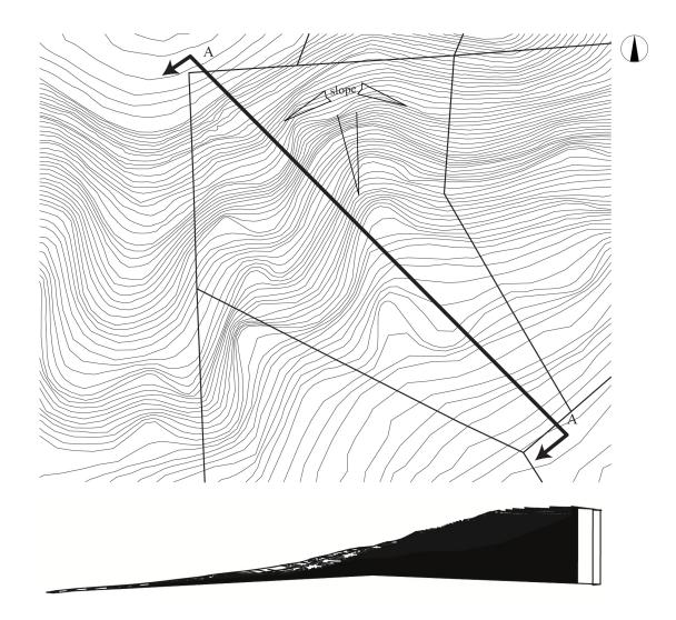
Figure 15: Section A-A through the proposed site, height difference 160metres
