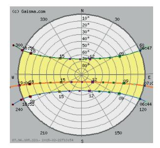
Figure16: Stereographic diagram of the sun's path over Mpirigwa (Source: Gaisma.com)
