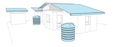
Figure 47: Rain water harvesting system for a single user's unit
