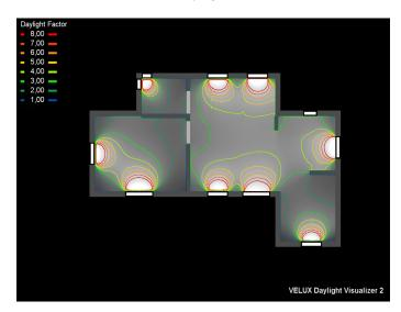
Figure 54: Day light factor in a couple's unit (Velux daylight visualizer 2)
