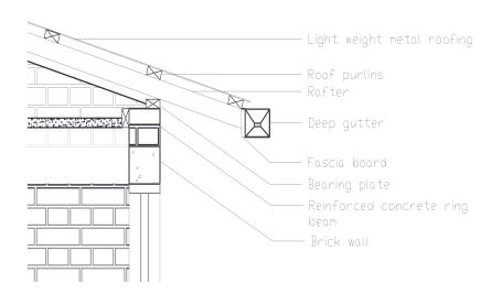
Figure 43: Construction system of the proposed roof
