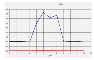
Figure 61: CO2 concenteration in the single user unit under 850ppm(Bsim)
