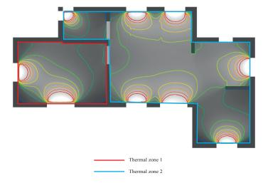
Figure 56: Thermal zones, single user's unit
