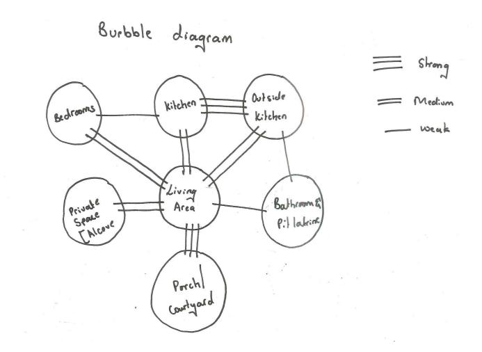
Figure 31: Bubble diagram showing the relationship between the spaces
