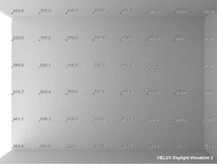
Luminance values of the adjacent wall on a sunny day, with outside reflector
