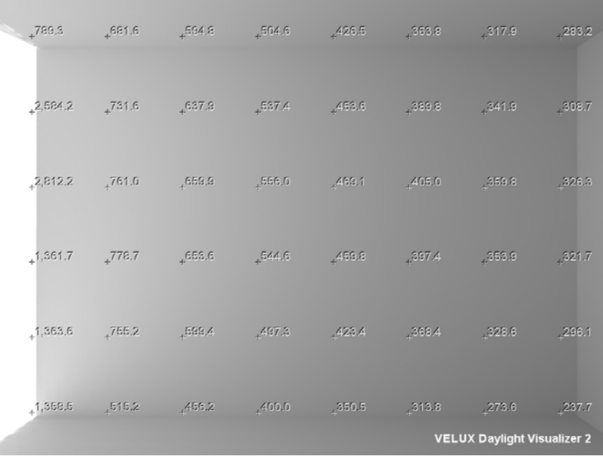
Luminance values of the adjacent wall on a sunny day, without outside reflector
