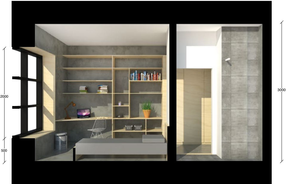
III. 64.3: Section of the dorm single unit, scale 1:50
