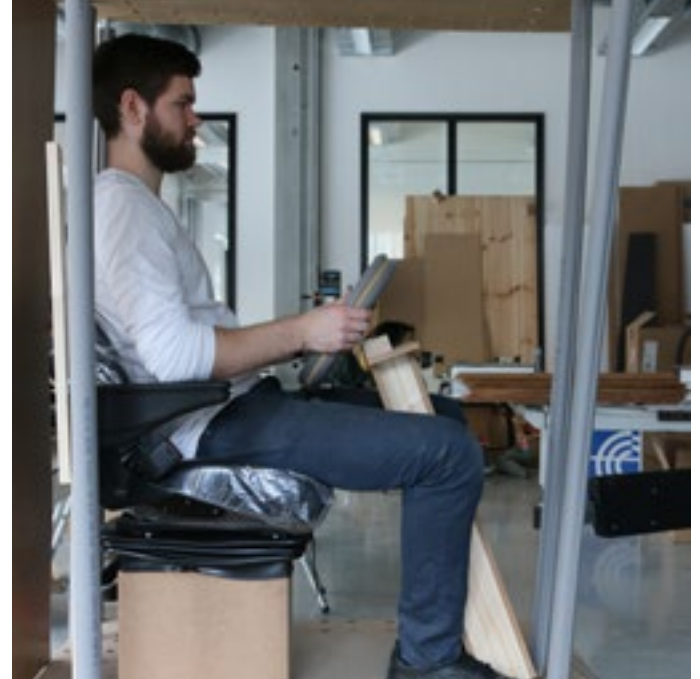
ill 163. Testing visibility over steering wheel
