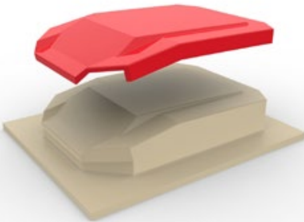
VACUUM MOLD WITH FINISHED PART
