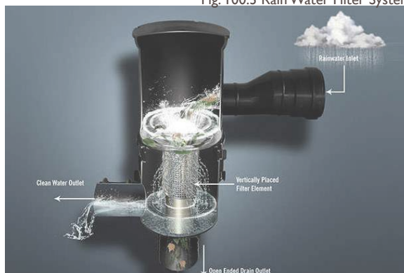
Fig. 100.3 Rain Water Filter System
