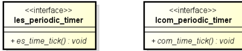
Figure 7-1 Periodic timer interface implemented by Event Service and COM-Service
