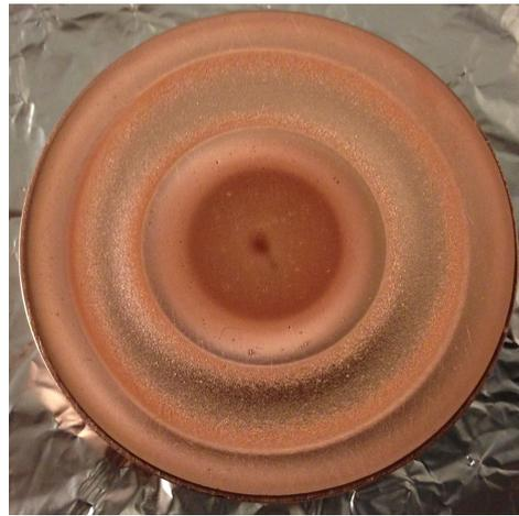
**Figure 2.9.** A copper target nonuniformly eroded by the magnetron sputtering process.
