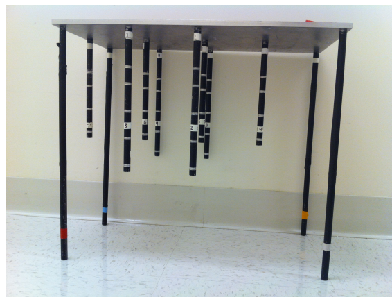
Figure 5.4: Illustrates the calibration device that was used for the calibration of the two infrared cameras, which was used to collect the kinematic data. Each of the reflective points on the 8 pins was marked in the Peak Motus system.
