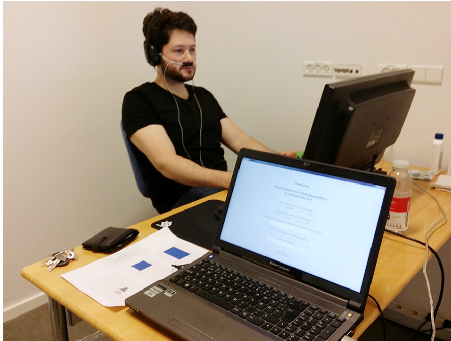
Figure 5.1 – A test participant wearing the headphones and sensors. The test application was run on the laptop and the screen was mirrored on a monitor facing the test participant. Checking of sensor signals was done with the monitor turned off, so only the experimenter would see the pulse wave and respiratory signals on the laptop display.
