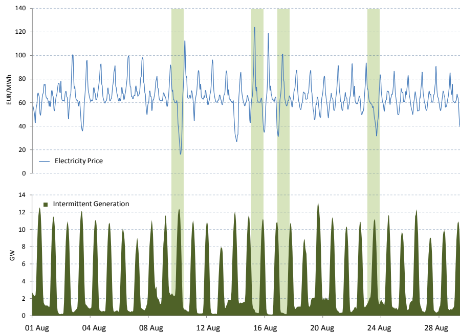
Figure 12: Day-ahead PUN in relation to wind and solar production in Italy. Low intermittent RE results in high electricity prices, while high RE results in low electricity prices. Data elaborated from GME[1] .
