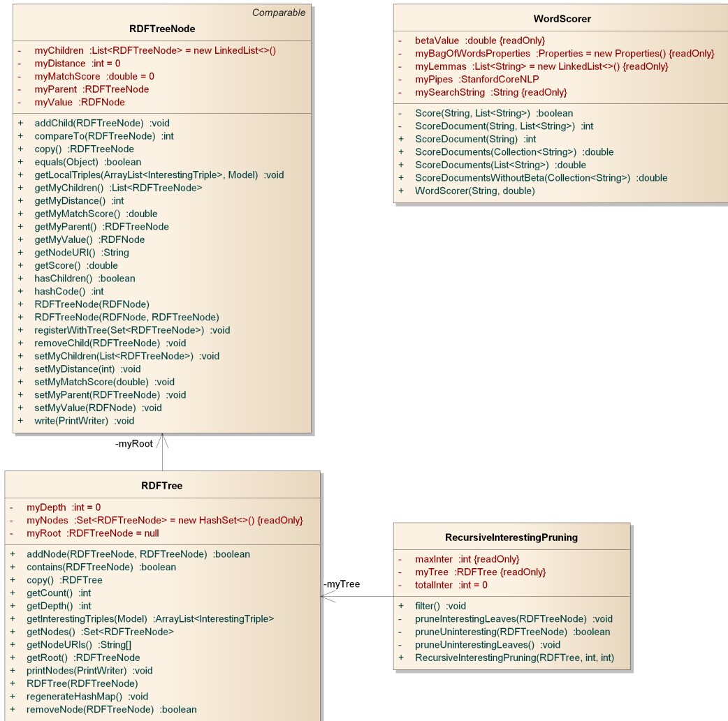
Figure E.4: RDFTree, node, filter and WordScorer classes
