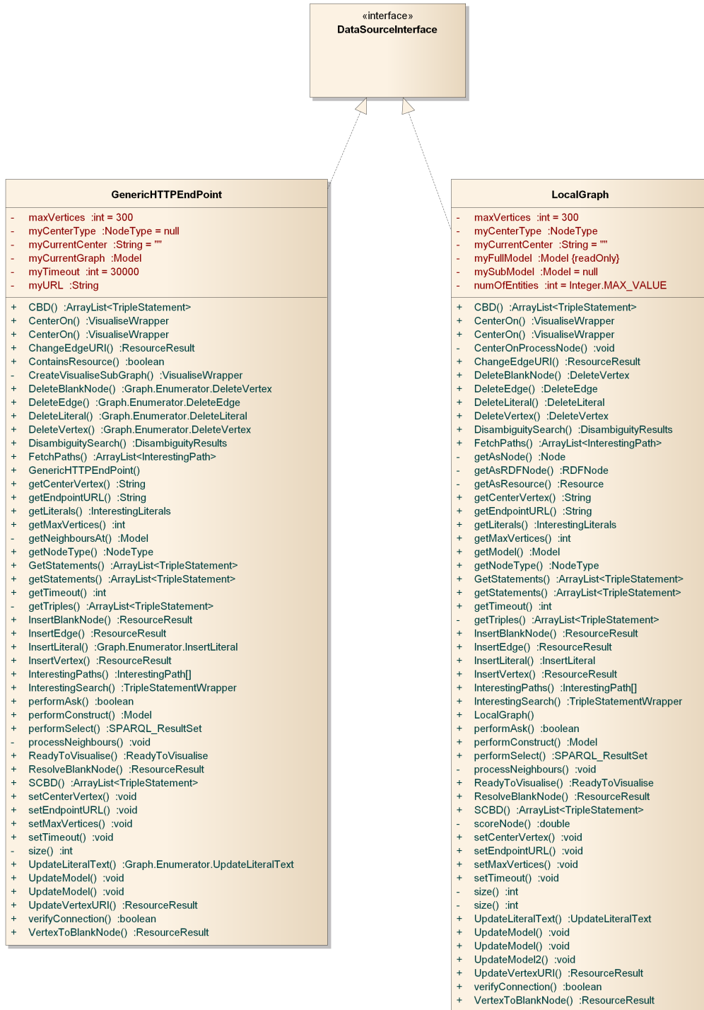
Figure E.5: DataSourceInterface, GenericHTTPEndPoint and LocalGraph classes
