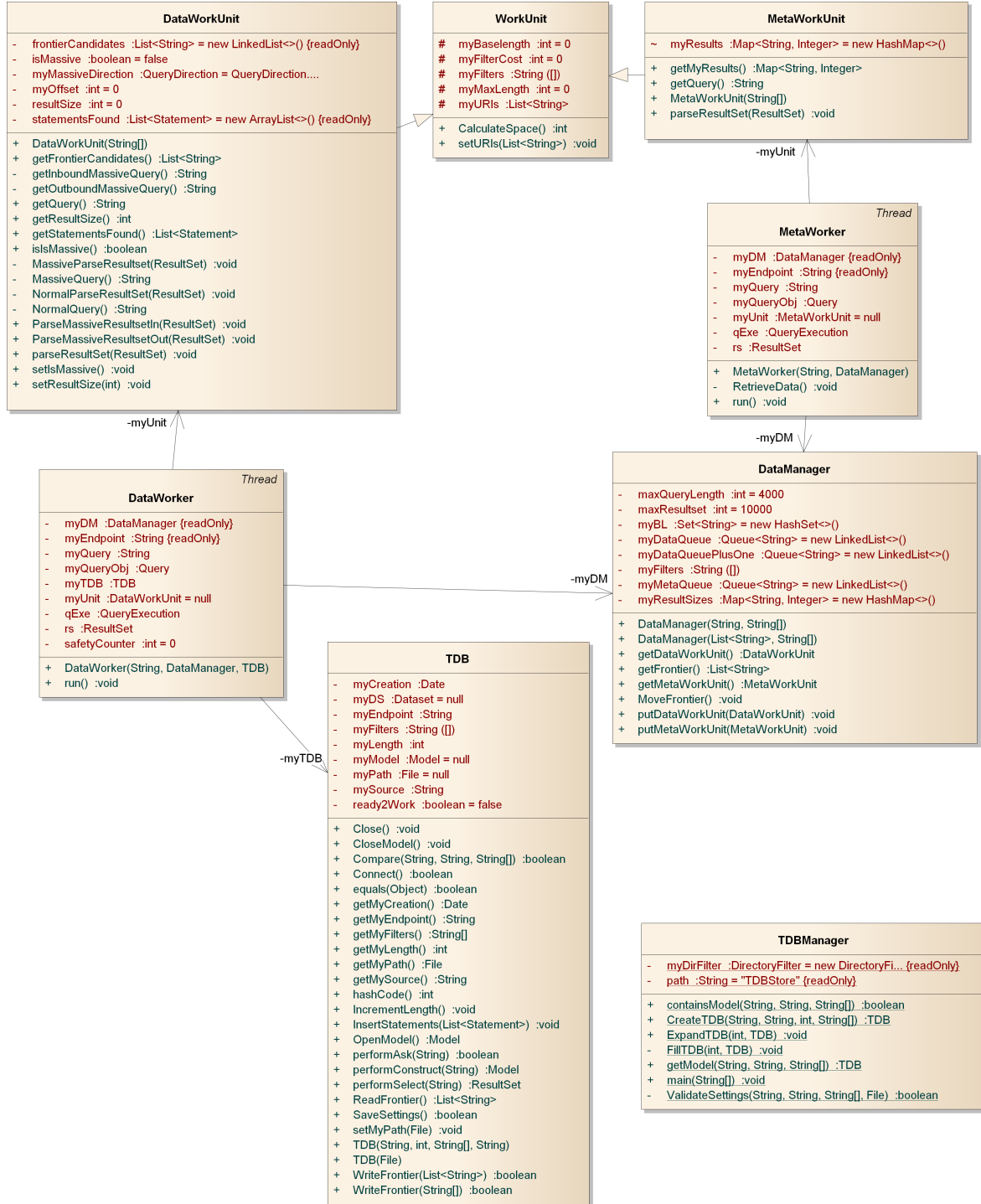
Figure E.1: Full class diagram for the PBBFS algorithm
