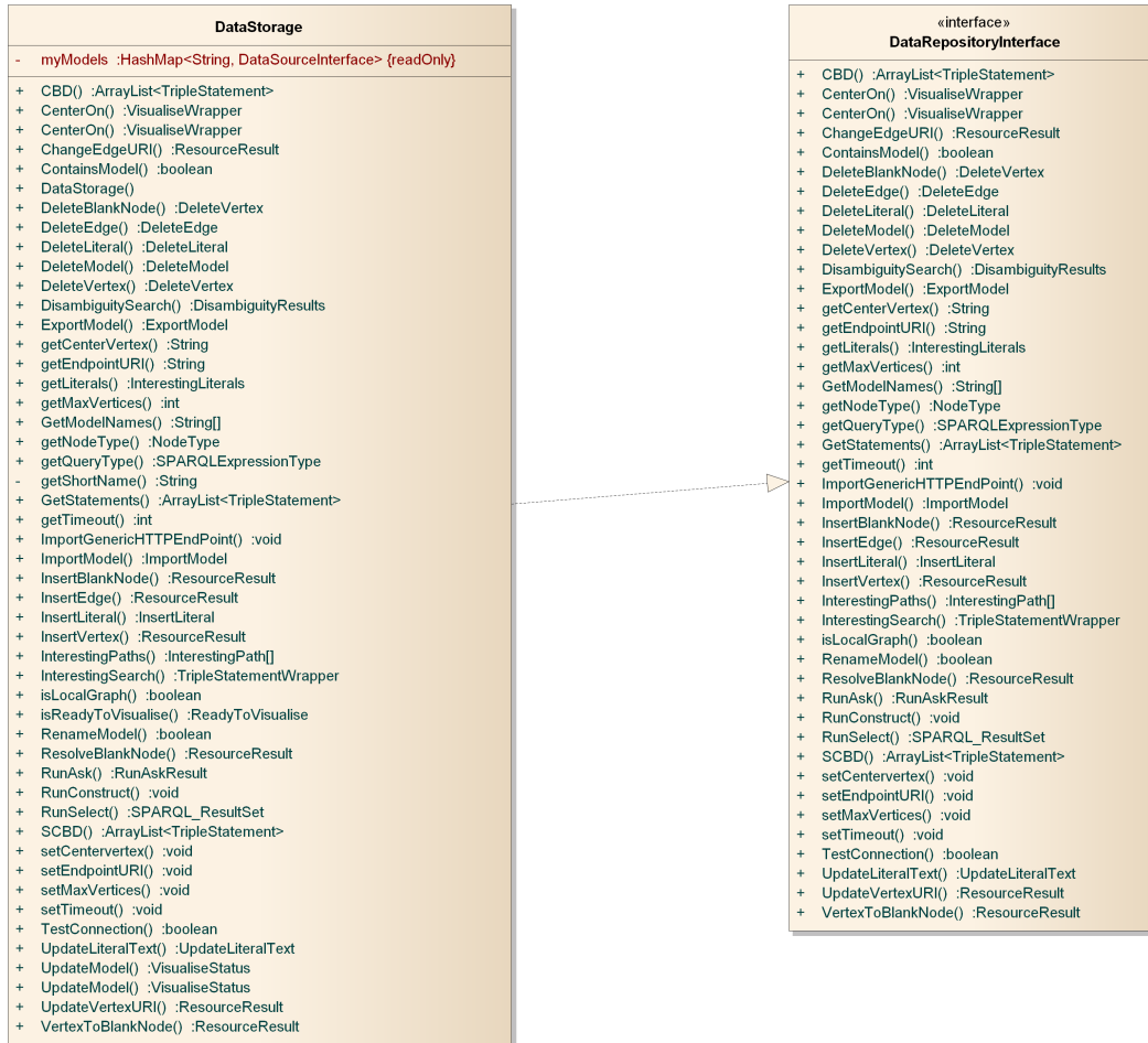
Figure E.6: DataStorage and DataRepositoryInterface classes
