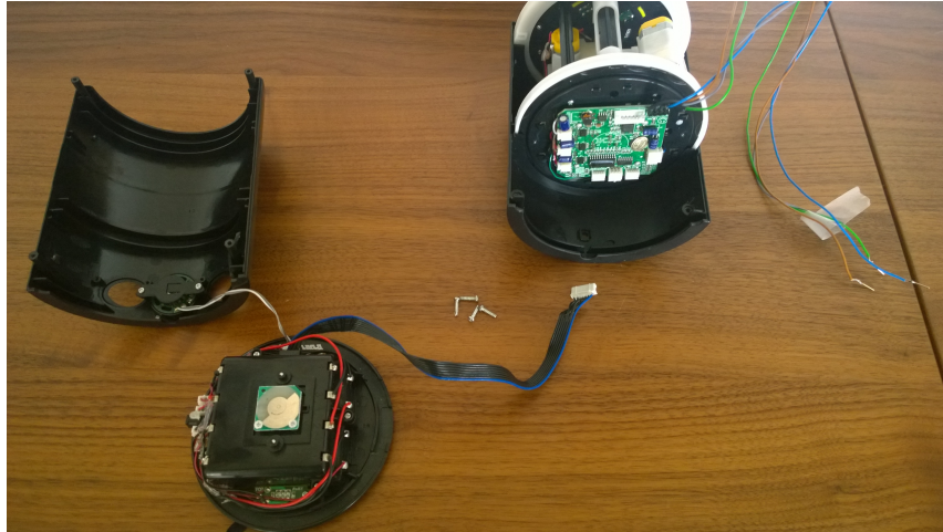
Figure A.2: My Keepon opened and the black/blue cable unplugged
