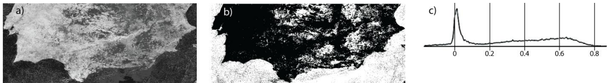
Figure 19 - a) Original image, clipped to the southern part of the Iberian Peninsula b) Pixels with NDVI < 0.07 (in white). c) Image histogram
