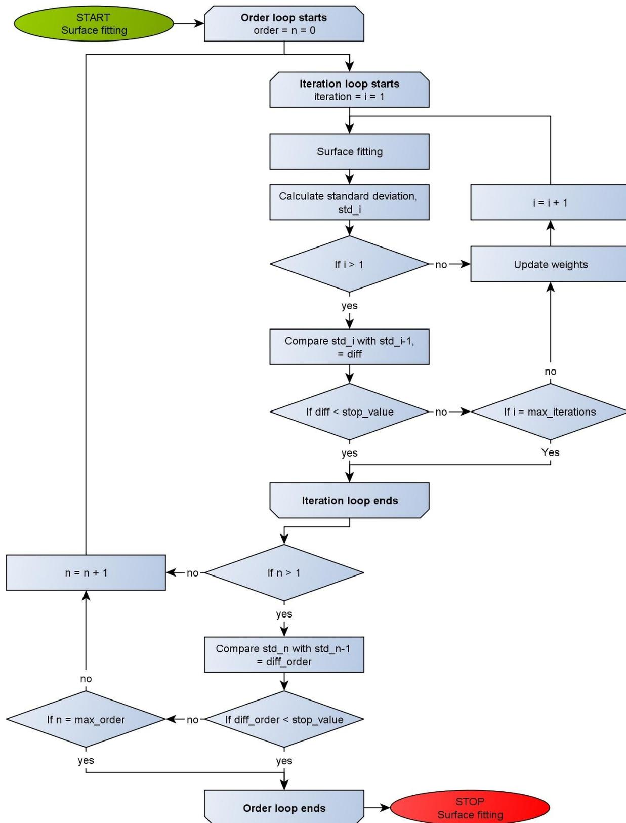
Figure 30 – Flow diagram for the automatic order and iteration detection
