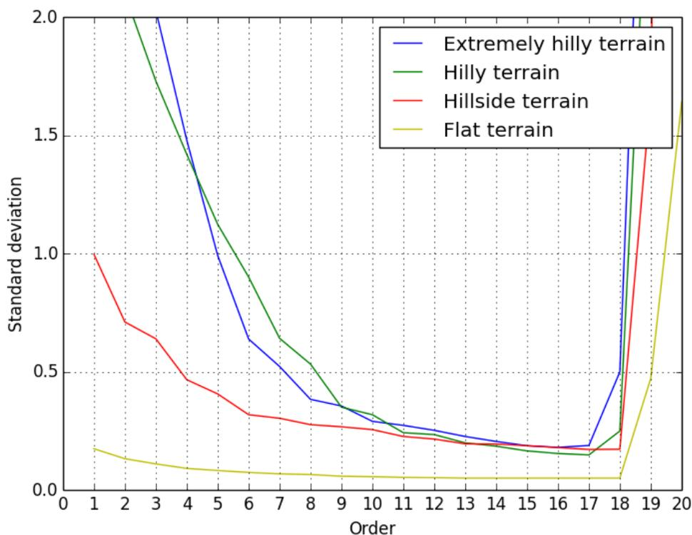
Figure 31 - The standard deviation of unit weight at different polynomial orders and with different terrain types(Matthesen og Schmidt 2014, 91)
