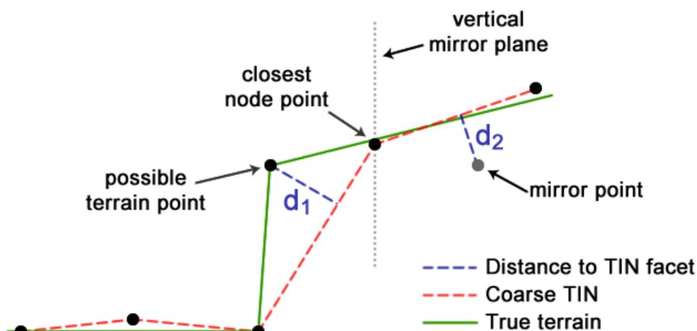
Figure 11 – Mirror points are used to handle discontinuities
