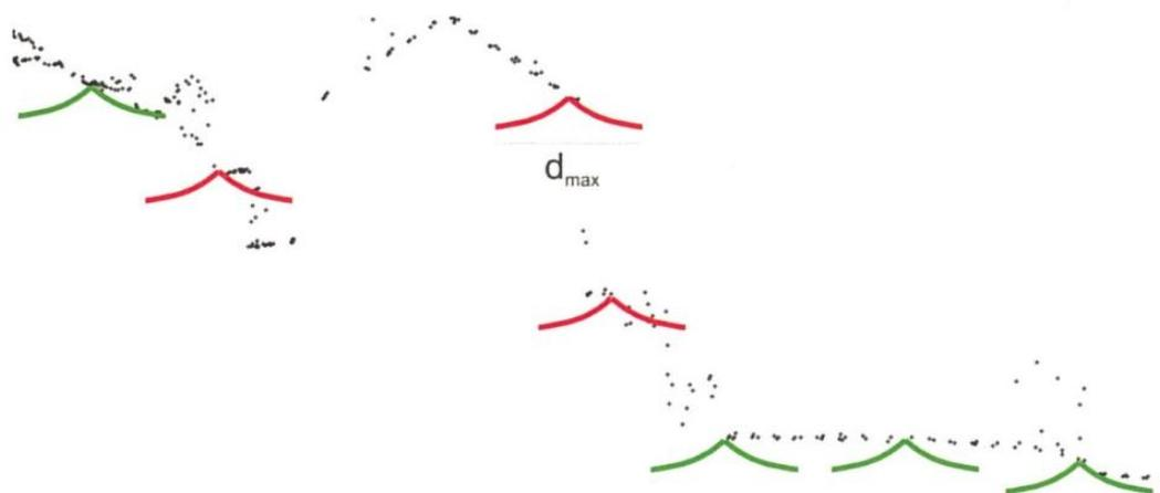
Figure 9 - A structure element with the size  $d_{max}$  is positioned at each point. For selected points, the evaluation function is shown. A green evaluation function means that the point is a terrain point, since no points are below the evaluation function. A red evaluation function means that the point is classified as non-terrain, since there are points below the function. (Vosselman [1] and Mass 2010, 141)
