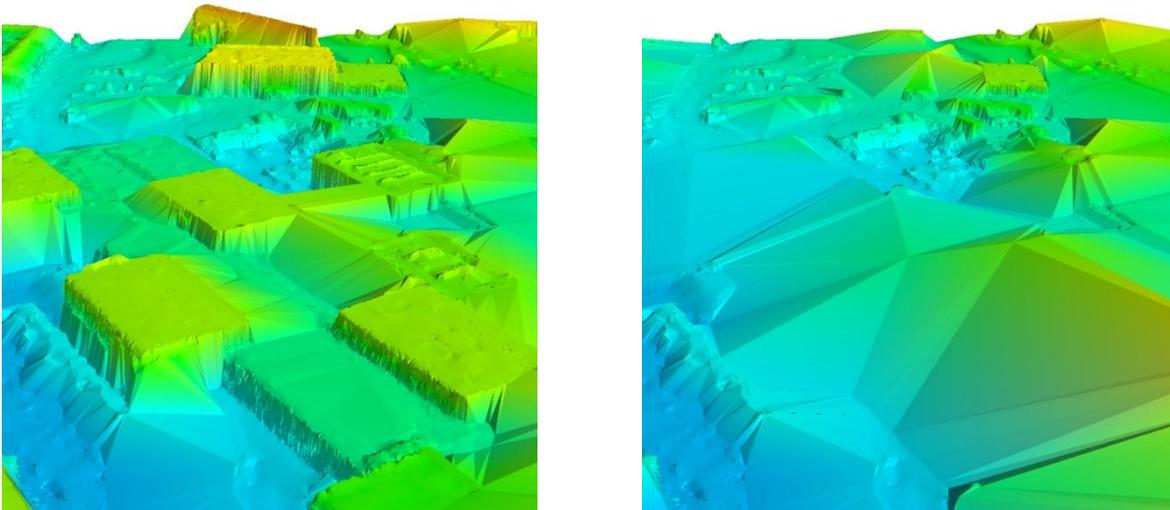
*Figure 112 – Plots before and after buildings are removed with the ray-casting algorithm*
