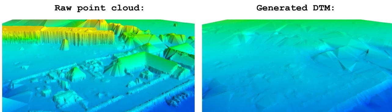
*Figure 100 – Points removed with the program DTM Creator 2.0*
