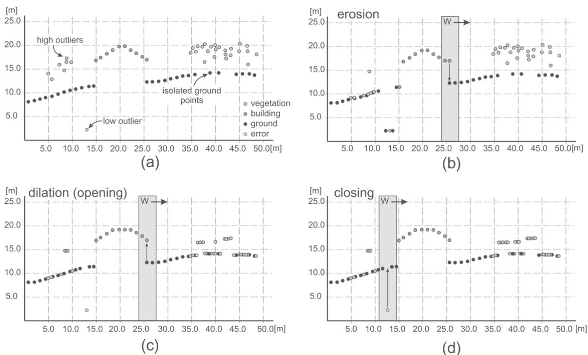
Figure 8 – “Cross section of LiDAR pointset (a), erosion of pointset (b), dilation of eroded pointset i.e. morphological opening (c), and morphological closing of opened pointset (d)” (Mongus og Zalík 2011, 3)
