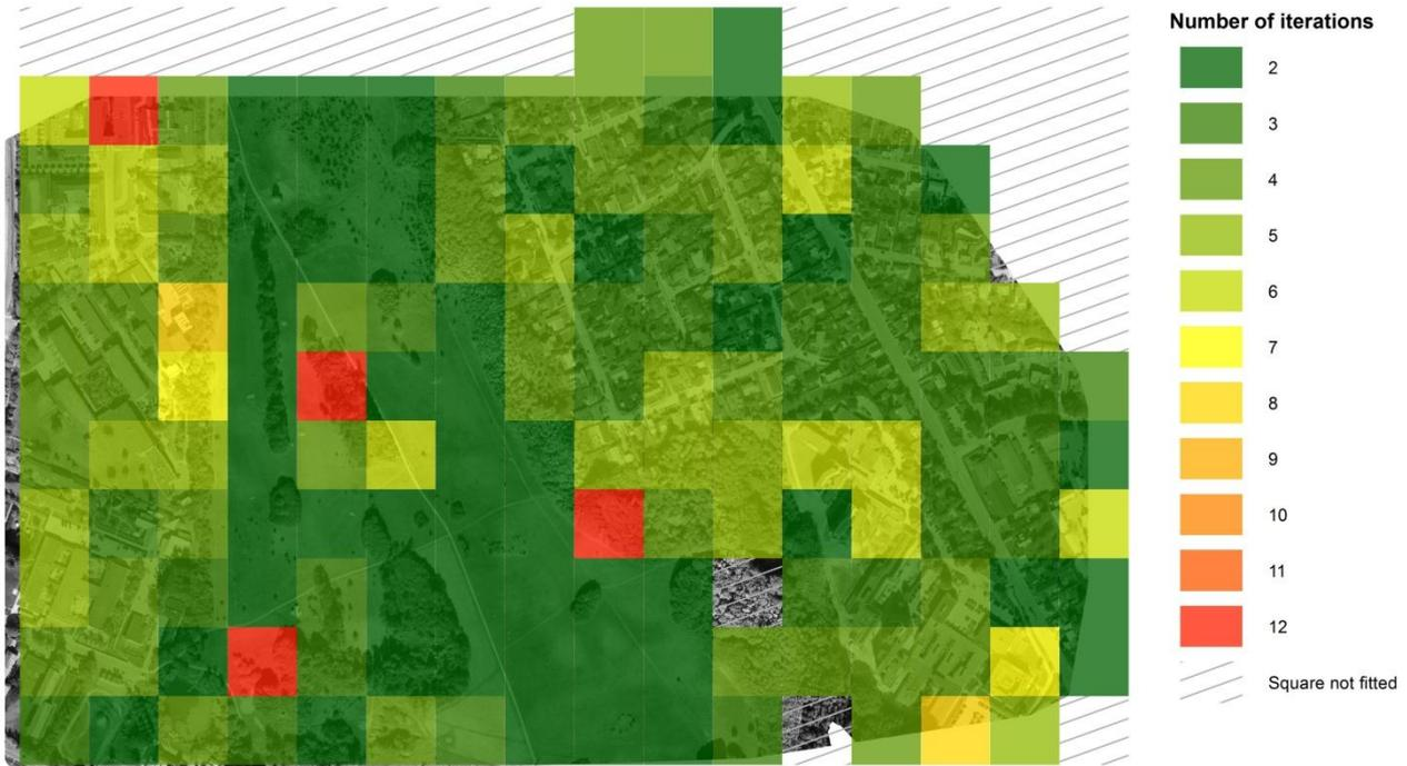
Figure 92 – Number of iterations in each square with the chosen polynomial order. Orthophoto can be seen behind.
