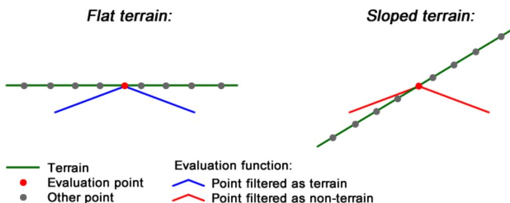
Figure 46 – The simple implementation of the slope-based filtering algorithm can lead to misleading results
