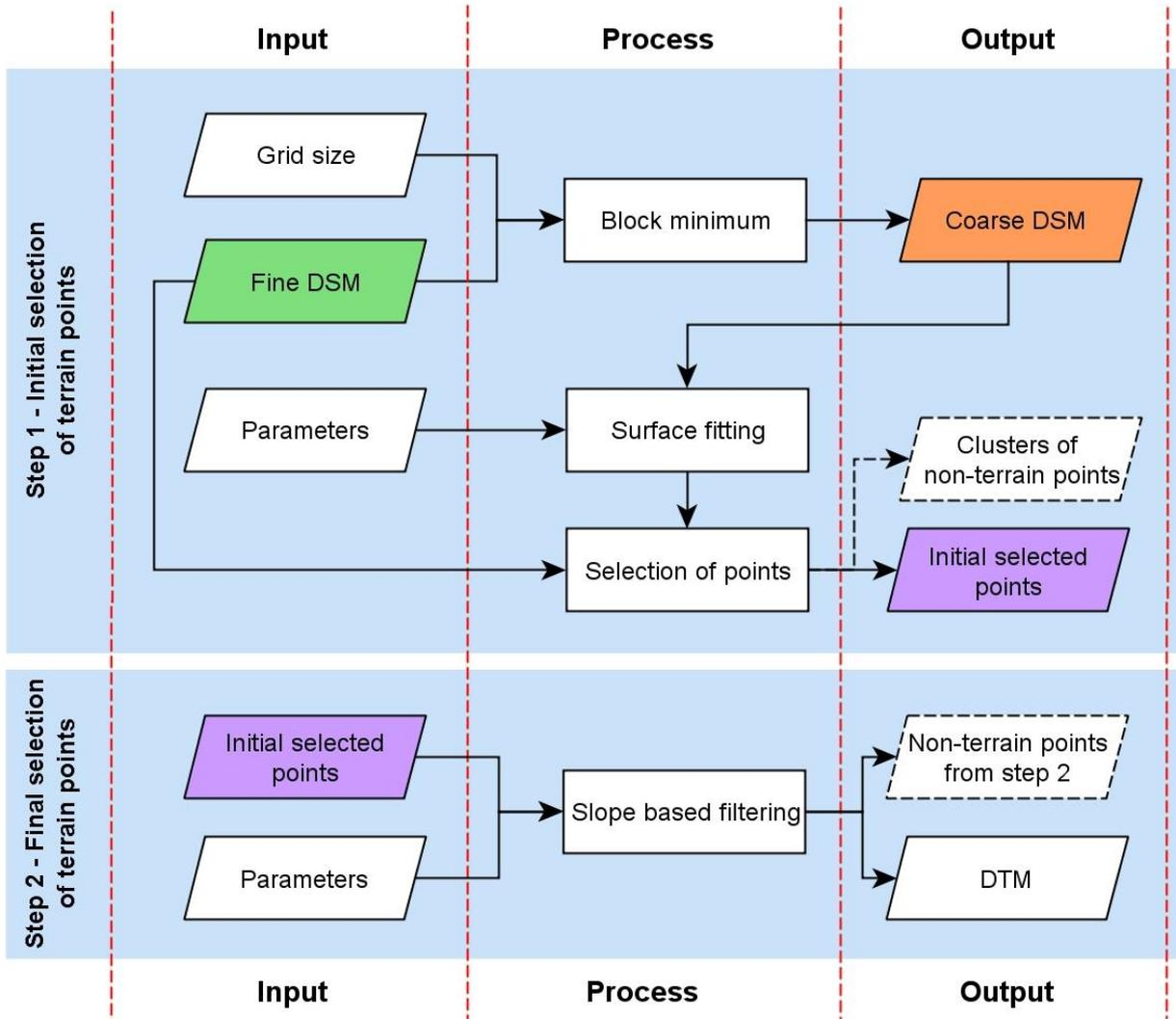
Figure 22 – Overall process for the filtering algorithm
