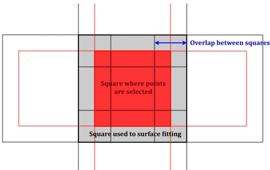
Figure 26 – The surface-based filtering works inside smaller overlapping squares. (Matthesen og Schmidt 2014, 105)
