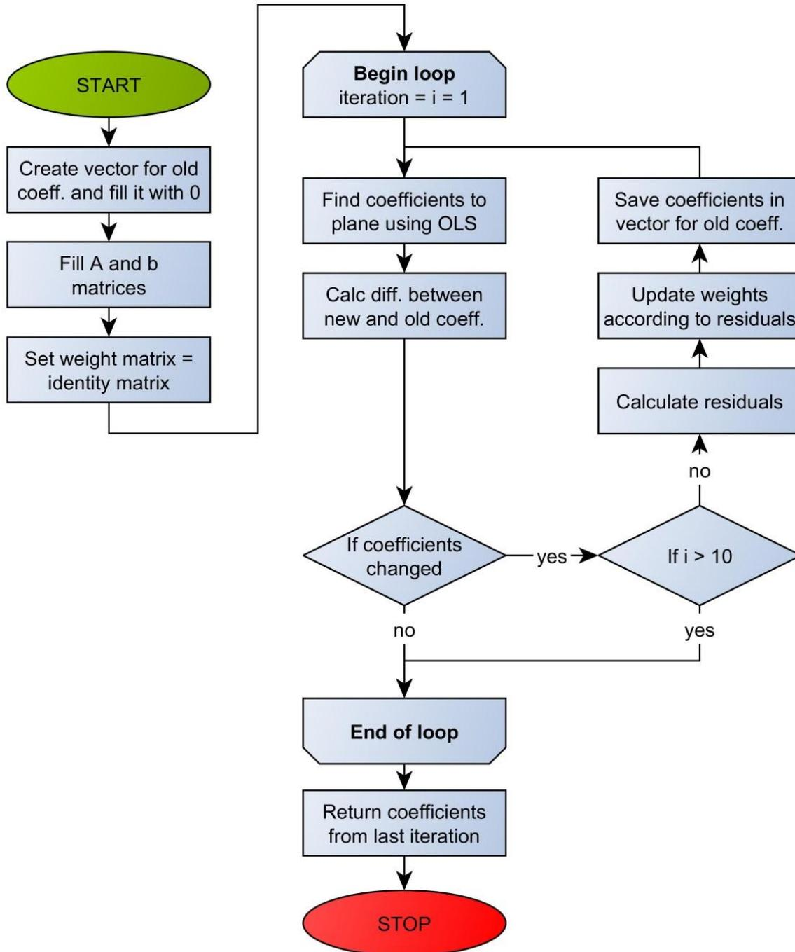
Figure 56 - Flow diagram showing the steps involved in robust fitting of a plane to a subset of the point cloud
