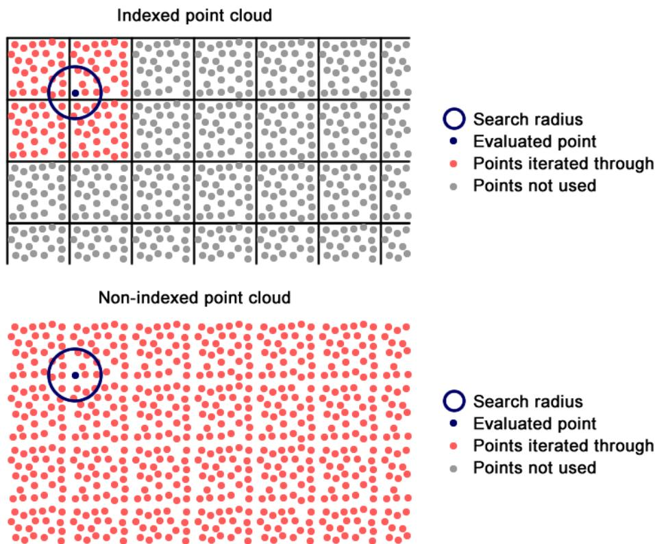
Figure 50 – Points used to find neighboring points within a given radius with and without indexing.
