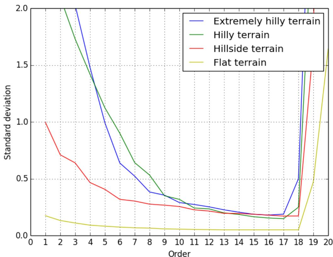
Figure 18 - The standard deviation of unit weight at different polynomial orders and with different terrain types (Matthesen og Schmidt 2014, 91)
