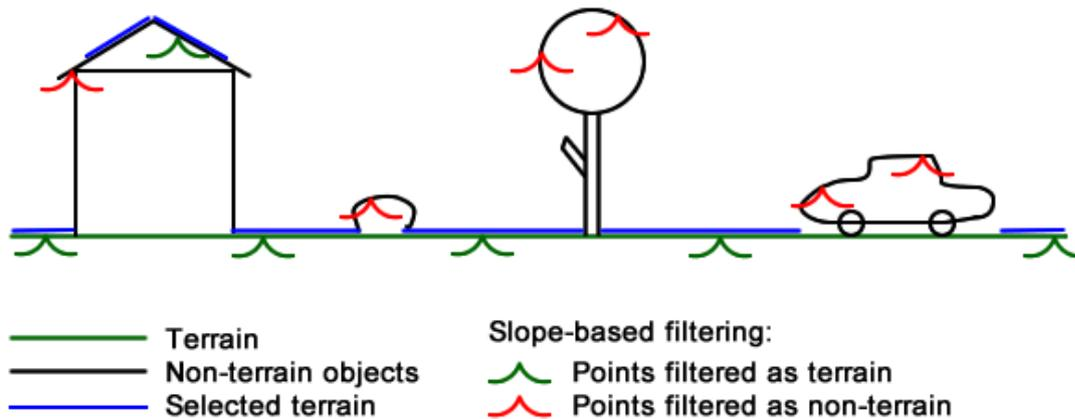
Figure 14 – Principle sketch of slope-based filtering
