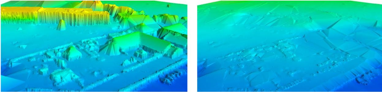
Figure 3 – Point cloud before and after filtering. (Matthesen og Schmidt 2014, 155)
