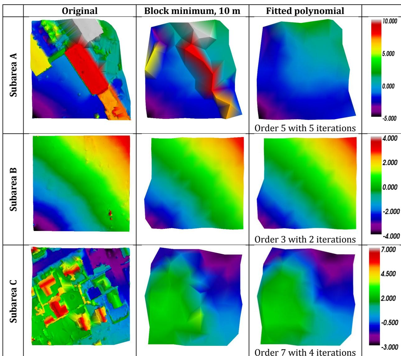
Figure 43 - Selected polynomial order in comparison with the original point cloud and the block minimum point cloud
