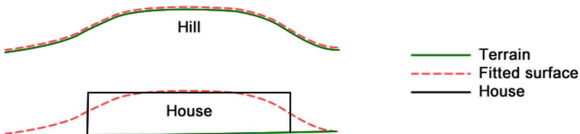
Figure 15 – The algorithm cannot differentiate between a hill and a large low-rise building.
