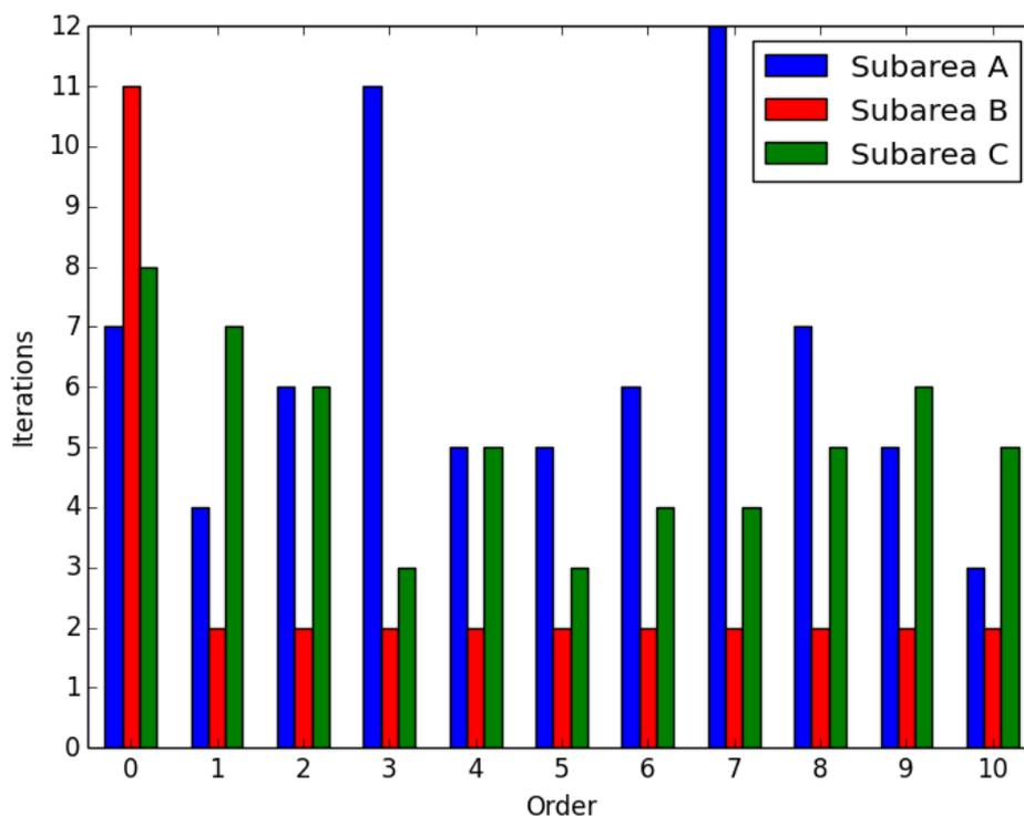
Figure 37 – Maximum iterations used to fit different orders of polynomials to the subareas when the iteration stop criterion is 1%
