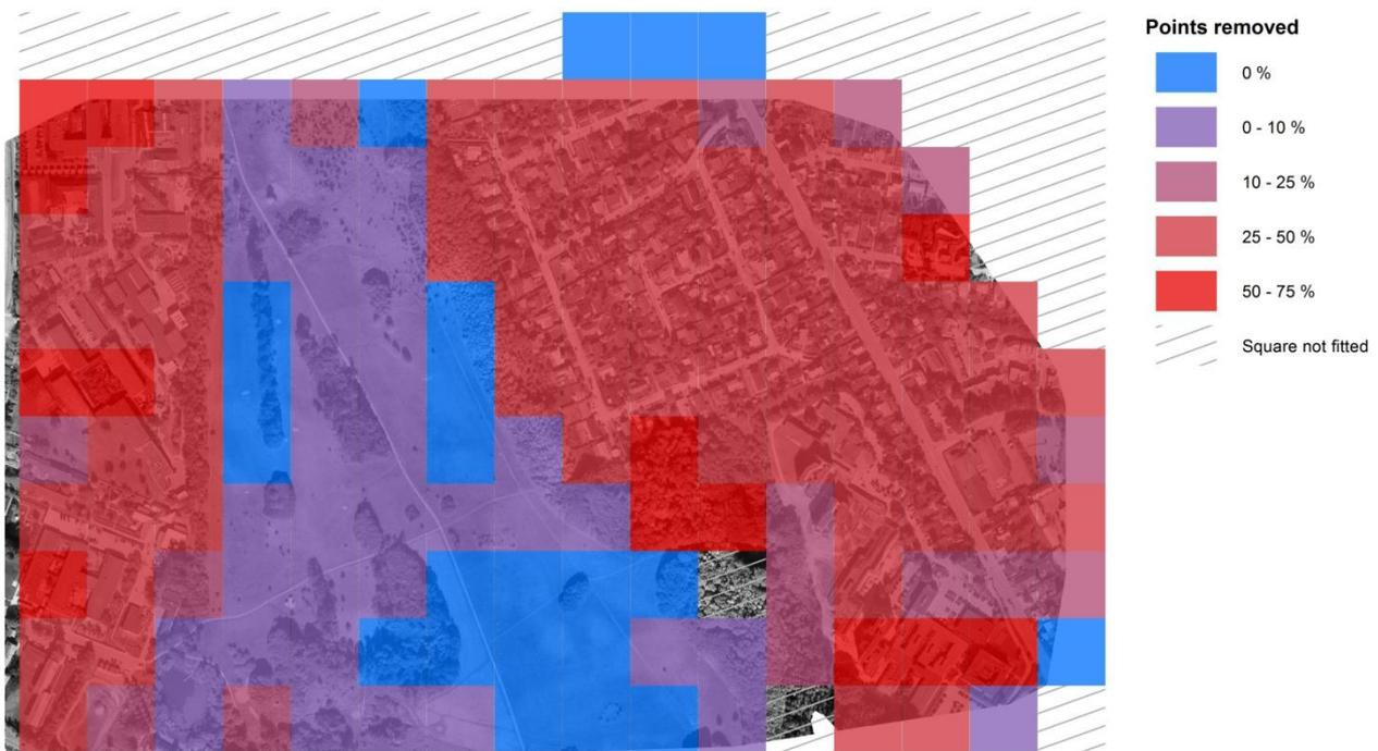
Figure 93 – Removed points as percent of the original number of points in each square. Orthophoto can be seen behind.
