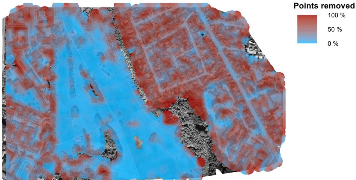
Figure 99 – Removed points in step 2. Orthophoto can be seen behind.
