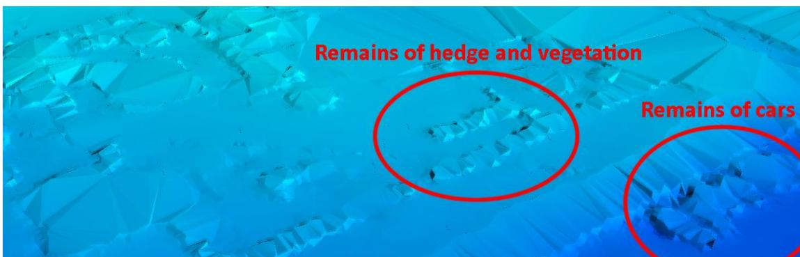
Figure 4 - Remains of non-terrain points because of buffer
