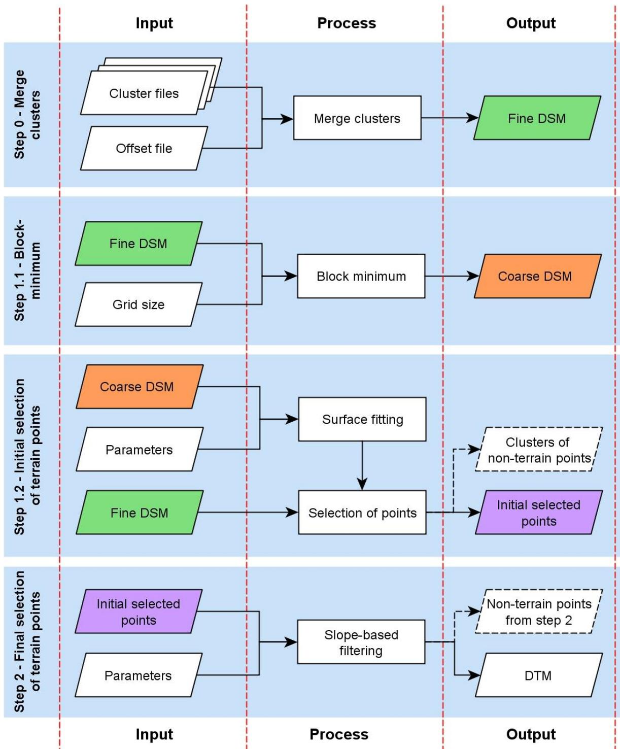
Figure 72 - Steps in the final program. The relations between input/output files from the different steps are marked with colors. For simplicity, the generated documentation files are not showed.
