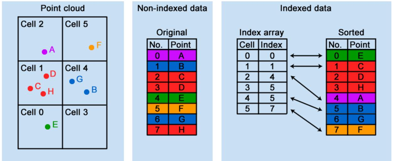
Figure 51 – Illustration of the used implementation of grid-based indexing
