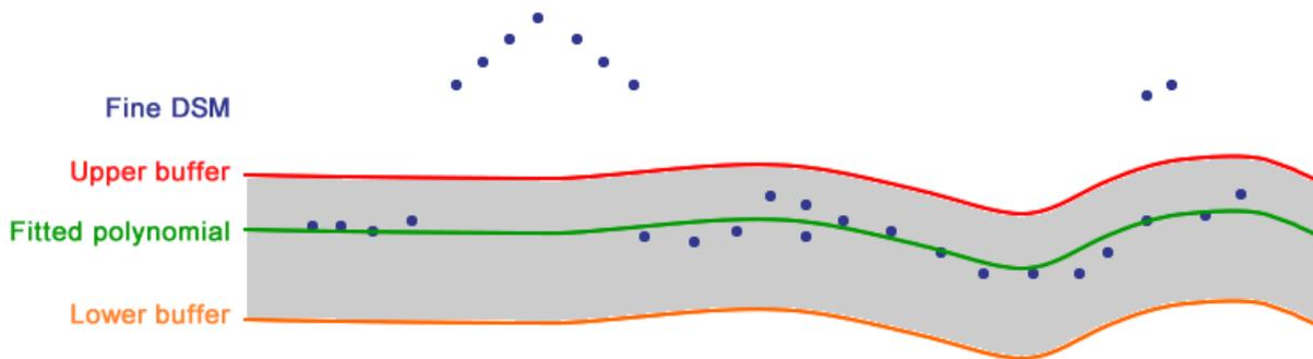
Figure 44 – Illustration of the buffer principle, with an upper buffer above the surface and a lower buffer below the surface
