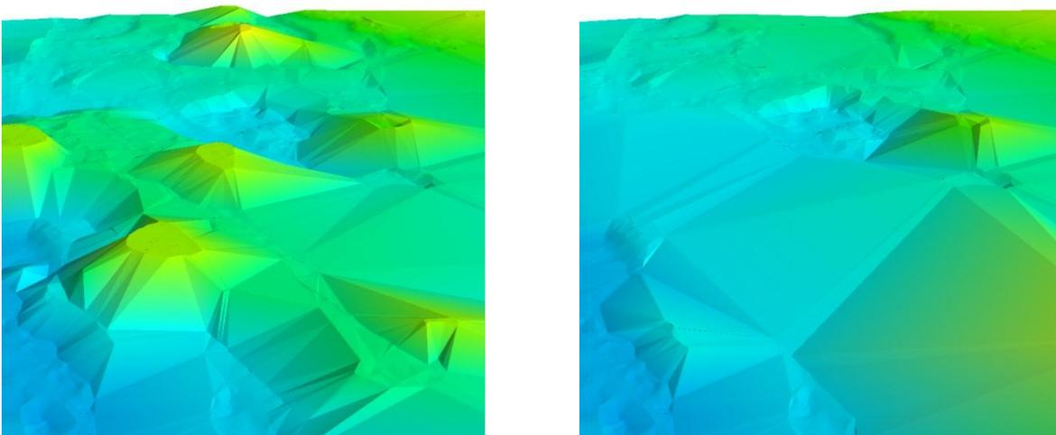
*Figure 113 – Plots before and after buildings are removed with the ray-casting algorithm*
