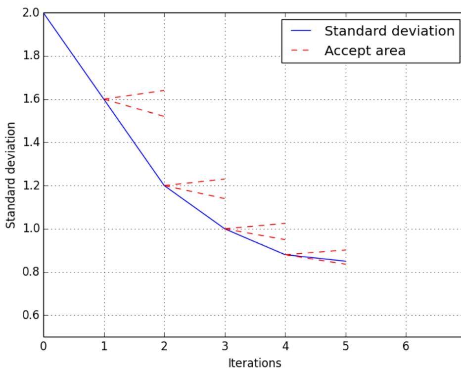
Figure 39 – Illustration of the chosen stop criterion. It can be seen that the accept area decrease when the standard deviation decrease.
