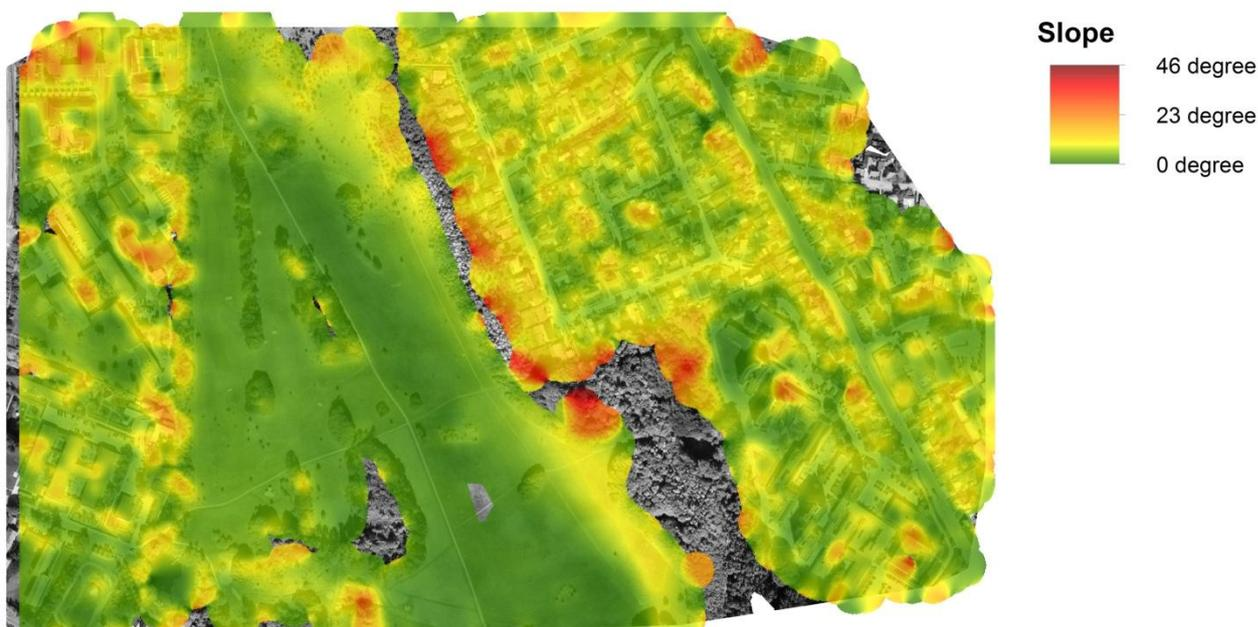
Figure 98 – Terrain slope according to the slope correction in step 2. Orthophoto can be seen behind.
