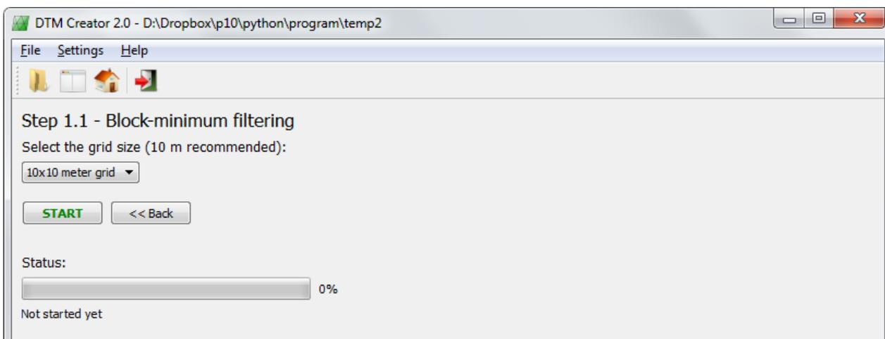
Figure 78 – In Step 1.1 a block-minimum filter is applied to the raw point cloud from Step 0
