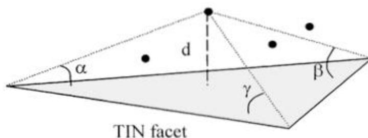
Figure 10 – Illustration of a point's angles to the nodes and the distance to the TIN facet plane (Axelsson 2000, 3)
