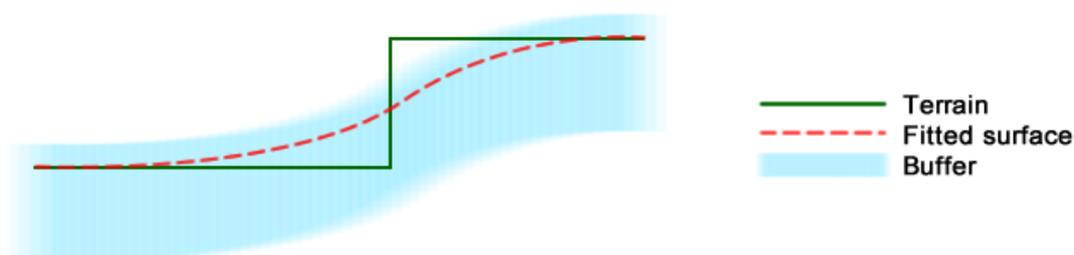
Figure 21 – Surface-based filtering will cut the upper edge.
