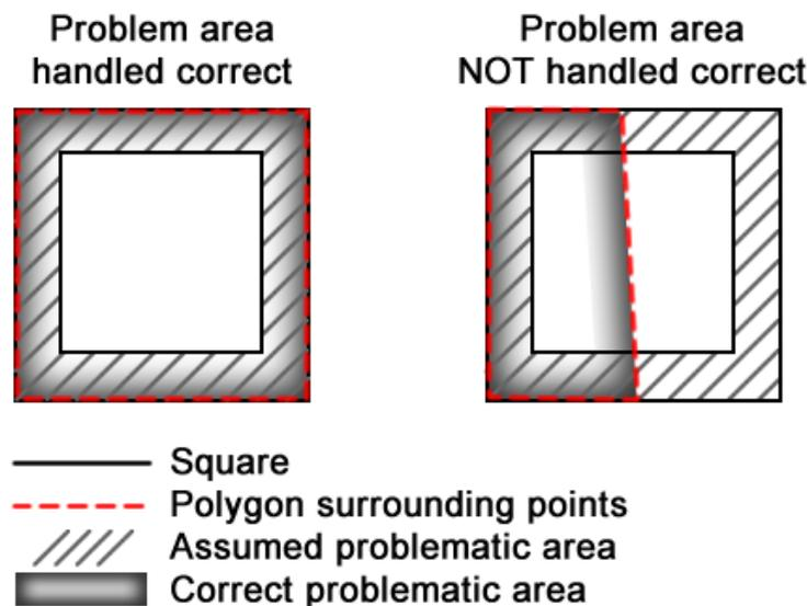
Figure 19 – Problematic areas are not handled correct in the previous algorithm, if the points are not equally distributed in the square.
