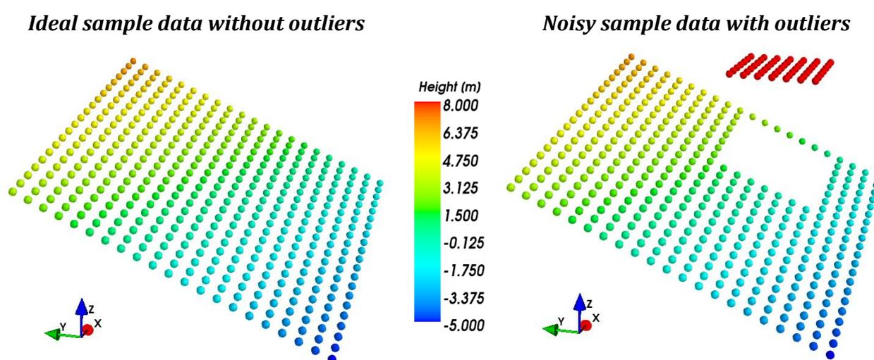
Figure 57 – Generated sample data used for testing of the robust plane fitting algorithm
