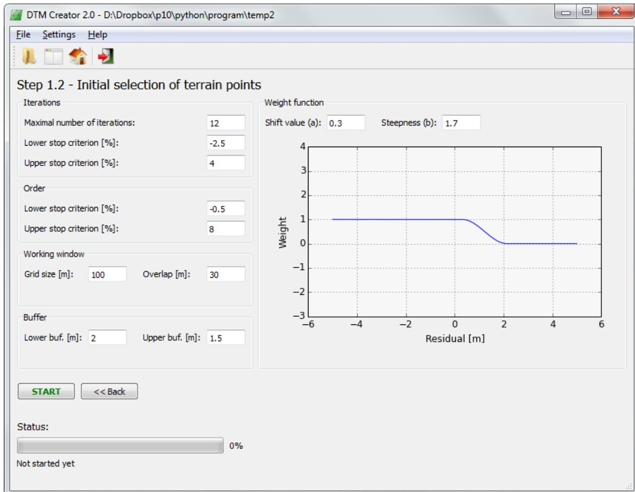
Figure 80 – In Step 1.2 an initial selection of terrain points is performed
