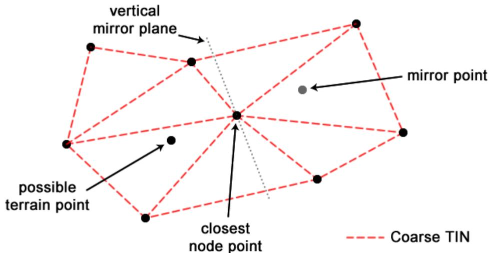
Figure 12 - Creation of mirror point seen from a top view
