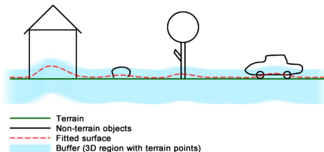
Figure 13 – Principle sketch of surface based filtering
