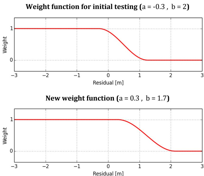
Figure 35 – Initial and new weight function
