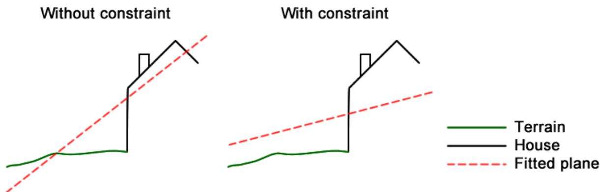
Figure 20 – Example of a plane fitted to a house placed on the boundary of the working area/square
