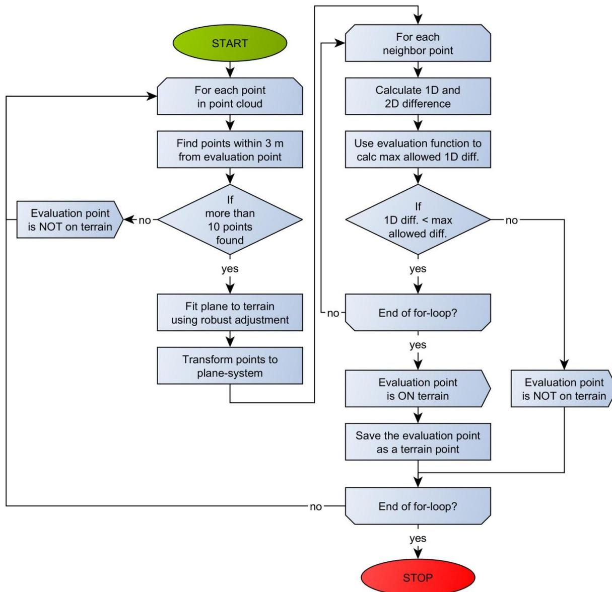
Figure 49 – Flowchart showing the overall structure for the slope-based filtering algorithm
