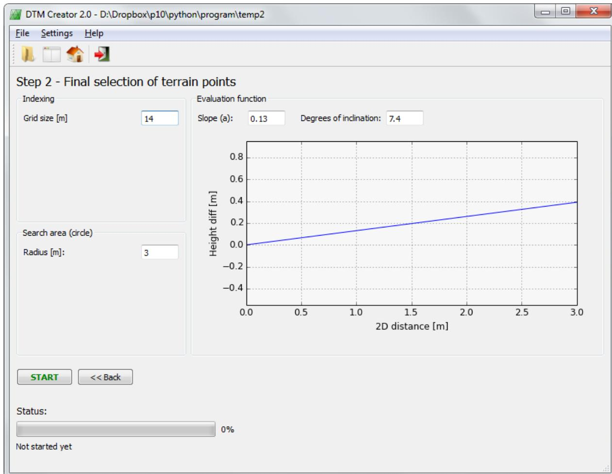
Figure 82 – In Step 2 the final DTM is created using slope-based filtering
