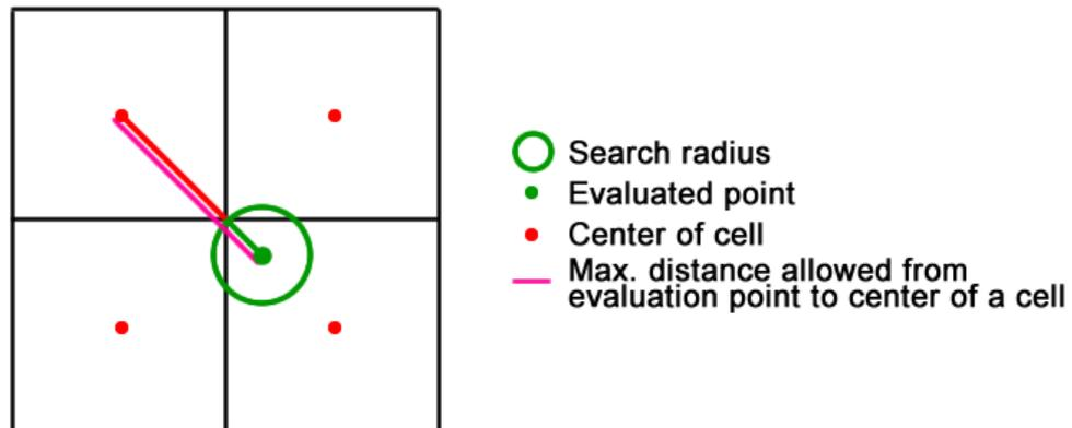
Figure 52 - Max distance used to find the correct cells when searching for points within a given search radius
