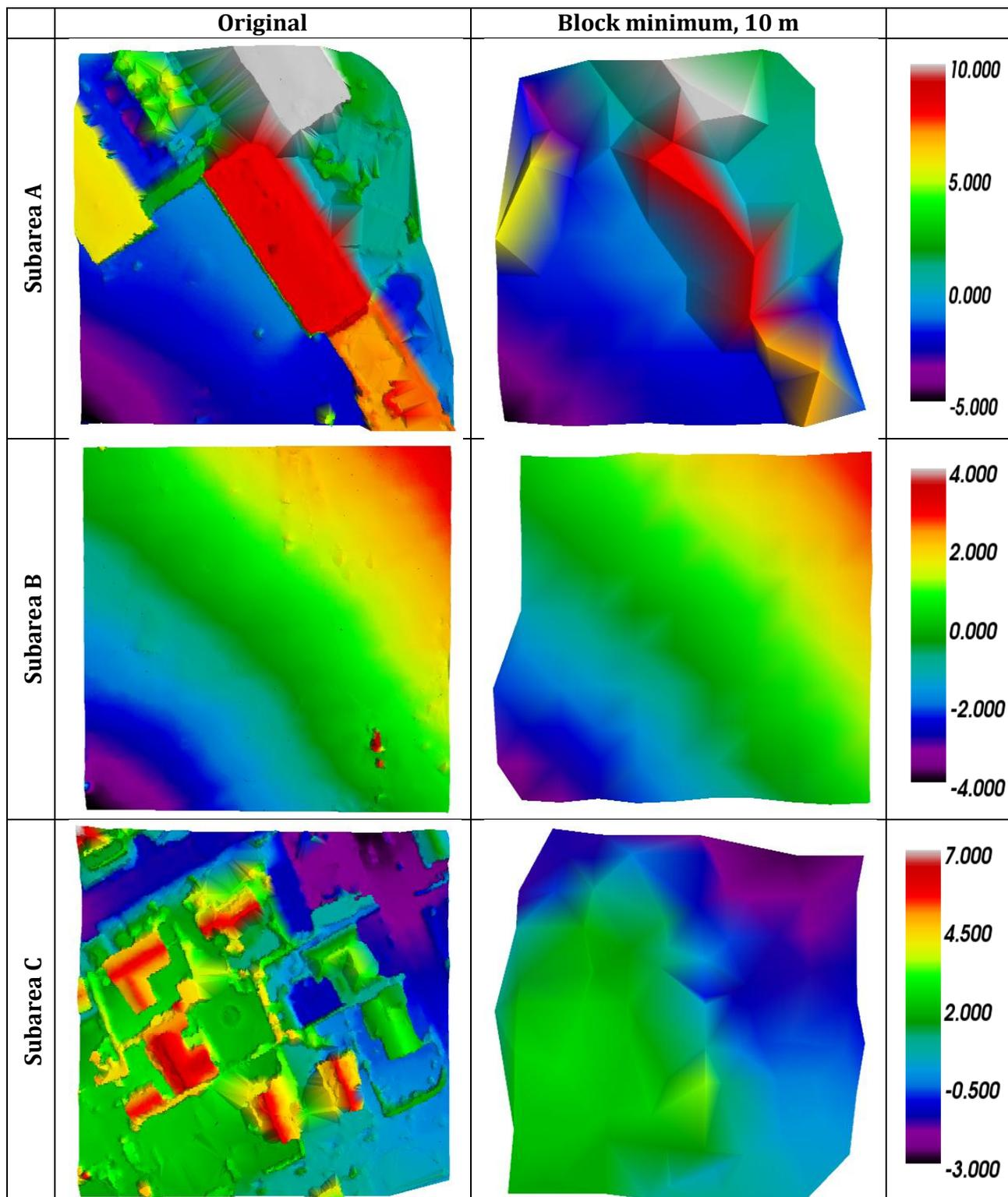
Figure 29 – Point cloud before and after applying the block-minimum filter
