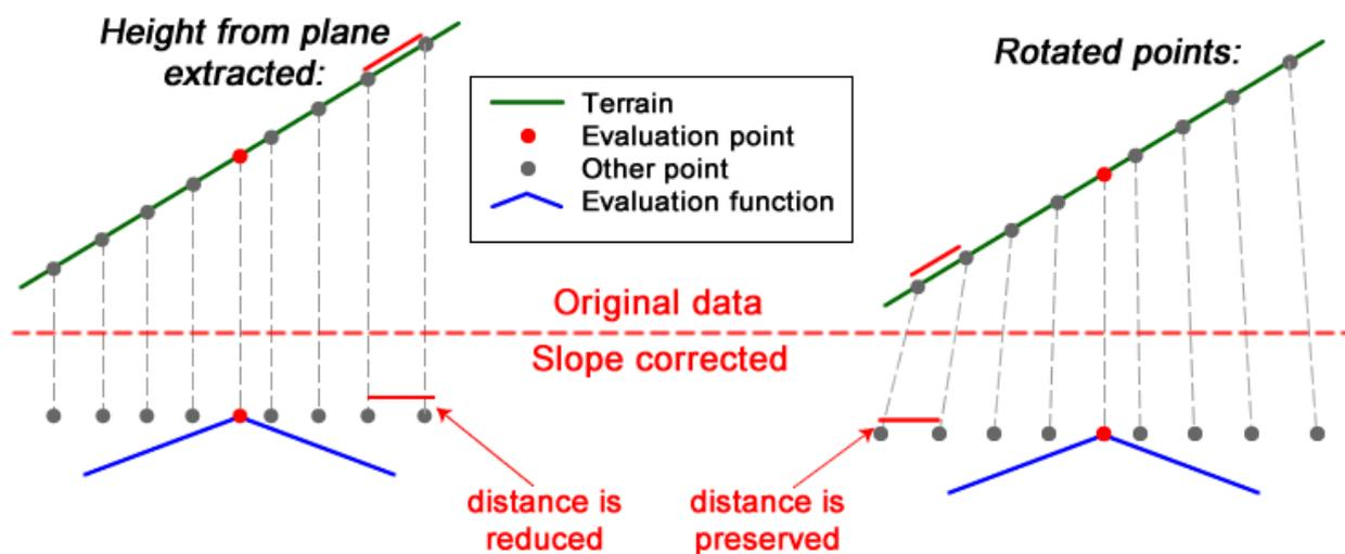
Figure 60 – Illustration of the different suggested methods for slope-correction.
