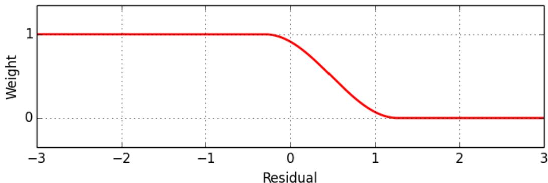
Figure 2 - One of the weight functions used in the iterative surface fitting (Matthesen og Schmidt 2014, 95)
