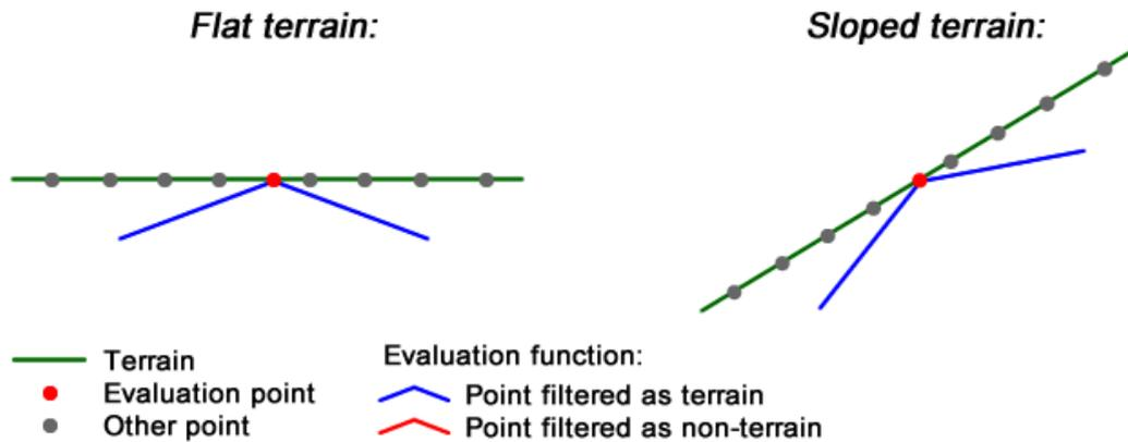
Figure 47 – For the best results, the evaluation function should be adjusted according to the mean slope
