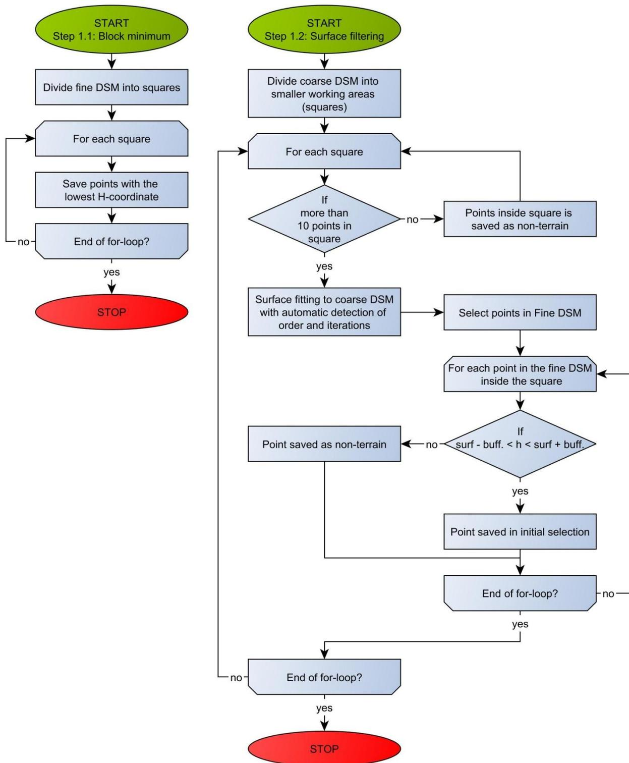
Figure 27 – Flowchart for the overall structure in step 1
