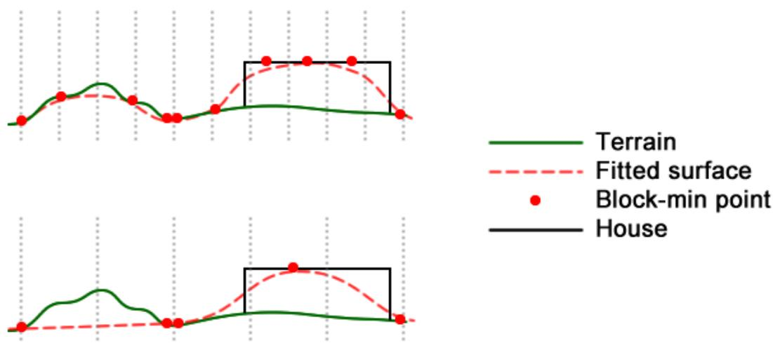
Figure 17 – A block-minimum filter with a large grid size results in fewer points on the problematic buildings, but might happen at the cost of removing valid terrain.
