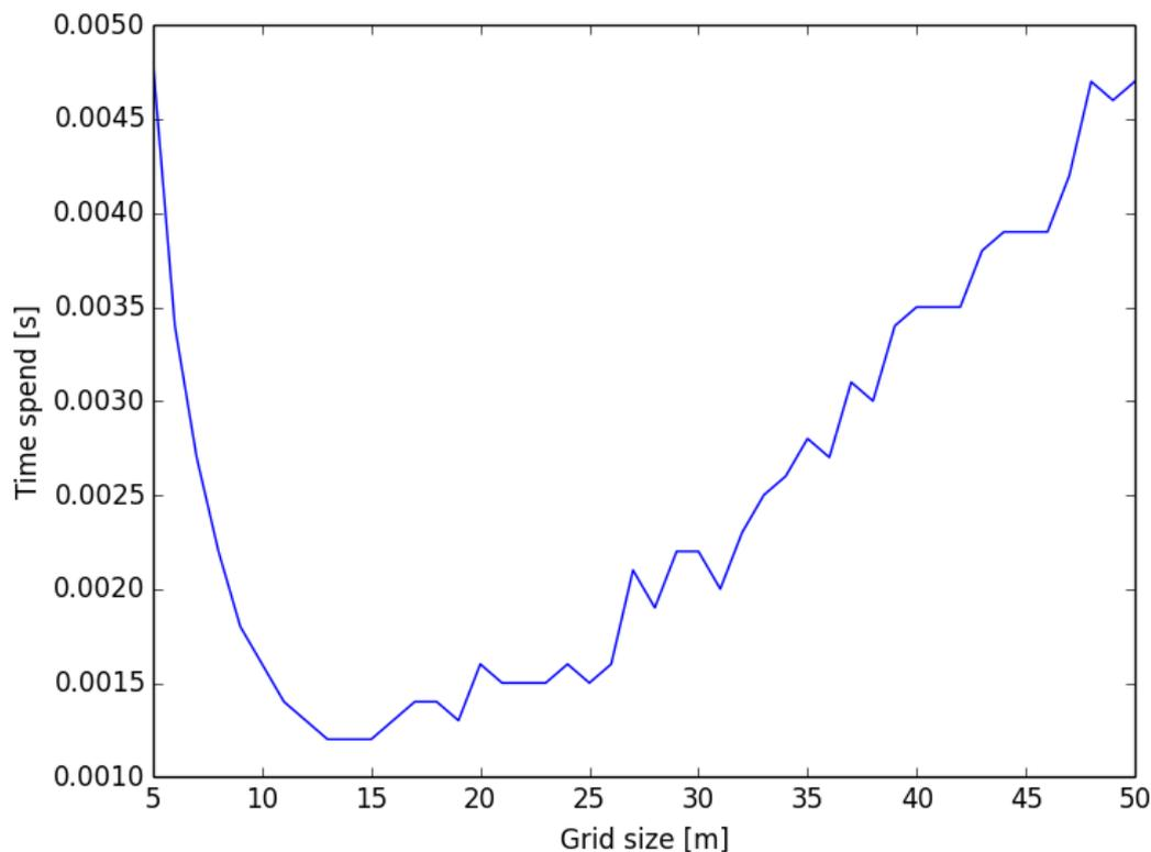
Figure 53 – For different grid sizes, the graph show the time spend to find the points inside a search radius of 3 meters from a random evaluation point inside Subarea B.
