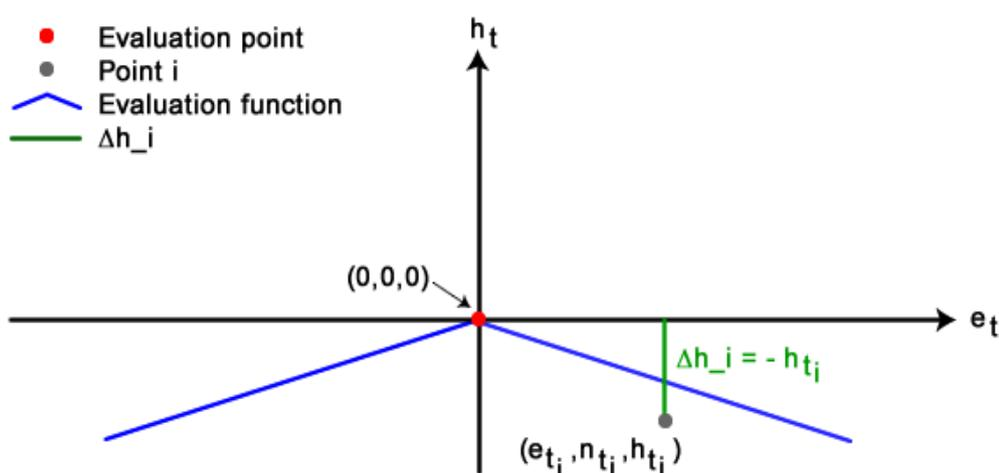
Figure 67 – Illustration of the evaluation function and the actual height difference. In this case the evaluation point is classified as non-terrain.
