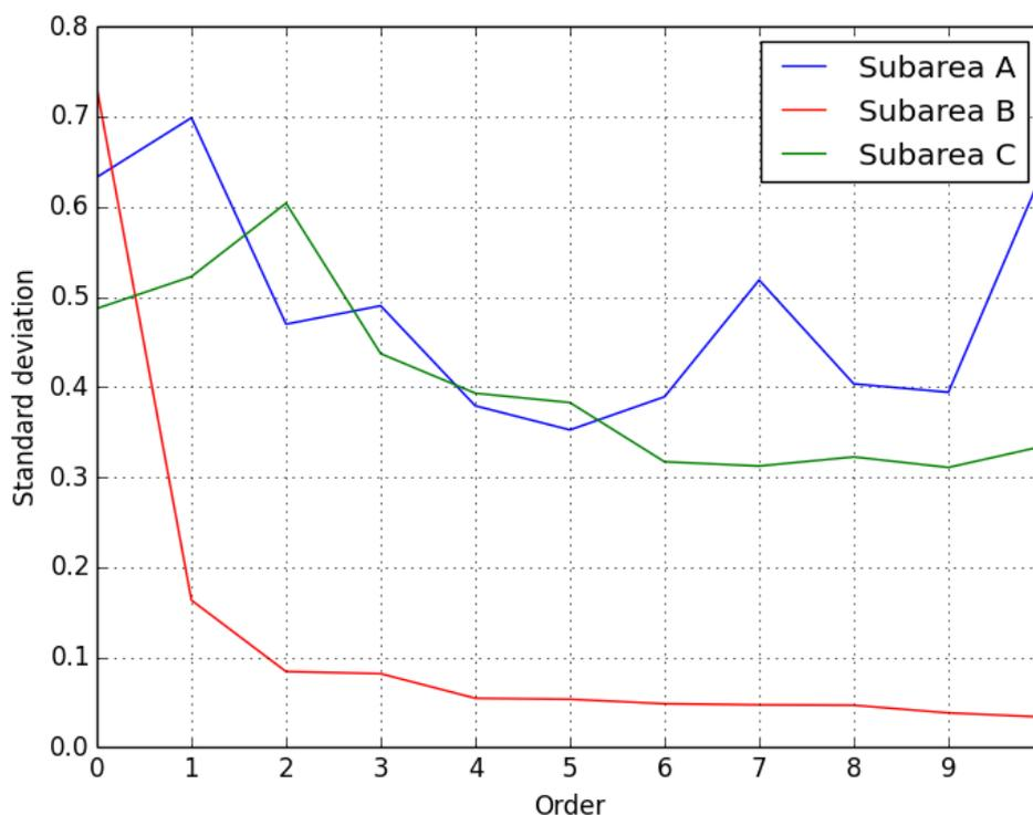
Figure 36 - Standard deviation for each order in the subareas (the number of iterations for each order is decided according to the stop criterion, of 6%, used in the initial testing)
