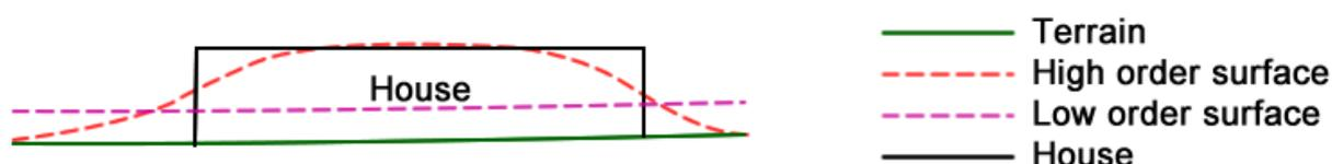
Figure 16 – A low order surface polynomial makes it easier to remove points on large low-rise buildings, because it is less flexible.
