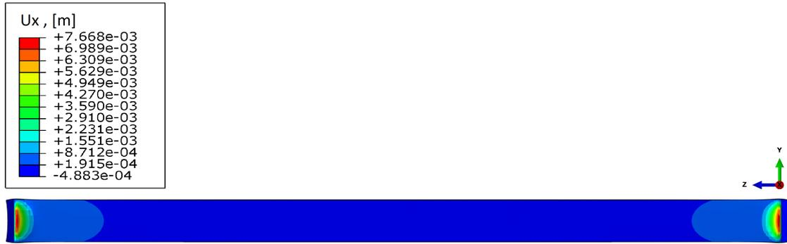
**Figure 5.11.** The deformed column with an initial out-of-square imperfection.
