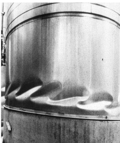
*Figure 1.1:* Example of local buckling of a wine tank [Bushnell, 1981]
