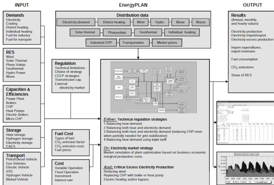
Figure 60: Input output structure of the EnergyPLAN model
