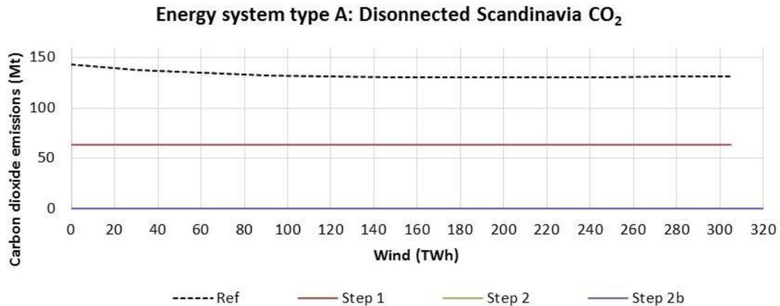
Figure 40: CO<sub>2</sub>-emissions for steps in energy system type A in Disconnected Scandinavian system
