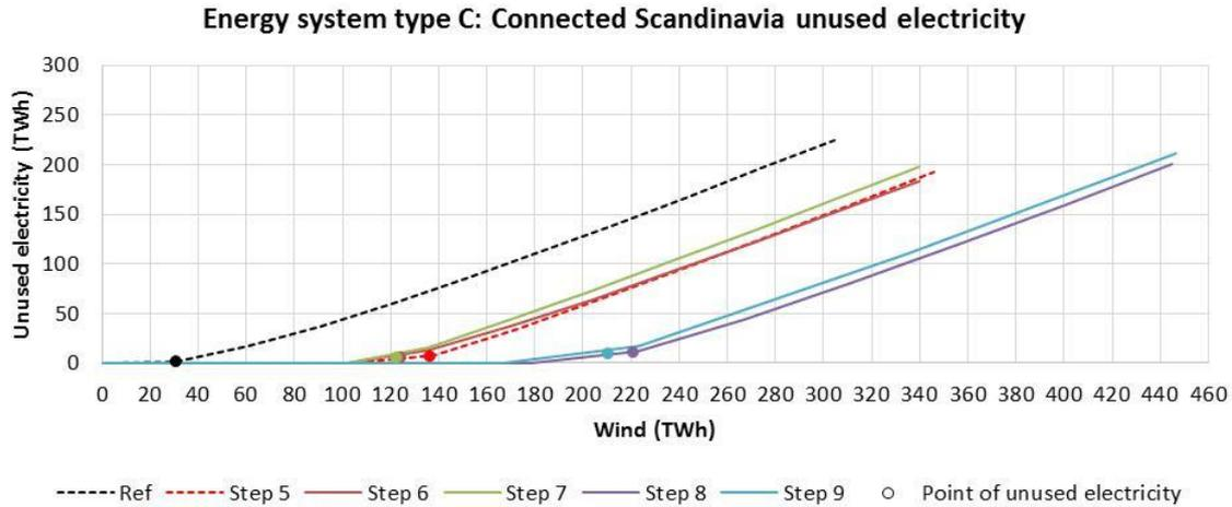
Figure 49: Wind integration for steps in energy system type C in Connected Scandinavian system
