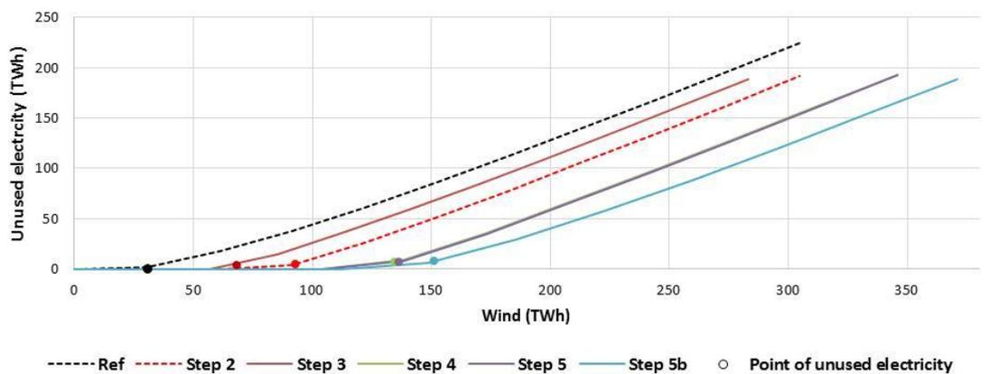
Figure 43: Wind integration for steps in energy system type B in Connected Scandinavian system
