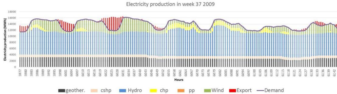
Figure 26: Electricity production distribution in a week in the Swedish reference energy system
