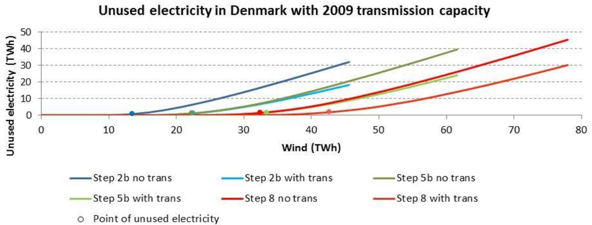
Figure 56: Sensitivity of installing transmission capacity as of 2009 in Denmark
