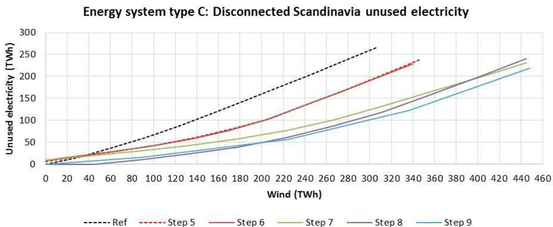
Figure 48: Wind integration for steps in energy system type C in Disconnected Scandinavian system
