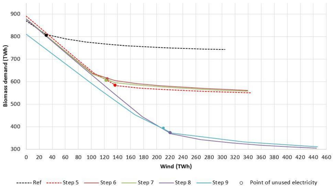
Figure 51: Biomass demand for steps in energy system type C in Connected Scandinavian system
