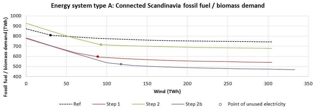
Figure 37: Fossil fuel and biomass demand for steps in energy system type A in Connected Scandinavian system
