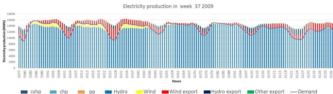
Figure 27: Electricity production distribution in a week in the Norwegian reference energy system
