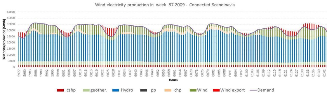
Figure 31: Electricity production distribution in a week in the Connected Scandinavian reference energy system
