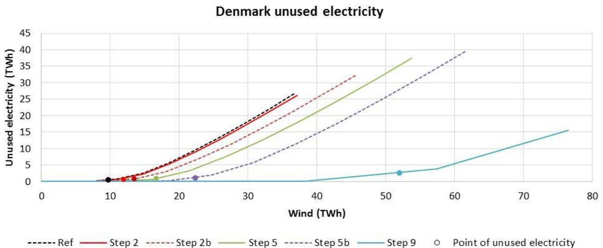
Figure 8: Unused electricity curves for Denmark for selected steps with integration of wind from 0-100% of electricity demand
