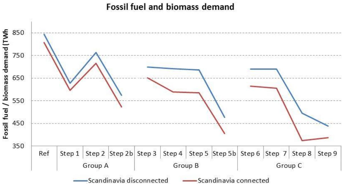
Figure 4: Fossil fuel and biomass demand for the Connected and Disconnected Scandinavian energy systems
