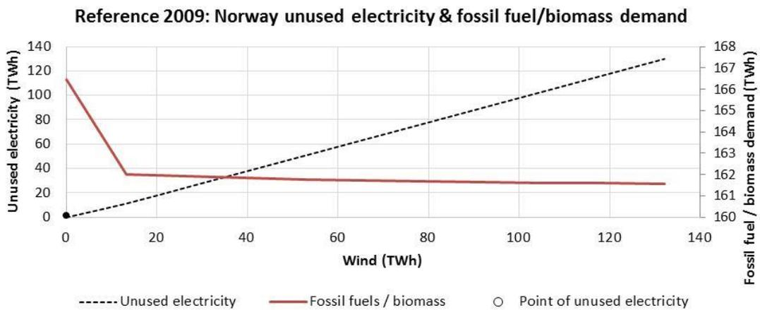
Figure 23: The unused electricity production and fossil fuel and biomass demand in the Norwegian reference system
