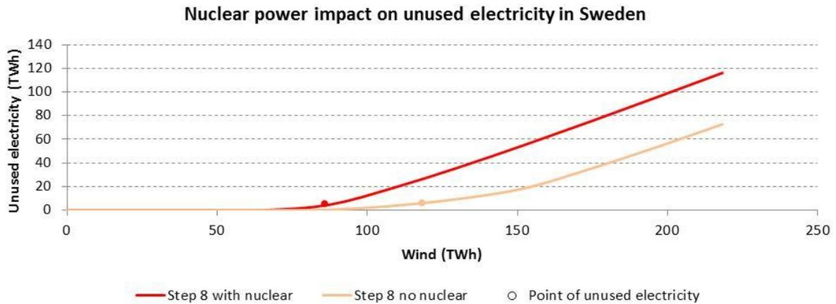
Figure 57: Sensitivity of removing nuclear power in the Swedish energy system
