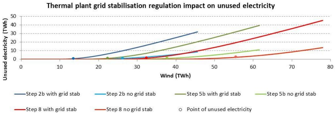
Figure 55: Sensitivity of thermal plant regulation on unused electricity in the Danish energy system
