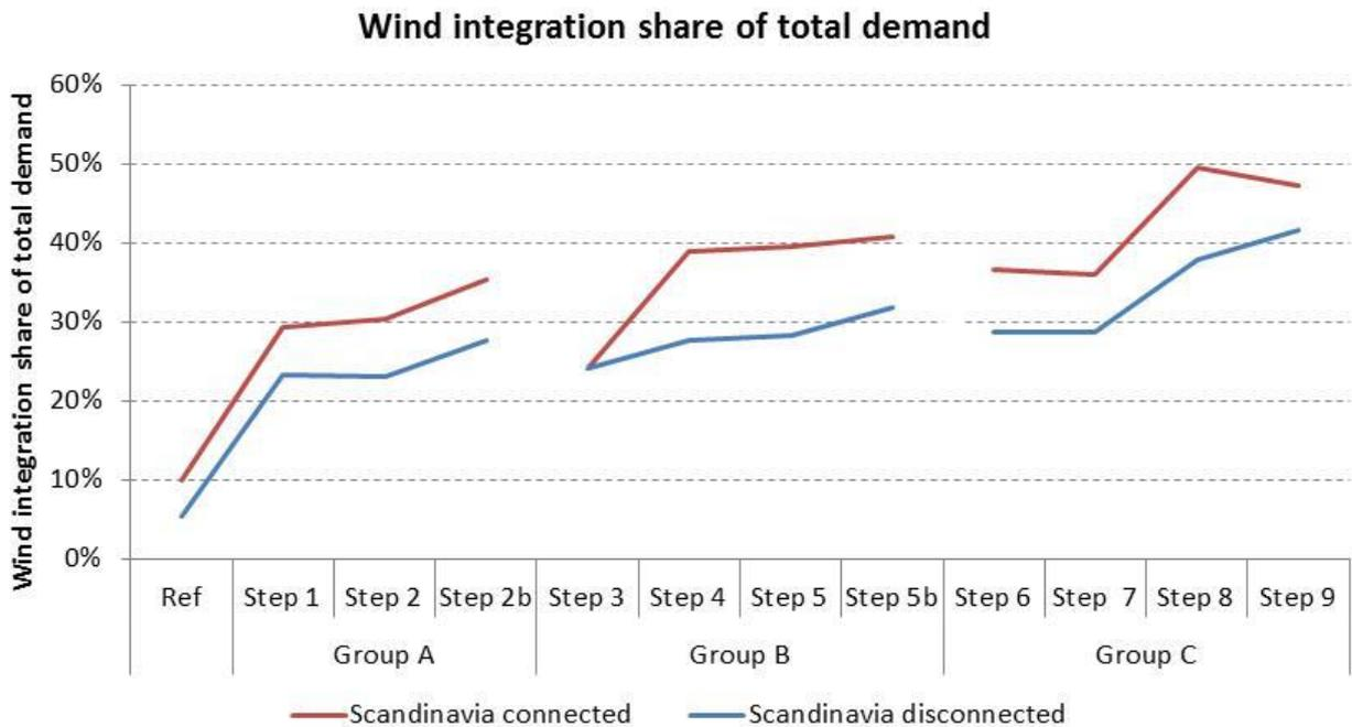
Figure 2: Wind integration share of total demand for the Connected and Disconnected Scandinavian energy systems
