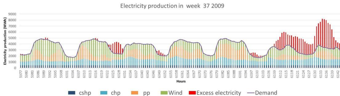
Figure 25: Electricity production distribution in a week in the Danish reference energy system
