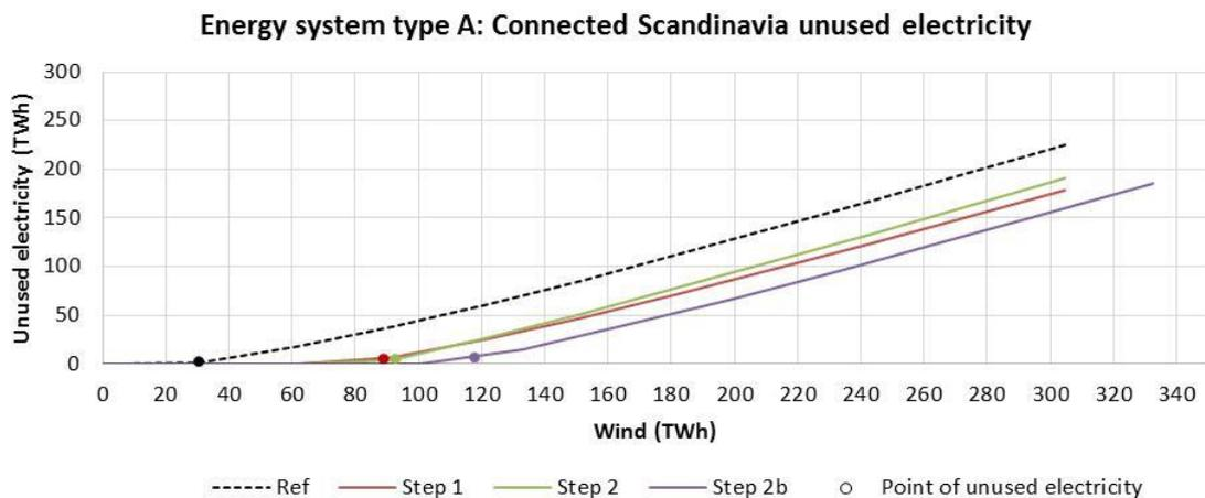
Figure 35: Wind integration for steps in energy system type A in Connected Scandinavian system
