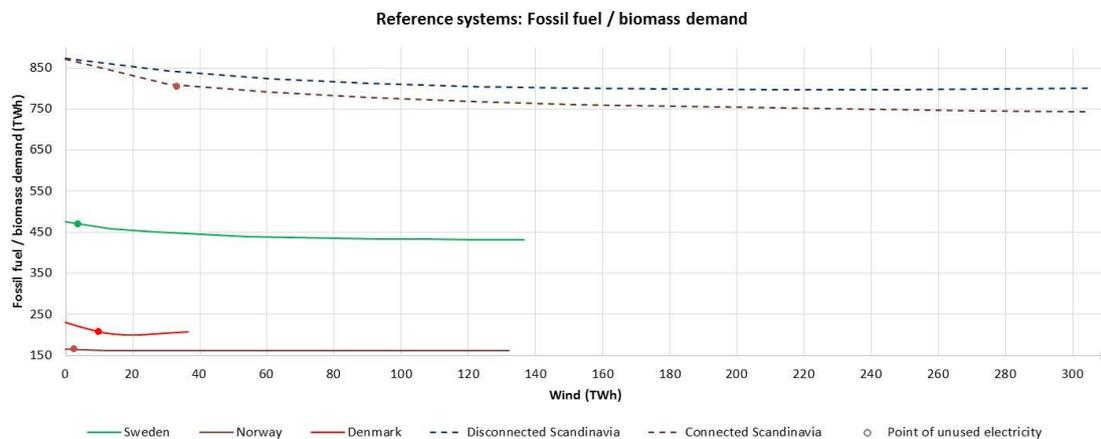
Figure 29: The fossil fuel and biomass demand for Denmark, Sweden, Norway, Disconnected and Connected Scandinavia
