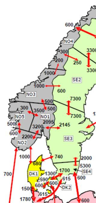
Figure 14: Transmission capacity between Denmark, Sweden and Norway (Nord Pool 2014)
