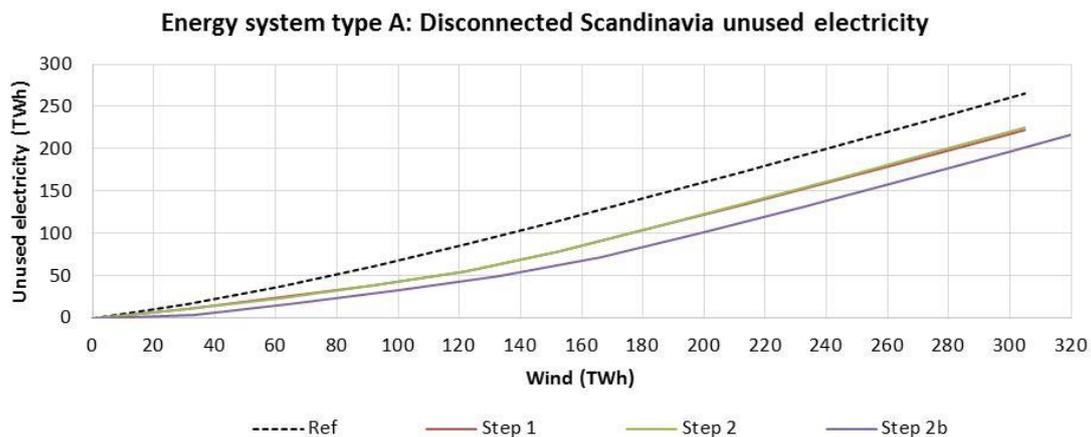
Figure 34: Wind integration for steps in energy system type A in Disconnected Scandinavian system
