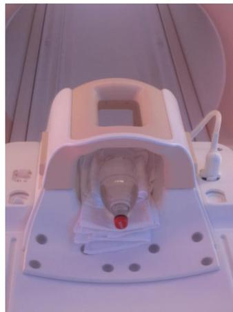
Picture 2: Placement of the phantom within the coil.
