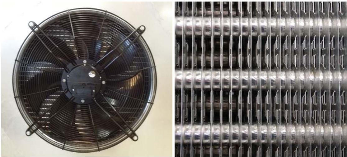
Figure 3.2. Left: The evaporator with the fan. Right: The louvered fin-and-tube configuration.
