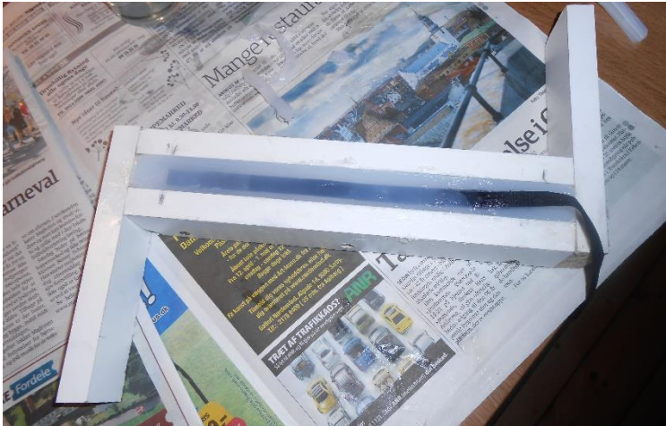
Figure 6.6. The casting mould filled with silicone and a sensor.
