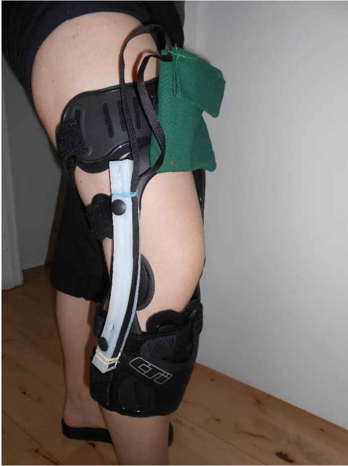
Figure 6.9. The final prototype where the sensor is placed on top of the silicone block.
