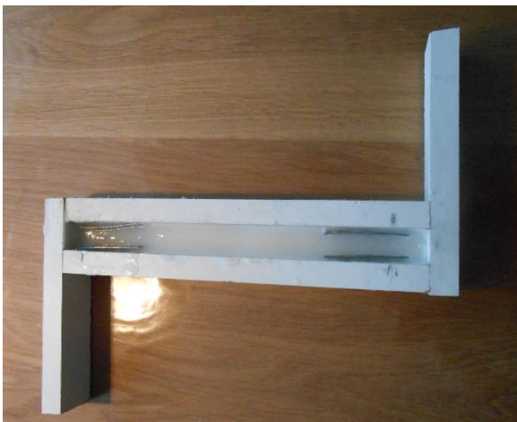
Figure 6.7. The iron plates were placed in the end of the silicon block.
