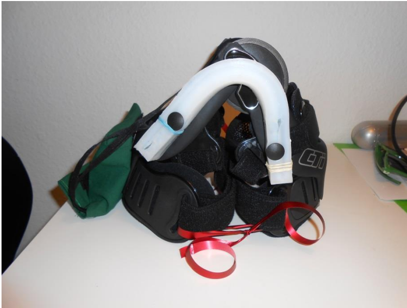
Figure 6.13. Shows how the sensor is stretched when the brace was fixed in position of maximum flexion.
