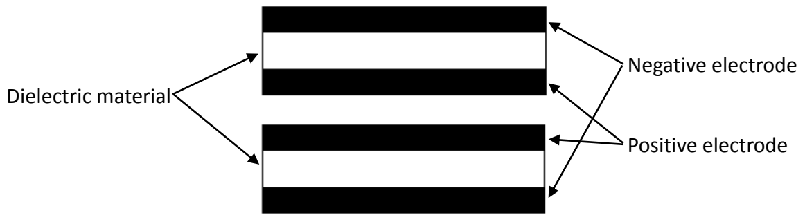
Figure 3.4. Shows how the charge of the electrodes lies around the dielectric material.
