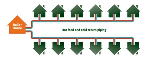
FIGURE 2: DIAGRAM OF DISTRICT HEATING NETWORK (SUSTAINABLE WOOD ENERGY, N.D.)
