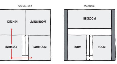
Fig. 36 The straight staircase causing the semi-heated space to be used as internal flow area
