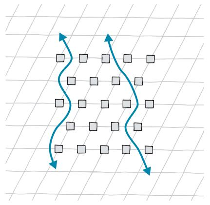
Fig. 30 Principle for weaving the traffic roads in between the buildings
