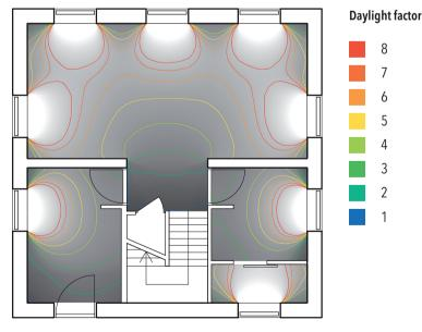
Fig. 51 Daylight factor on the ground floor
