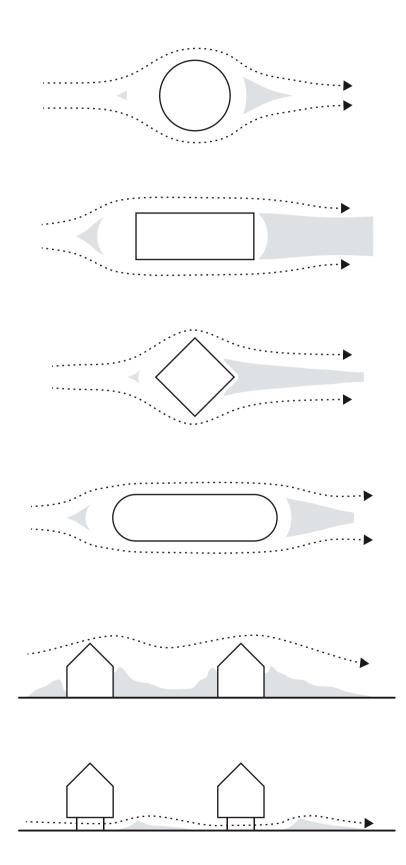
Fig. 7 Snow drifting around buildings
