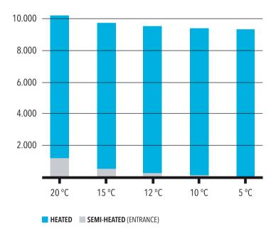
Fig. 47 Annual energy use for heating (Heating, fan power and heat coil)
