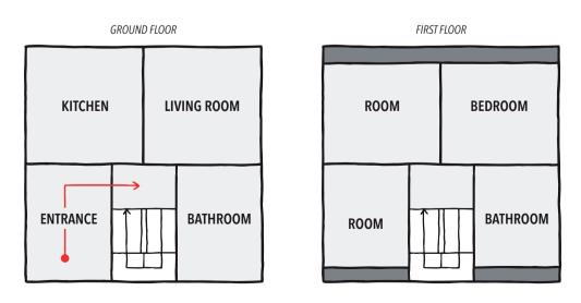
Fig. 37 The staircase with landing has a small distribution area that eliminates the entrance as flow area
