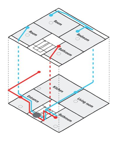
Fig. 44 Ventilation unit placed beneath staircase
