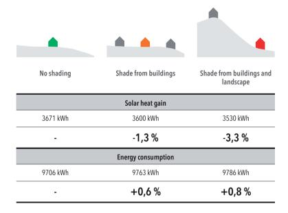
The result from these studies shows that the context does not have a significant impact on the energy use. The worst placement of a house, in relation to solar radiation, causes a 0,8 % increase in energy consumption in comparison to a house with no shading at all. The reason for the relatively small loss of energy might be that there is small amount of glazing facing the shaded areas and that there is not much heat to capture from the sun anyway at the time of day when the building is in shade.
