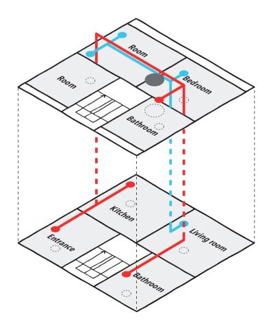
Fig. 45 Ventilation unit placed in entrance
