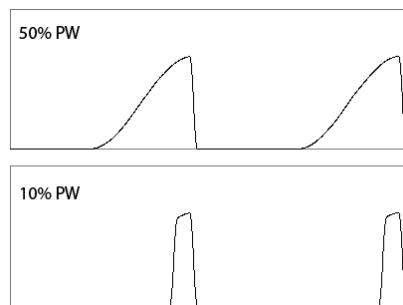
**Figure 23 The influence of pulse width on the duration and envelope of the haptic event**
