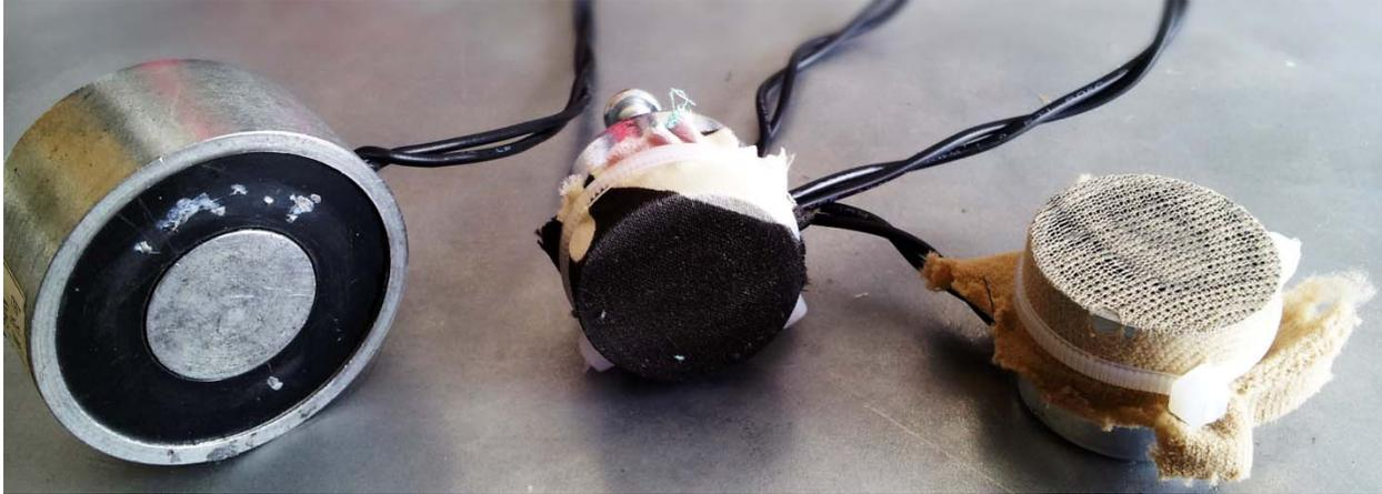
Figure 6 Large magnet (left) and two smaller magnets with fabric covering.
