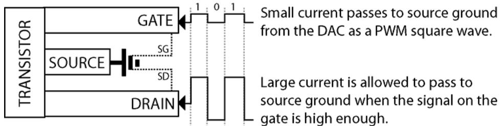
Figure 14 Modulating a high current with an audio signal using a FET.
