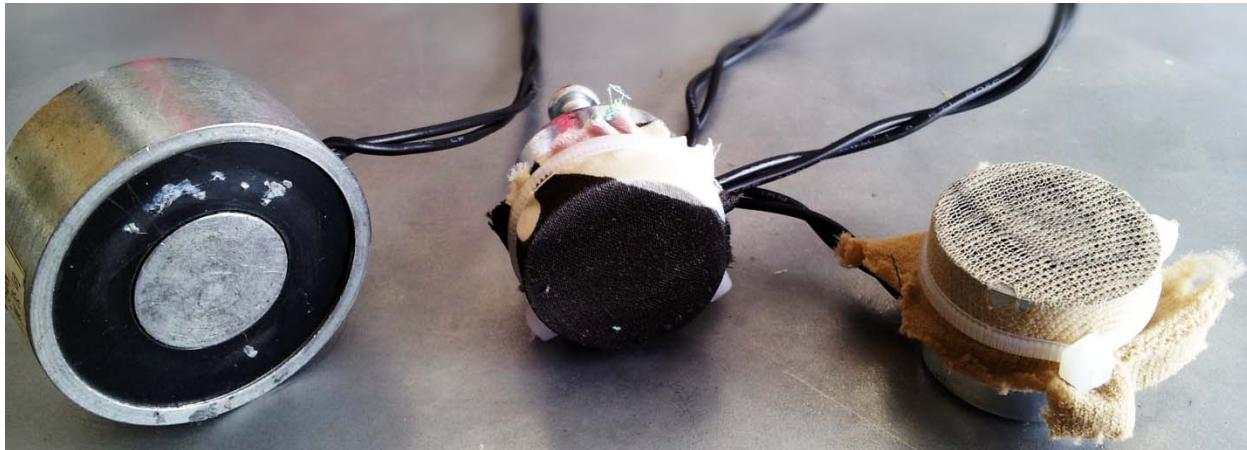
Figure 6 Large magnet (left) and two smaller magnets with fabric covering.
