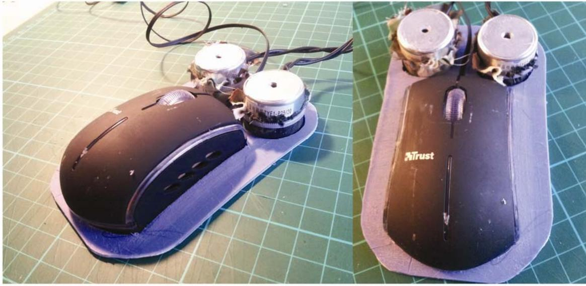
Figure 7 Prototype using a travel mouse and magnets
