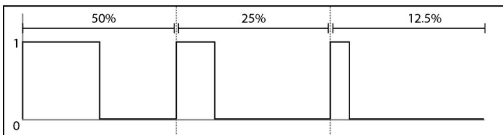
Figure 18 Pulse Waves with Pulse Widths of 50%, 25% and 12.5%
