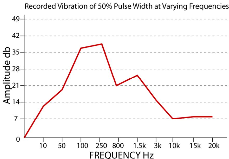
Figure 16 Recorded amplitude of acoustic vibration at varying frequency of control signal
