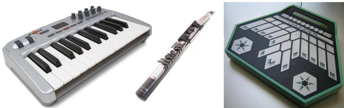
Figure 3 MIDI controllers. (Left to right) Portable keyboard with continuous encoders, breath controller and Buchla Thunder.
