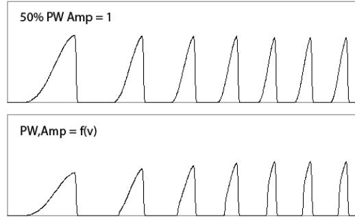
Figure 24 Mapping of  $v$  to PW and amplitude of the function
