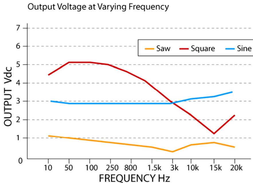
Figure 15 Output voltage with varying control signal frequency per waveform.
