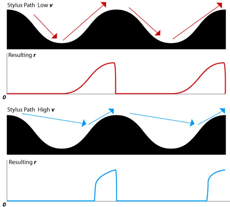
Figure 21 Graphic representation of how the path of the stylus changes with velocity and how this may be simulated with  $r$
