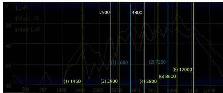
Figure 32 Annotated frequency response showing the harmonic content of the Guiro strike
