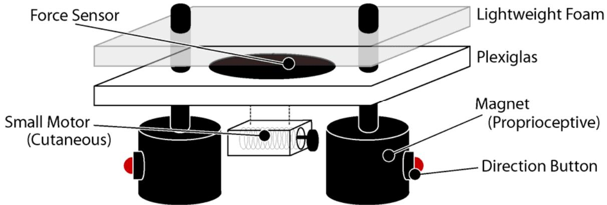
Figure 13 Sensor and actuator hardware design
