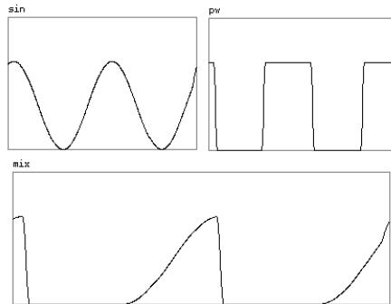
**Figure 22 Resultant multiplication of two simple waveforms to simulate the haptic response of a sinusoidal surface**
