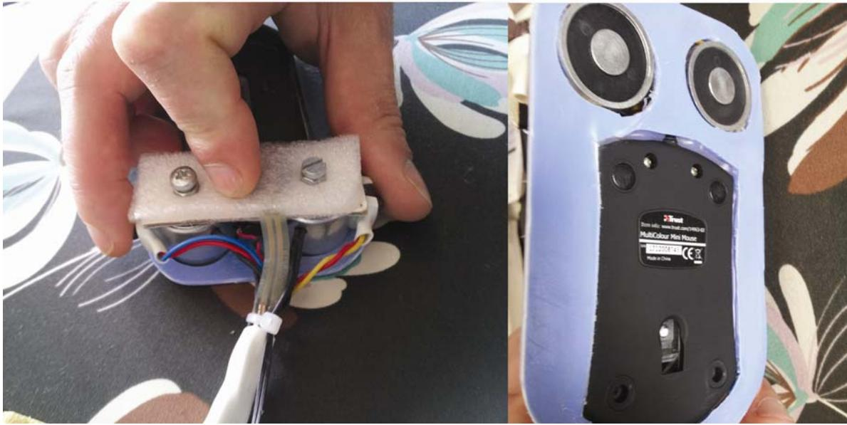
Figure 8. Prototype sensor assembly and magnet mounting
