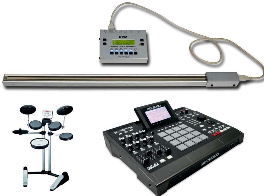
Figure 1 Music controllers. (Top) Ribbon controller, (left) Electronic Drums, (right) Akai MPC Drum pad and encoder unit.
