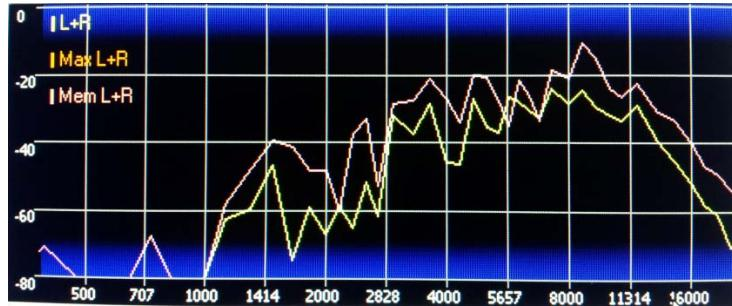
Figure 31 The frequency response of two isolated Guiro impacts during a stroke.
