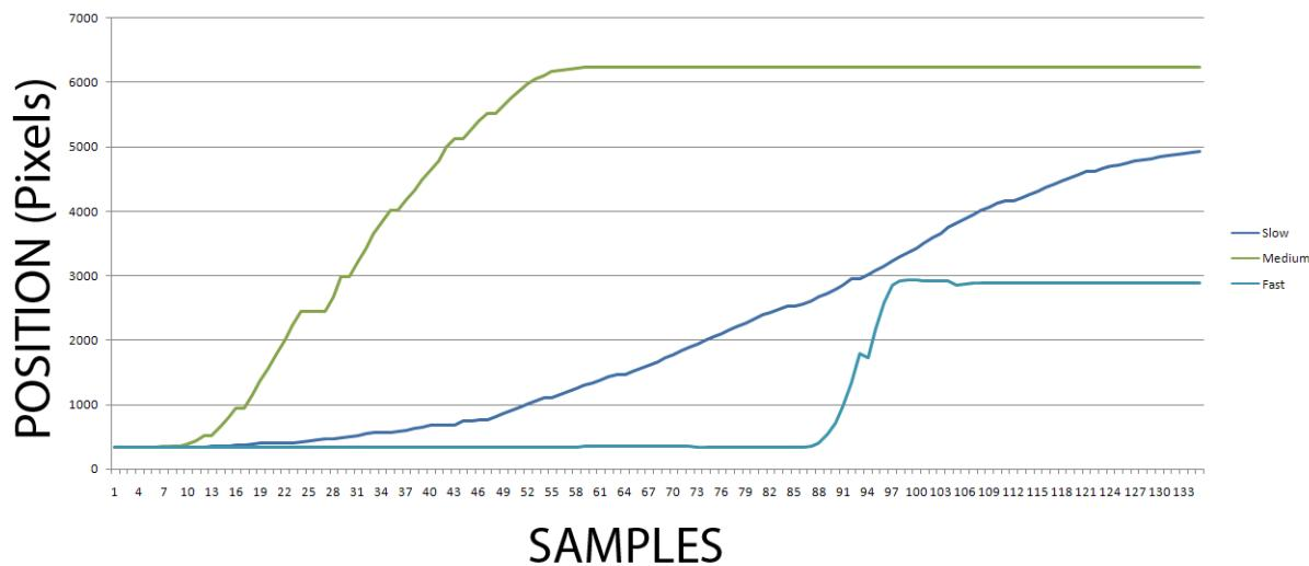
Figure 9 Graph of sampled mouse position for three stroking speeds over the same physical distance (20 cm).
