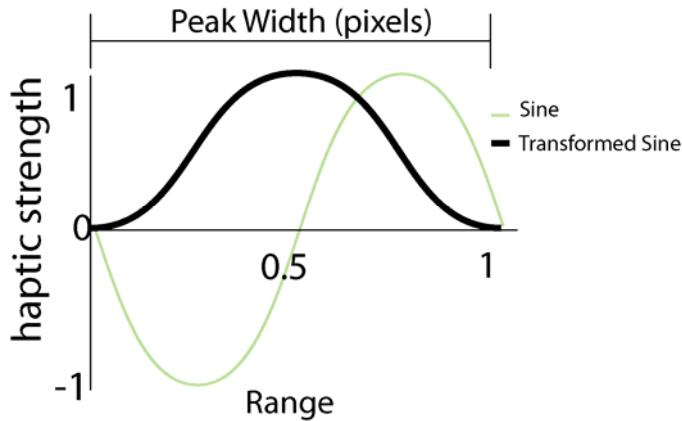
Figure 20 Transforming a sine wave for the Surface Function
