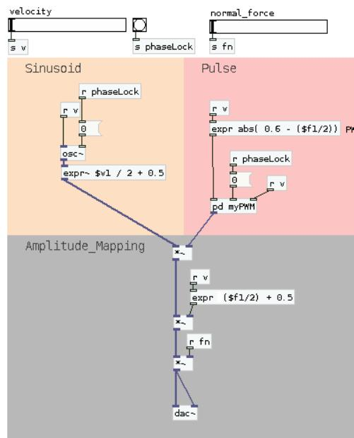
Figure 25 Pd implementation of the surface function
