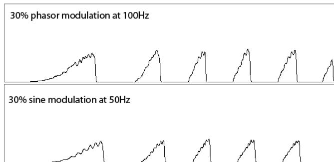
**Figure 26 Modulating the function with a higher frequency waveform to simulate roughness**
