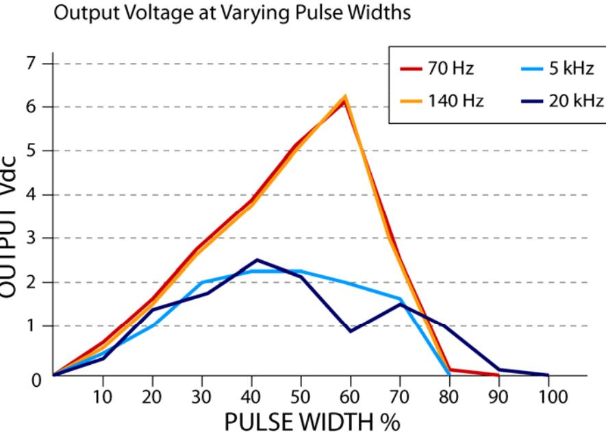
Figure 19 Output voltage at varying pulse widths
