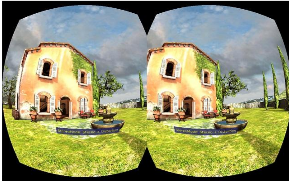
FIGURE 2: OUTPUT PICTURE OF THE OCULUS RIFT DISPLAY VIEWED WITHOUT LENSES. THE DISTORTION FITS THE VIEWING AREA WHEN SEEN THROUGH THE LENSES FITTED INTO THE DEVICE
