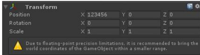
FIGURE 7: UNITY3D IS NOT ABLE TO HANDLE THE ASTRONOMICAL DISTANCES REQUIRED FOR A TRUE RELATIVE MODEL OF THE SOLAR SYSTEM WHEN IMPLEMENTING A STEREOSCOPING, EGO-CENTRIC SPACESHIP SIMULATION
