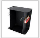
The three fluid pumps are screwed on the right side panel and the PCB's on the left side panel. Both screwed on from the inside.
