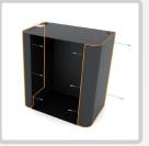
The side faceplates are screwed onto the back panel and the side panels.
