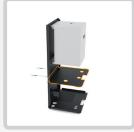
The middle plate is riveted onto the bottom sheet.
