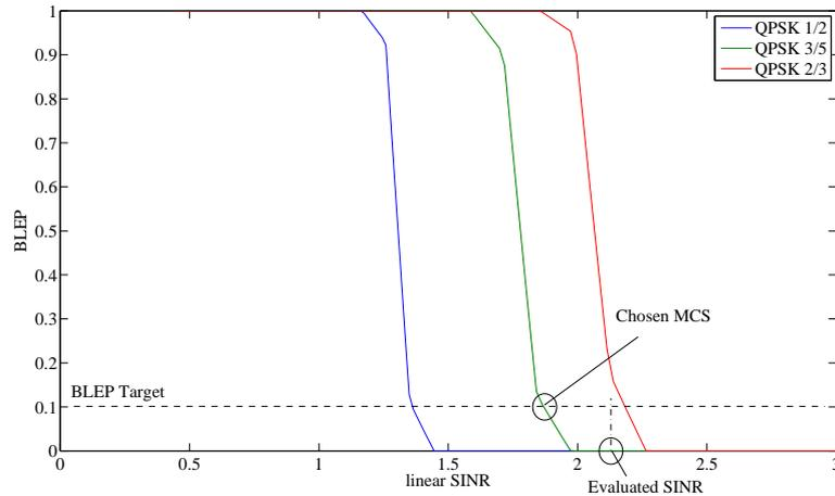
Figure 3.8: SINR versus BLER mapping function used to find the MCS that ensure BLER target
