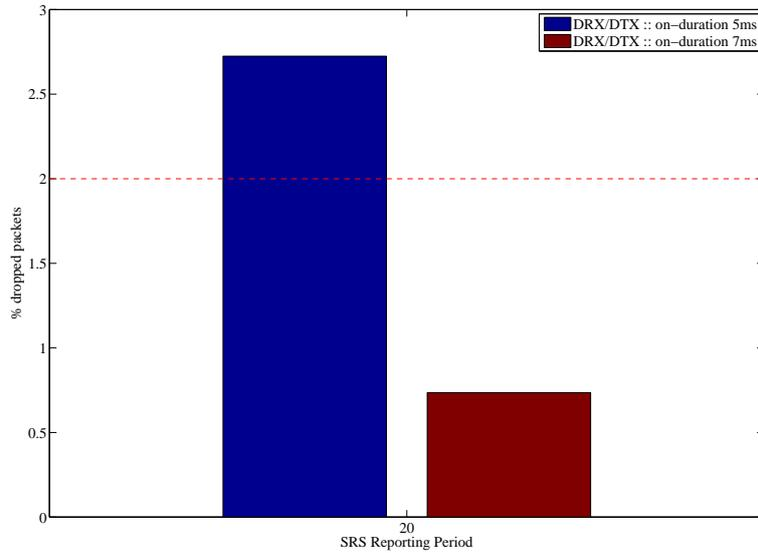
Figure 5.7: DS - Uplink packet drop probability, multiple users scenario (250 users at cell edge)
