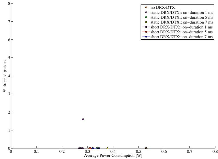
Figure 6.7: SPS - Average power consumption versus uplink packet drop probability, multiple users scenario (250 users)
