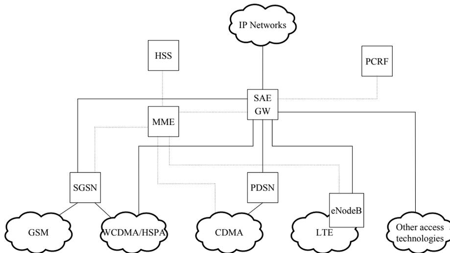
Figure 2.4: LTE and SAE combined architecture
