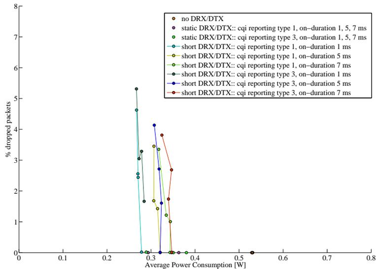
Figure 6.5: SPS - Average power consumption versus downlink packet drop probability, multiple users scenario (250 users)
