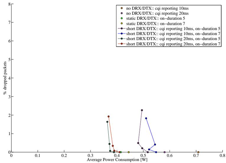
Figure 6.2: DS - Average power consumption versus downlink packet drop probability, single user scenario
