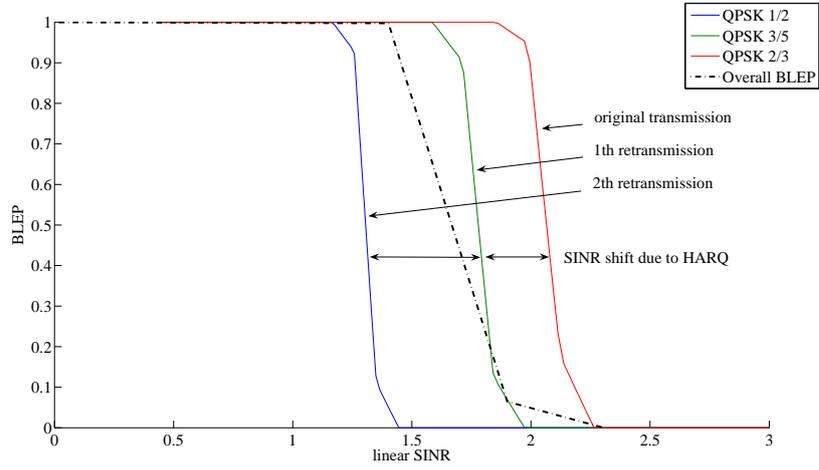
Figure 3.34: Overall BLEP after two retransmissions
