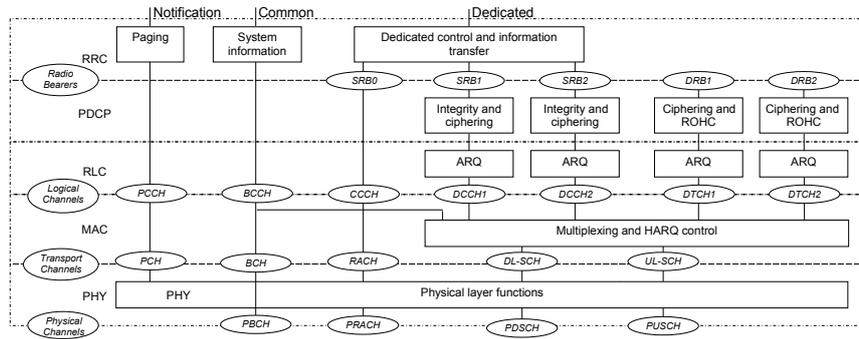
Figure 2.8: Radio Architecture for LTE. All channels denominations are defined in [6], [5] and [7]
