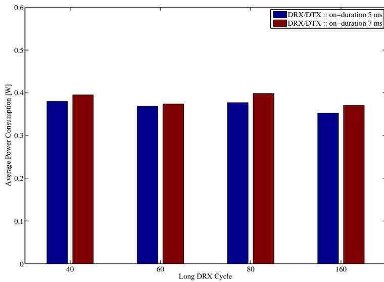
Figure 5.16: DS - Average power consumption, shortDRX, CQI/SRS periodicity 20ms, multiple users scenario (250 users at cell edge)
