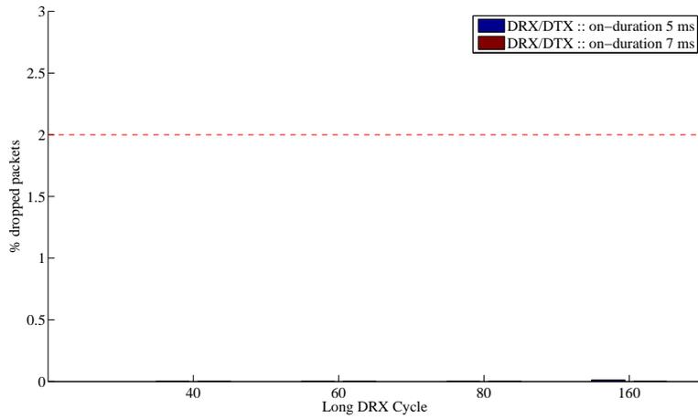
Figure 5.15: DS - Uplink packet drop probability, CQI/SRS periodicity 20ms, single user scenario
