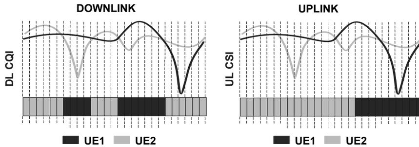
Figure 2.11: Frequency allocation comparison in DL and UL due to SC-FDMA constraints [13]
