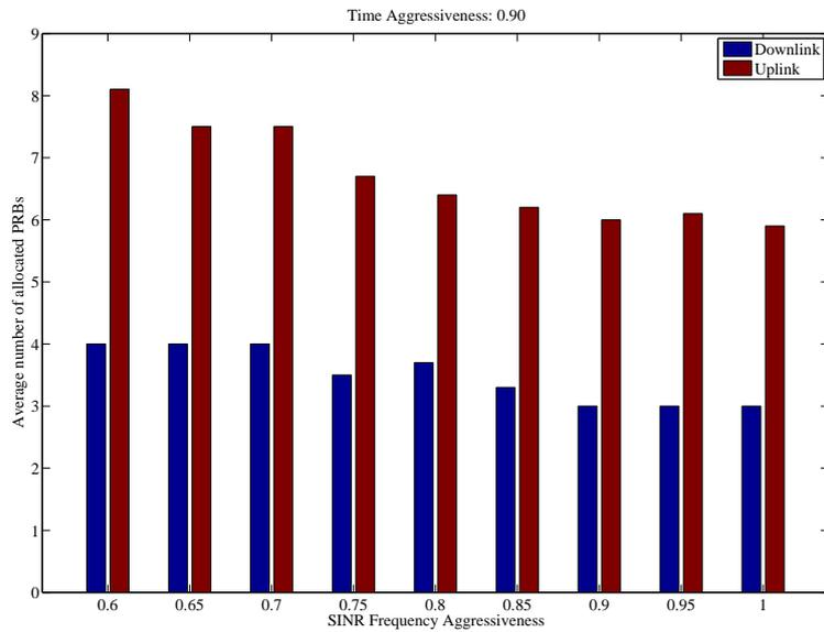
Figure 3.25: SPS - Average number of allocated PRBs in downlink and uplink transmission, Time Aggressiveness = 0.9
