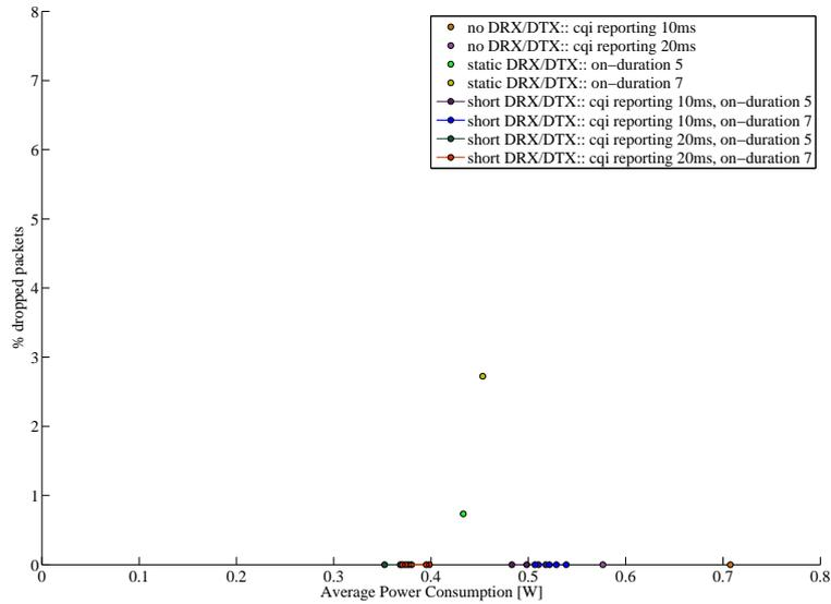
Figure 6.8: DS - Average power consumption versus uplink packet drop probability, multiple users scenario (250 users)
