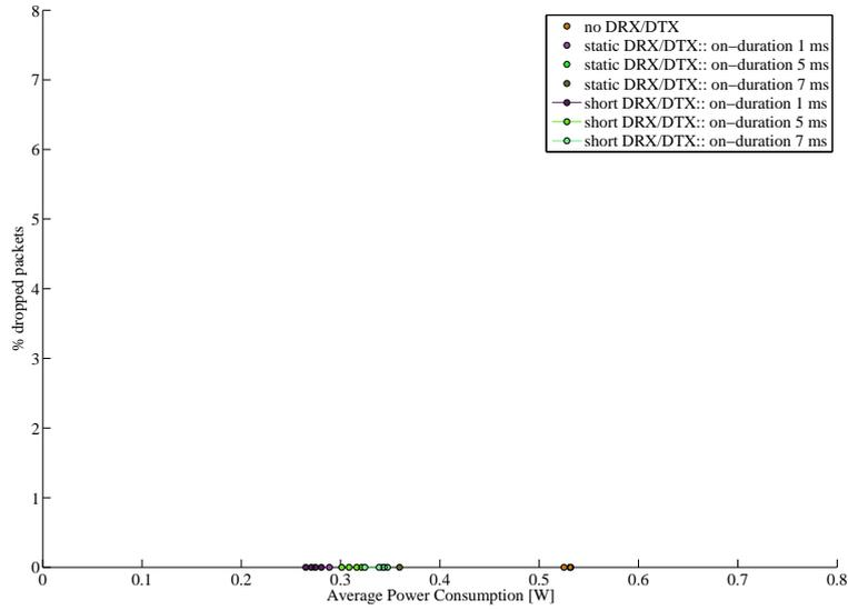
Figure 6.3: SPS - Average power consumption versus uplink packet drop probability, single user scenario
