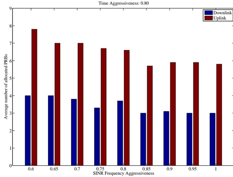
Figure 3.26: SPS - Average number of allocated PRBs in downlink and uplink transmission, Time Aggressiveness = 0.8
