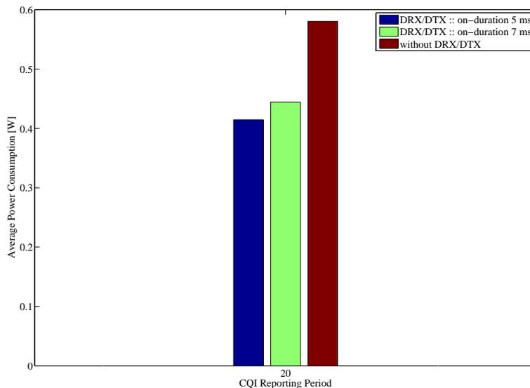
Figure 5.6: DS - Average power consumption, CQI/SRS periodicity 20ms, multiple users scenario (250 users at cell edge)
