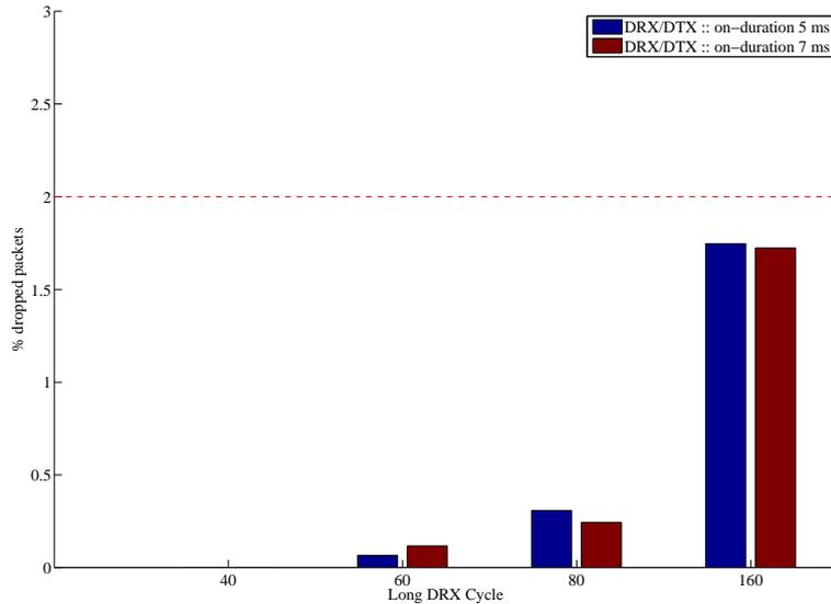
Figure 5.17: DS - Downlink packet drop probability, shortDRX, CQI/SRS periodicity 20ms, multiple users scenario (250 users at cell edge)
