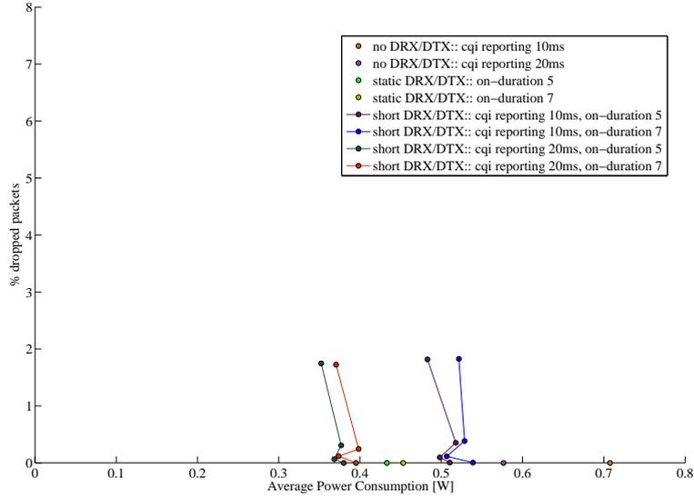
Figure 6.6: DS - Average power consumption versus downlink packet drop probability, multiple users scenario (250 users)
