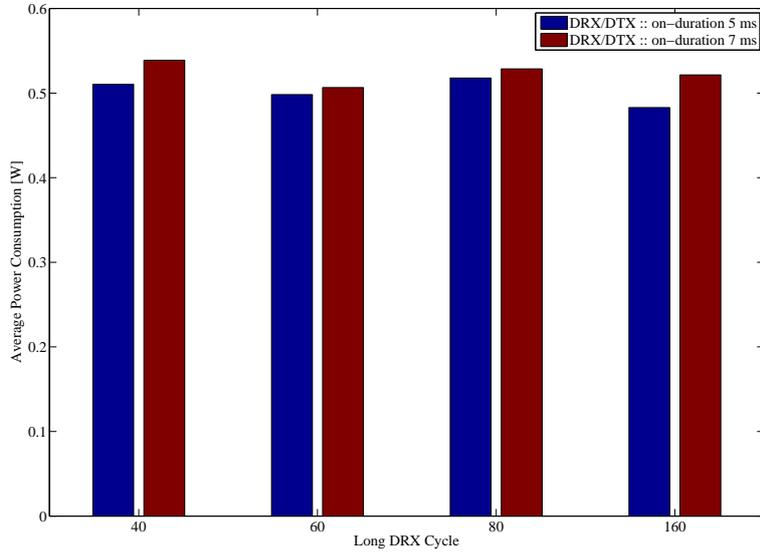
Figure 5.11: DS - Average power consumption, shortDRX, CQI/SRS periodicity 10ms, multiple users scenario (250 users at cell edge)
