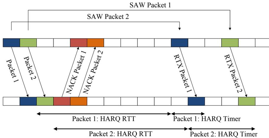
Figure 3.32: Downlink HARQ: the packet retransmission can be scheduled at least after 8 ms
