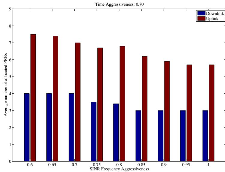
Figure 3.27: SPS - Average number of allocated PRBs in downlink and uplink transmission, Time Aggressiveness = 0.7
