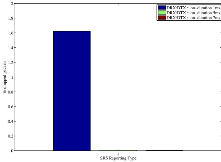
Figure 4.9: SPS - Uplink packet drop probability, multiple user scenario (250 users at cell edge)
