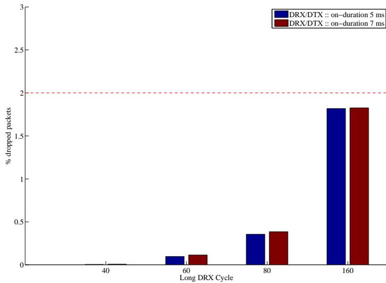
Figure 5.12: DS - Downlink packet drop probability, shortDRX, CQI/SRS periodicity 10ms, multiple users scenario (250 users at cell edge)
