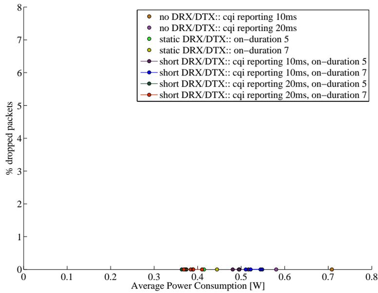
Figure 6.4: DS - Average power consumption versus uplink packet drop probability, single user scenario
