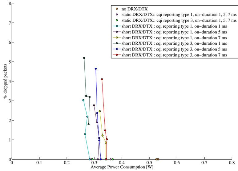
Figure 6.1: SPS - Average power consumption versus downlink packet drop probability, single user scenario
