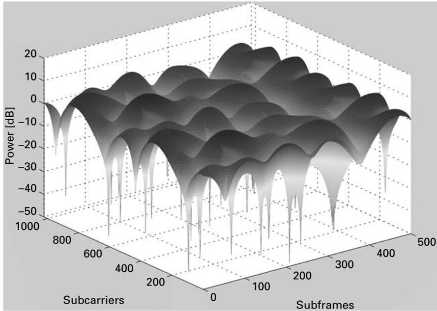
Figure 2.10: Signal power variation in time and frequency
