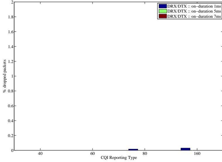
Figure 4.8: SPS - Downlink packet drop probability, multiple users scenario (250 users at cell edge)
