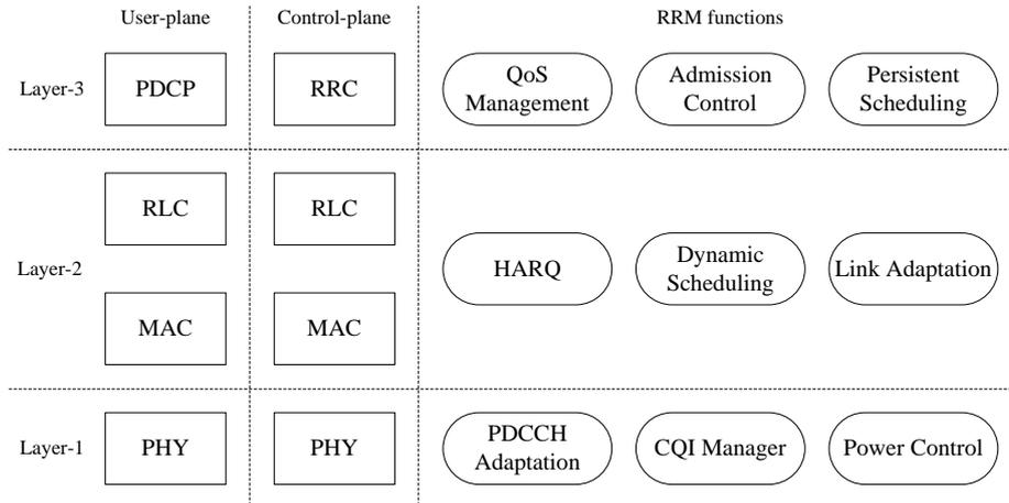
Figure 2.7: Overview of eNodeB user and control plane, with functionalities mapping over ISO/OSI layers
