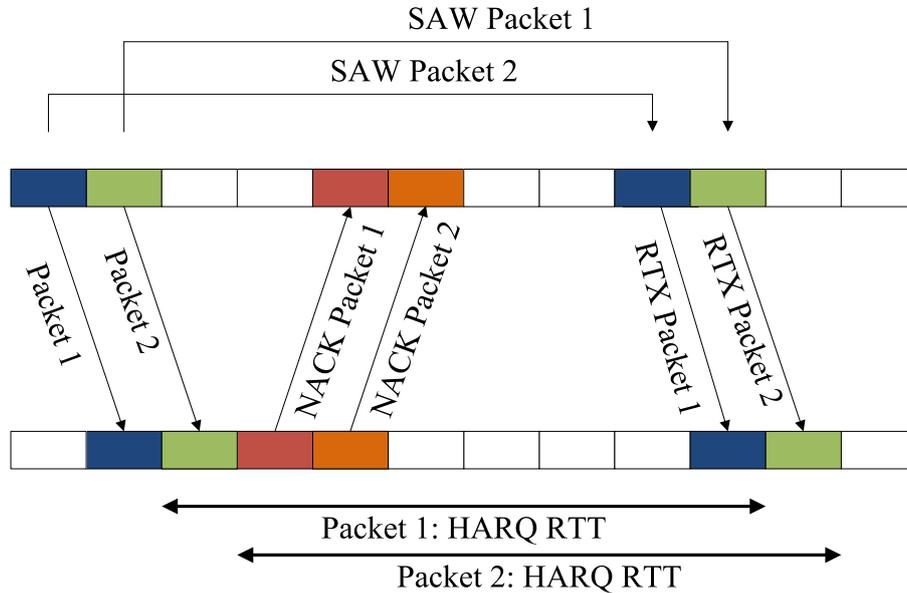
Figure 3.33: Uplink HARQ: the packet retransmission can be scheduled only after 8 ms
