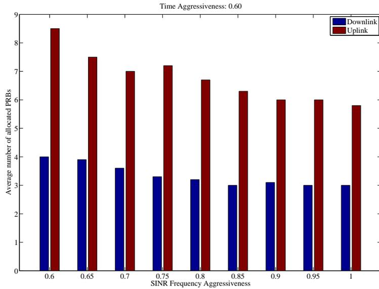
Figure 3.28: SPS - Average number of allocated PRBs in downlink and uplink transmission, Time Aggressiveness = 0.6
