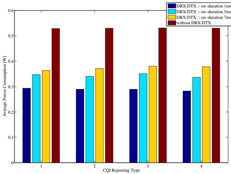
Figure 4.7: SPS - Average power consumption, multiple users scenario (250 users at cell edge)
