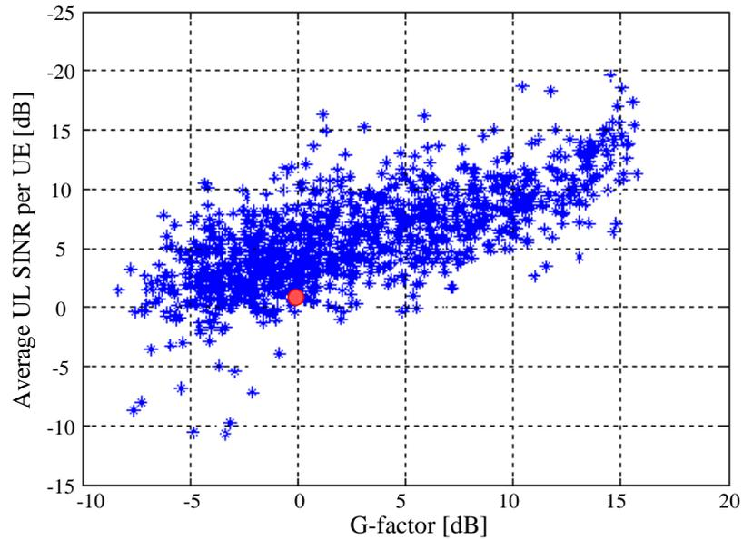
Figure 3.6: Downlink G-factor versus average UL SINR. Red point shows UE's working point
