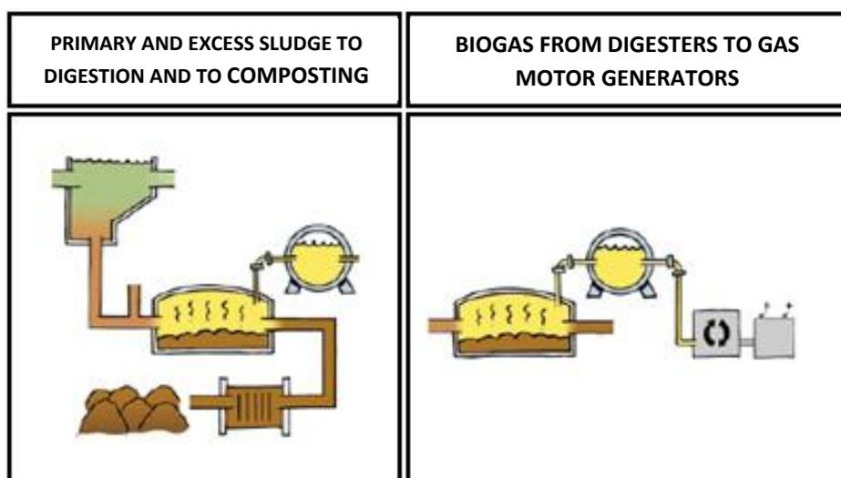
*Figure 7 Sludge management at Ejby Mølle WWTP*
