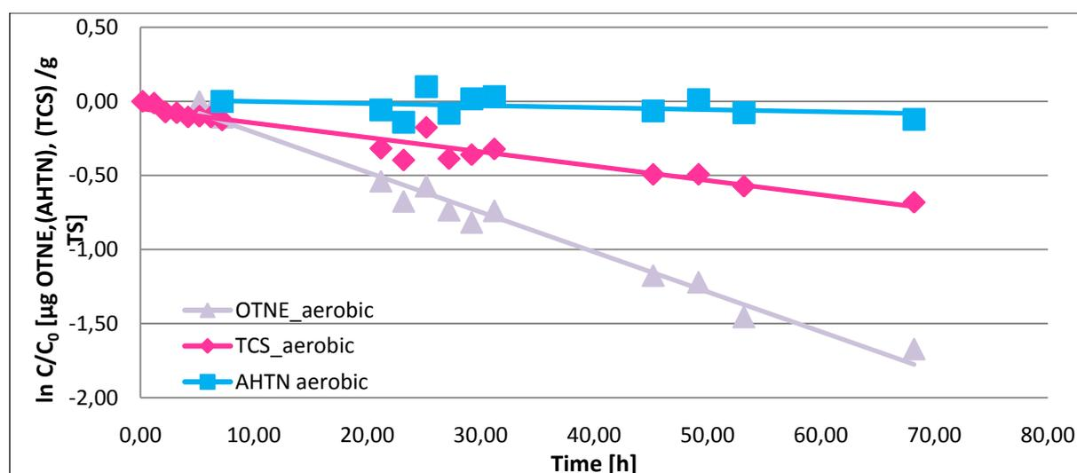
Figure 13 Comparison of AHTN, OTNE and triclosan  $\ln C/C_0$  during the first aeration experiment (Electron acceptor regimes I) in the activated sludge
