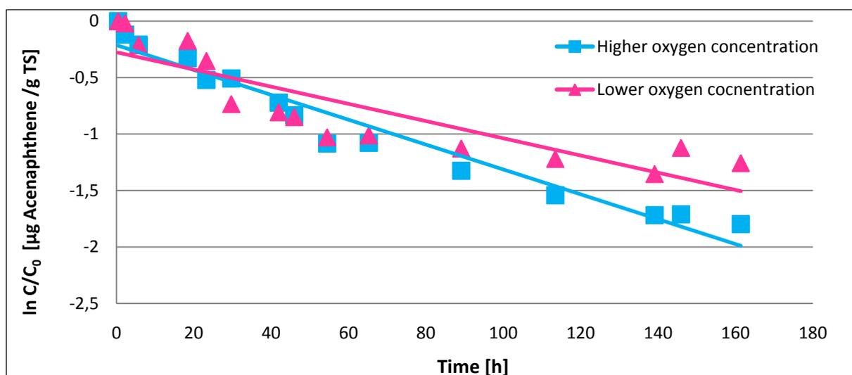
Figure 21 Comparison of acenaphthene  $\ln C/C_0$  during incubation with lower and higher oxygen concentration in the sixth degradation experiment (Oxygen concentration I)
