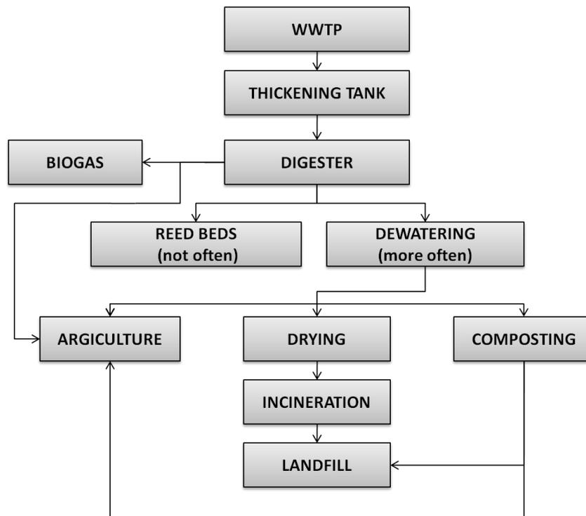
Figure 3 Process flowcharts of the sludge processing steps after digestion
