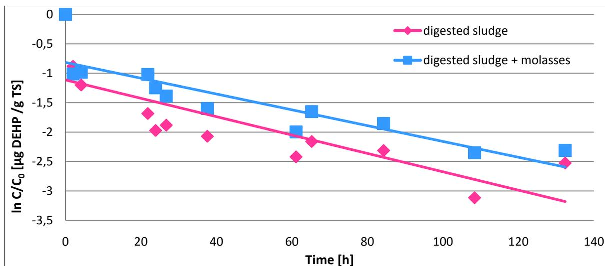
Figure 17 Comparison of DEHP  $\ln C/C_0$  in two reactors: I) digested sludge and II) digested sludge + molasses
