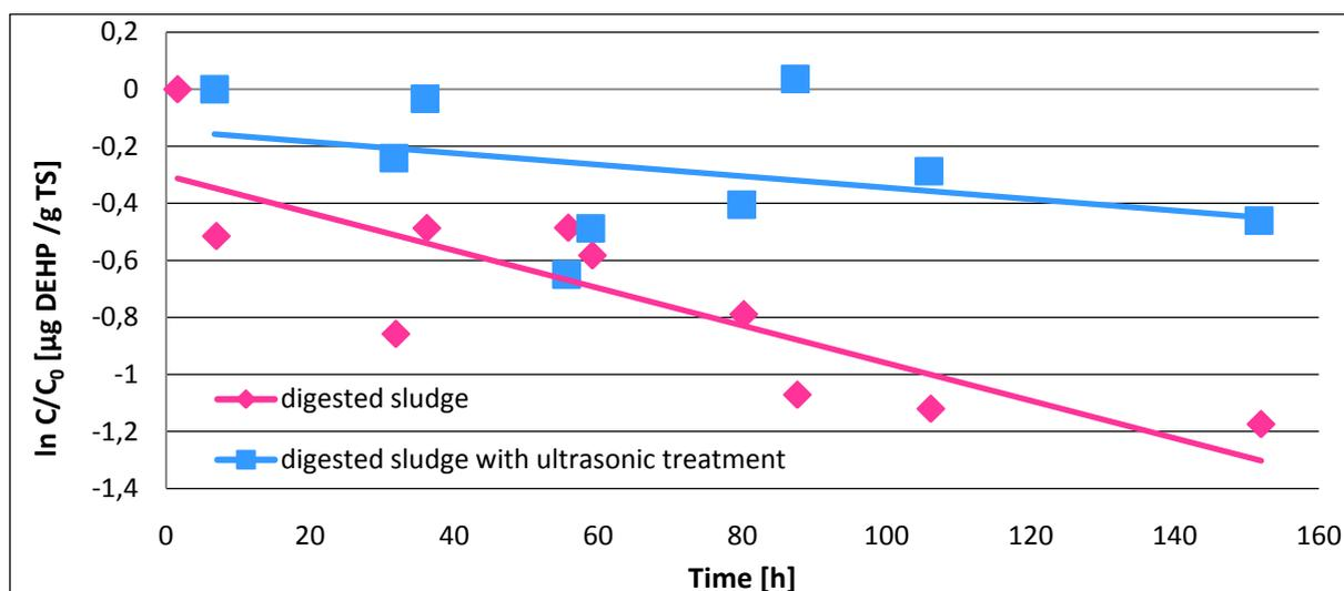
*Figure 18 Influence of the ultrasound treatment on the processes in the digested sludge;  $\ln C/C_0$  of DEHP versus time [h]*
