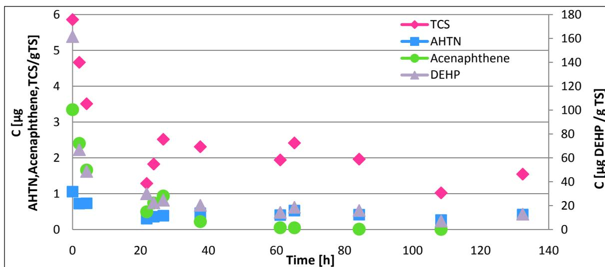
Figure 14 Comparison of AHTN, DEHP, triclosan and acenaphthene removal in the reactor I from the fifth degradation experiment (Ultrasound)
