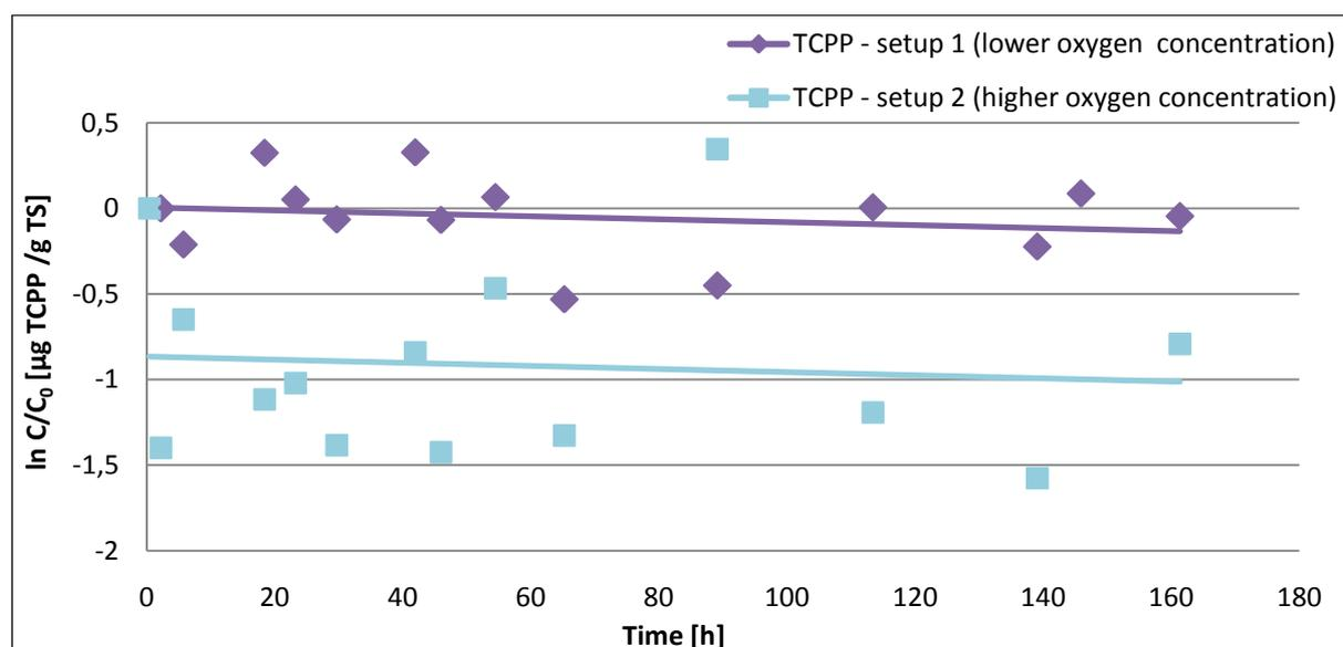
Figure 20 Ln C/C<sub>0</sub> of TCPP in the sixth degradation experiment (Oxygen concentration I) in two setups: 1) higher oxygen C, 2) lower oxygen C
