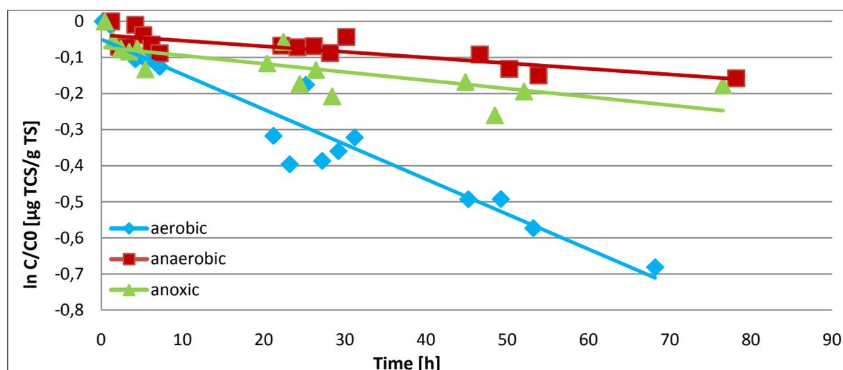
Figure 11  $\ln C/C_0$  of triclosan under aerobic, anaerobic and anoxic conditions during first aeration experiment (Electron acceptor regimes I) in the activated sludge (triclosan was spiked to the experiment)
