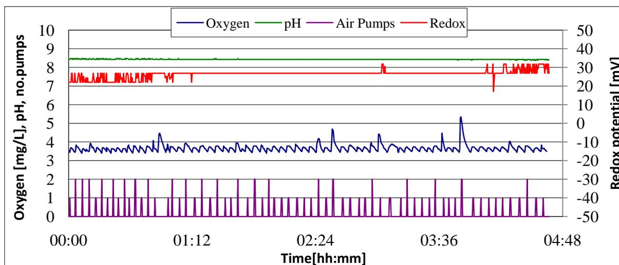
*Figure 22* Constant measurement of oxygen, pH, redox potential and number of pumps running within a short period of the sixth experiment (oxygen concentration I).
