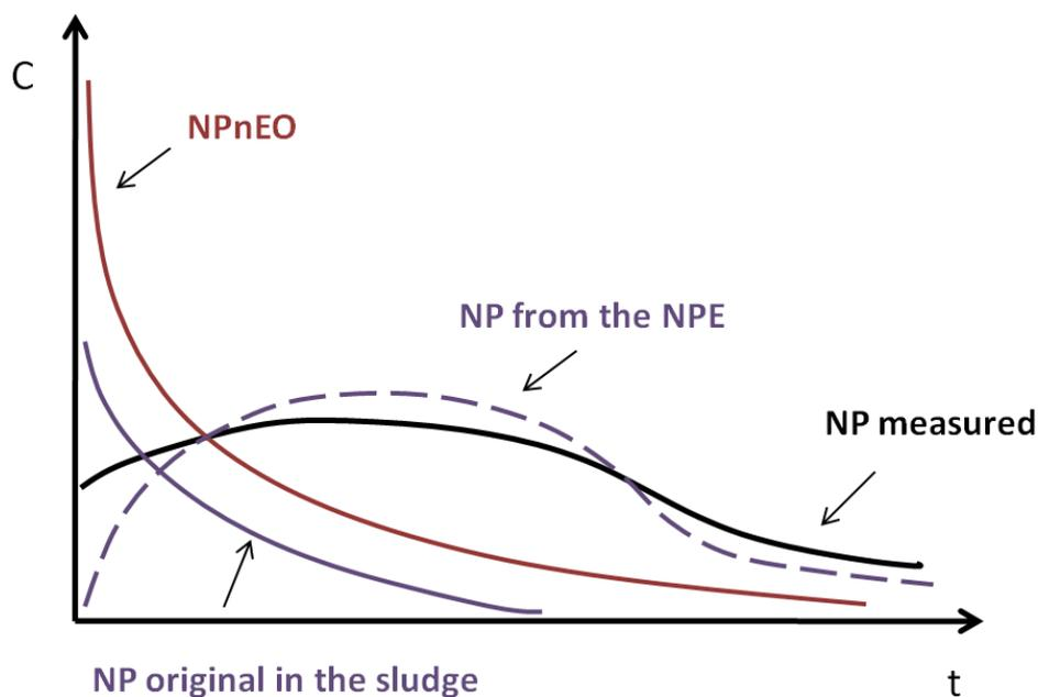
Figure 24 Expected concentration of nonylphenol (NP) and nonylphenol polyethoxylates (NPE) in the sludge under the aerobic conditions in the sludge
