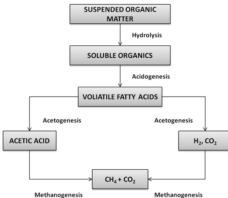
Figure 2 Subsequent steps in the anaerobic digestion process [10]
