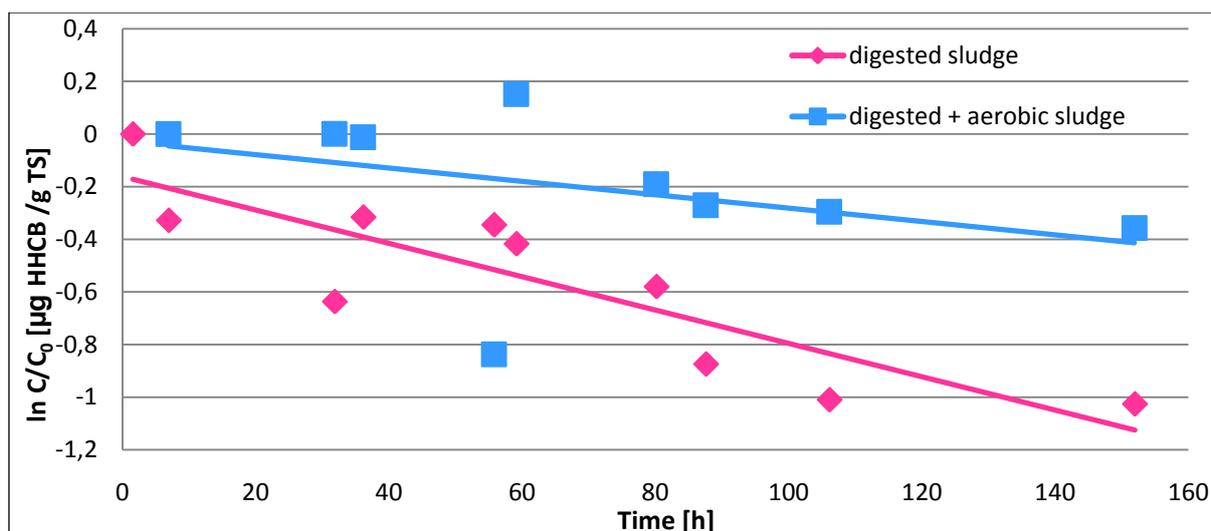
Figure 16 Comparison of  $\ln C/C_0$  of HHCB in to reactors: I) digested sludge, and II) digested sludge +sludge from aeration tank
