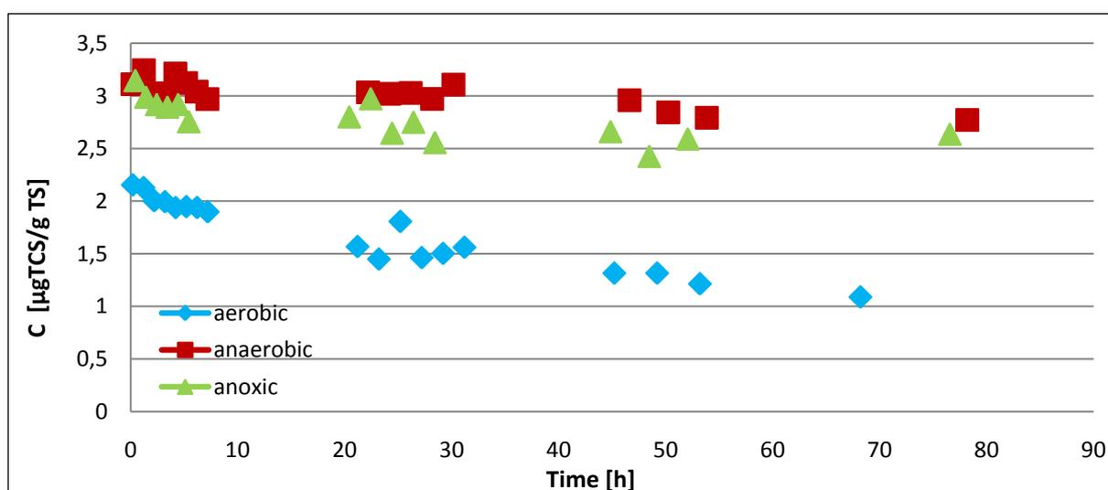
*Figure 10* Concentration of triclosan under aerobic, anaerobic and anoxic conditions during first aeration experiment (Electron acceptor regimes I) in the activated sludge (triclosan was spiked to the experiment). TSC = triclosan, TS = total solid
