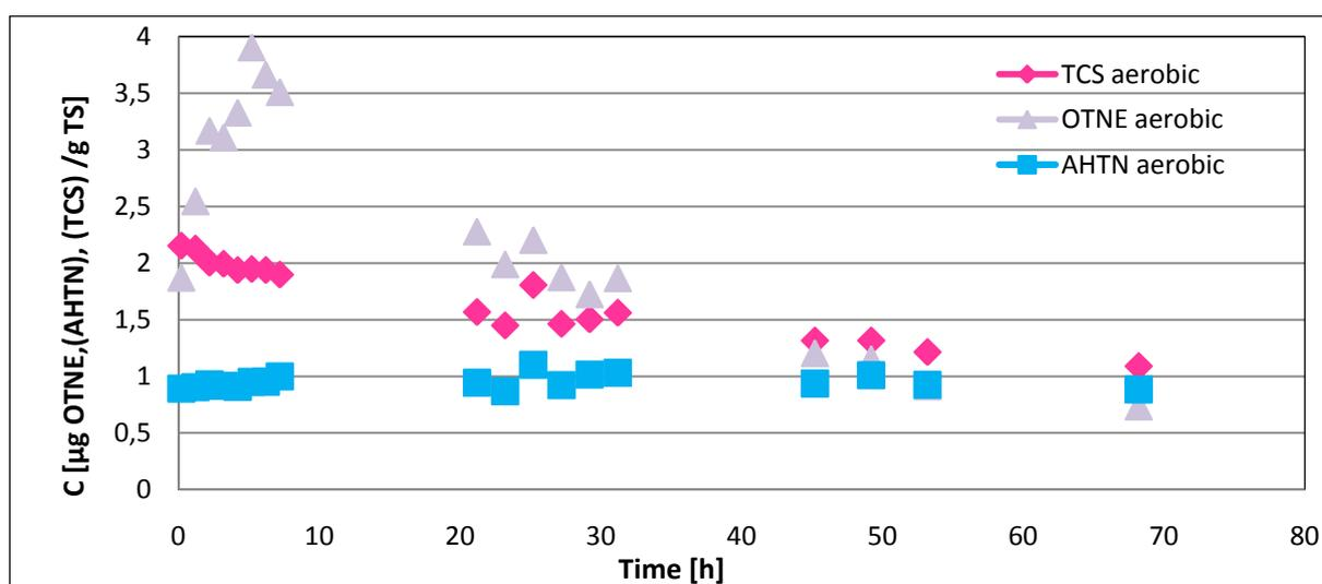
Figure 12 Comparison of AHTN, OTNE and triclosan during first aeration experiment (Electron acceptor regimes I) in the activated sludge
