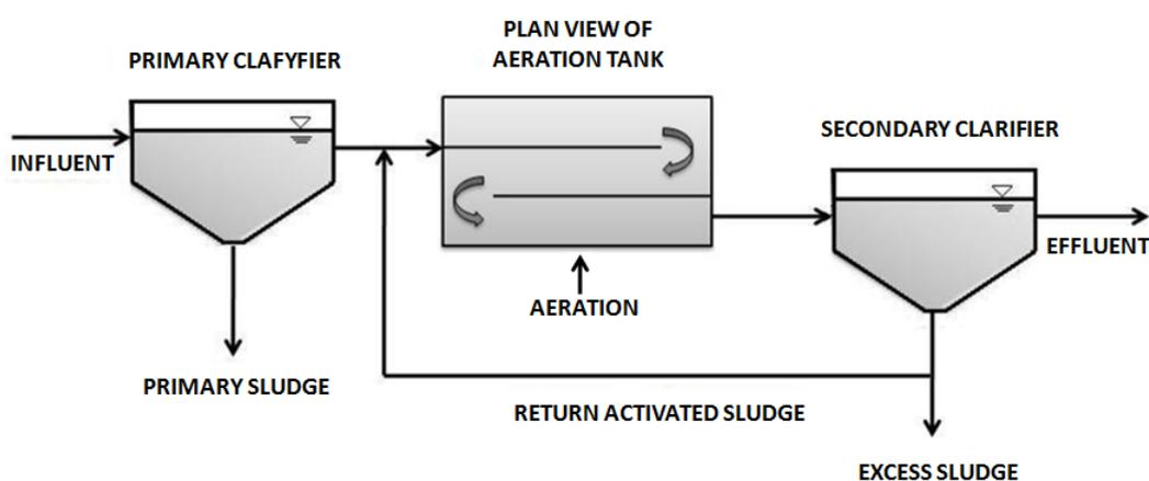
*Figure 1 Simplified activated - sludge treatment with plug-flow reactor*
