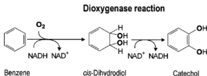
Figure 4 Initial attack on xenobiotics by oxygenases (redrawn from [78]). Dioxygenases incorporate both atoms into the substrate
