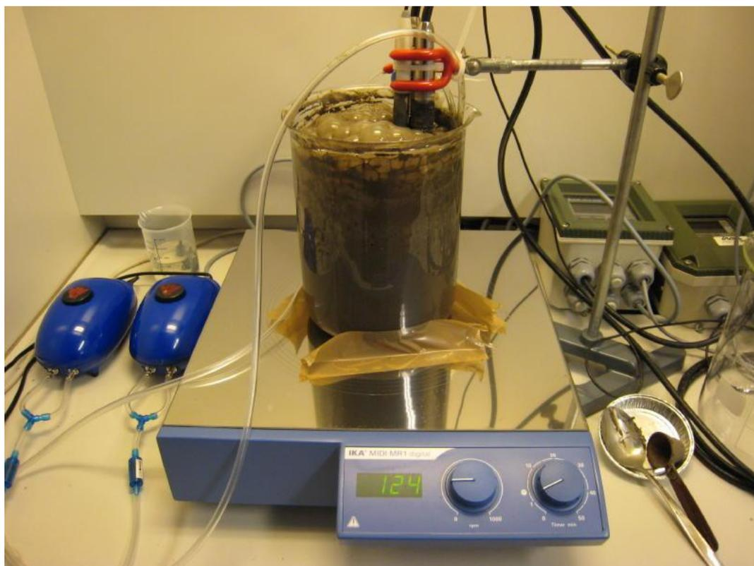
*Figure 8* Picture of the reactor with digested sludge during the experiment performed at Ejby Mølle WWTP
