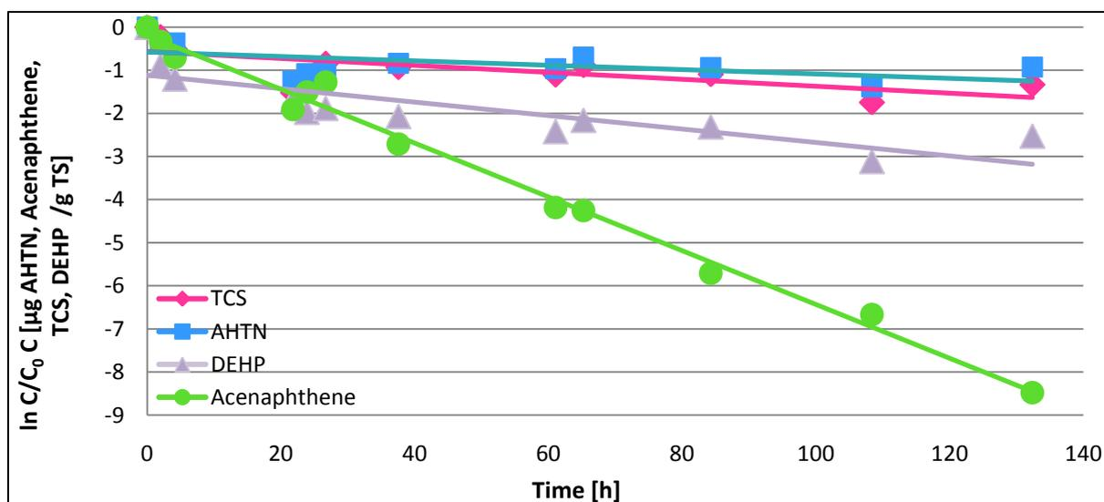
Figure 15 Comparison of  $\ln C/C_0$  of AHTN, DEHP, triclosan and acenaphthene removal in the reactor I from the fifth degradation experiment (Ultrasound)
