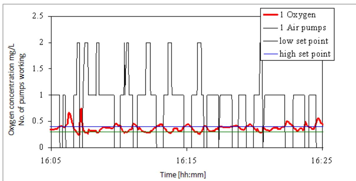
Figure 9 Oxygen control in set up 1
