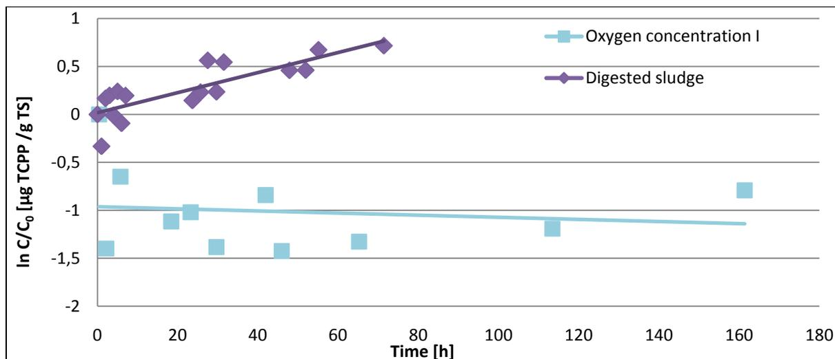
Figure 19 Comparison of TCPP  $\ln C/C_0$  in the third and fifth degradation experiment (Triclosan and Molasses), without and with correction of water evaporation, respectively.
