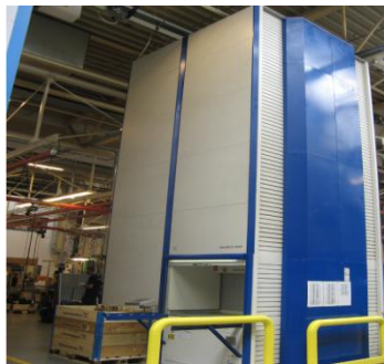
Picture 9: Kardex tower/inventory system
