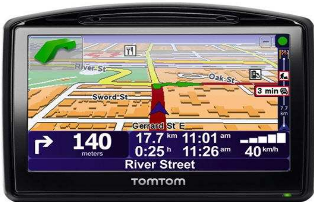
Picture 1. Example of the GPS in 'driving view'. The map is illustrated in 3D. In the map are street names, POI icons and zoom options. Navigation and system information are shown on the lower part of the screen.
