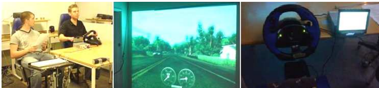
Figure 2. Pictures of the driving simulator. Left: the test manager sitting in the passenger seat next to the participant. Middle: A view of the road in the simulator (bottom part of the view included the speedometer). Right: The steering wheel and music player
