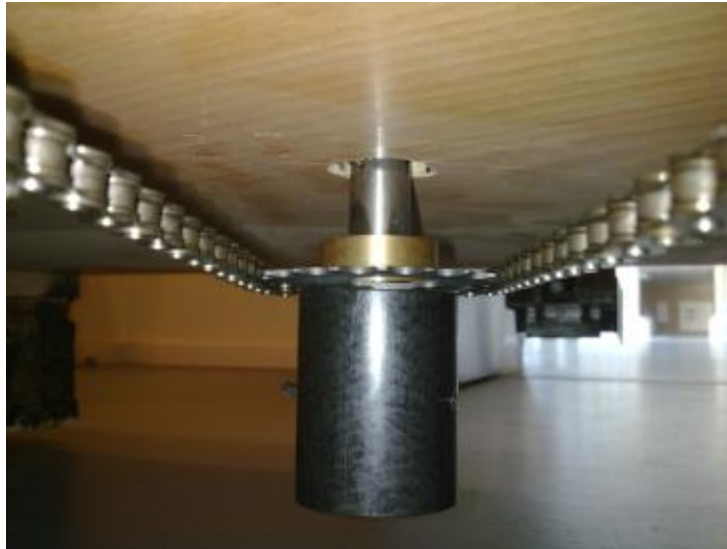
Figure 21 Picture of the implementation of the chain connection between the two platforms, allowing duplication of rotation.
