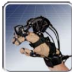
Figure 7 The CyberGrasp™ Exoskeleton allows the user to grab a object in a 3D virtual world and feel the size and shape of the object, this is an addition to the CyberGlove system.
