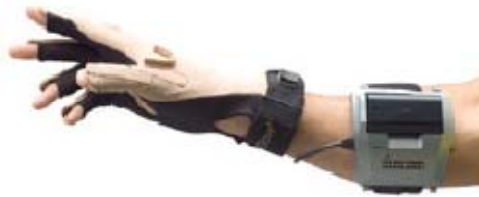
Figure 6 The CyberGlove® II System, allowing a user to use his or hers hands inside e.g. a virtual environment.
