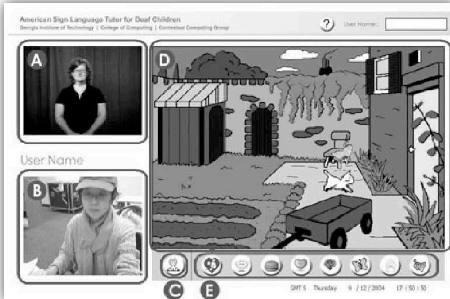
Figure 7 A screen shot of the interface, A) is the tutor video, B) The real life camera feed C) Attention button, D) The animated environment, E) Action button
