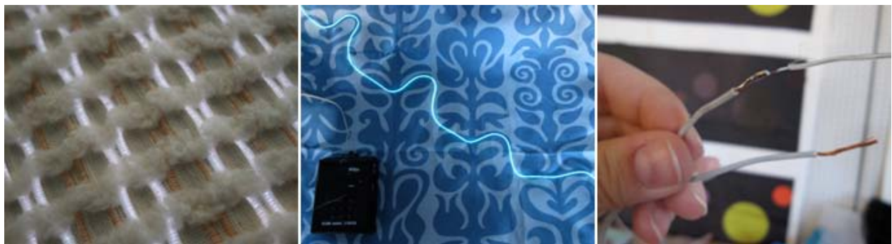
Figure 23 - Inspiration picture (left); EL wire connected to an inverter (middle); Soldering of EL wire with a connecting wire from the inverter (right)
