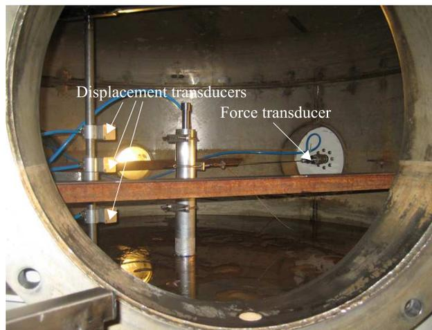
**Figure A.11:** The employed displacement transducers and force transducer.
