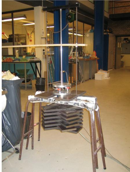
**Figure B.6:** Setup for CPT-calibration.
