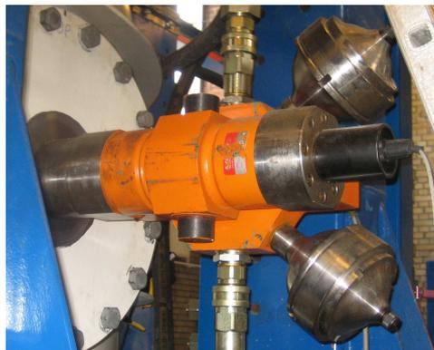
Figure A.4: Hydraulic piston employed to actuate the test piles.
