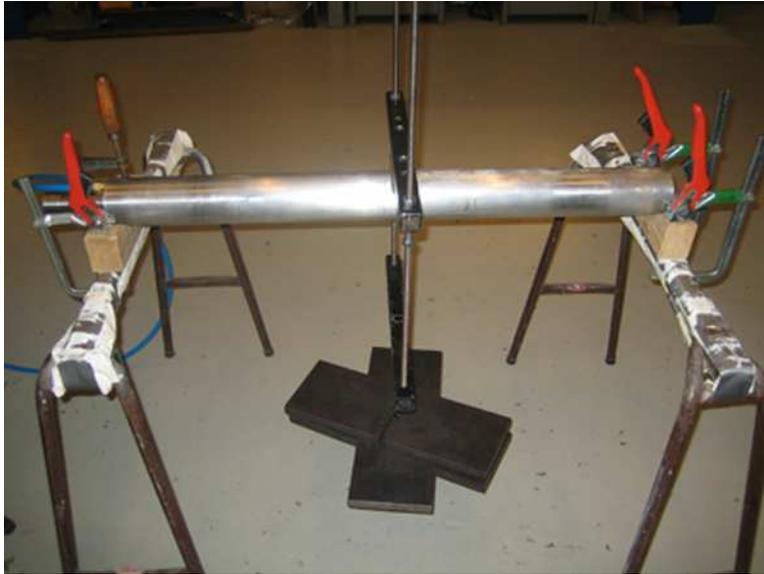
Figure A.17: Test setup for calibration of pile bending stiffness,  $E_p I_p$ .
