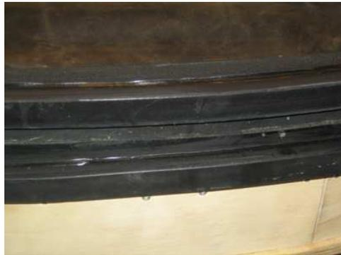
(a) Mouldings mounted on the outside of the membrane.
